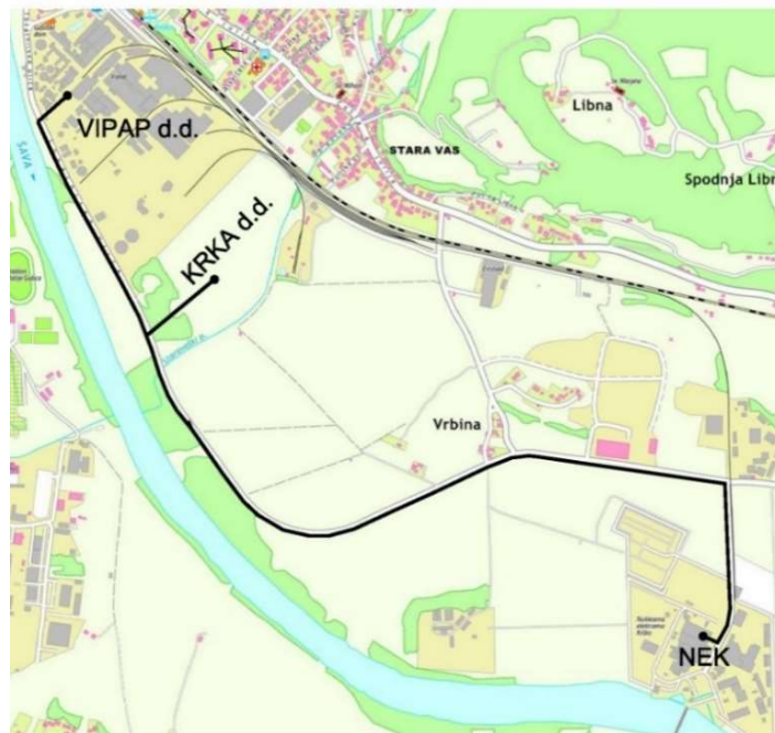
FIG. 6. A schematic display of the foreseen steam distribution system for industrial consumers Vipap and Krka [2].
