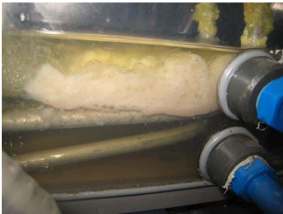
FIG. 15. Crud formation due to suspended solids (Courtesy of Hydromet Pty Ltd).
