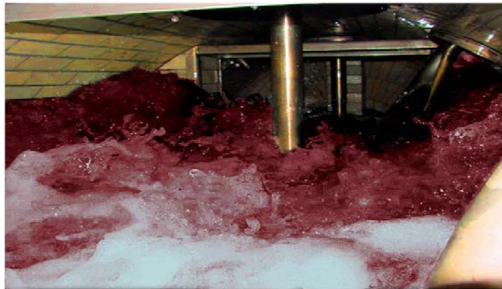
FIG. 5. View inside a pressure leach autoclave (courtesy Hydromet Pty Ltd).
