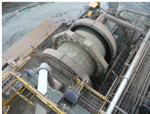
FIG. 19. Example of comminution equipment (SAG Mill, courtesy of Orway Mineral Consultants Pty. Ltd.).
