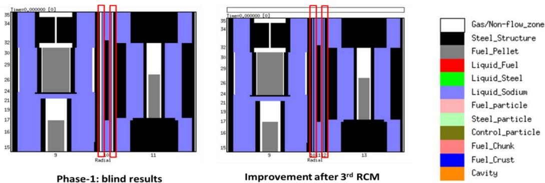
FIG. 98. SHRT-17: Improvement on the XX10 model after 3rd RCM: "explicit" modelling of inter-wrapper sodium.
