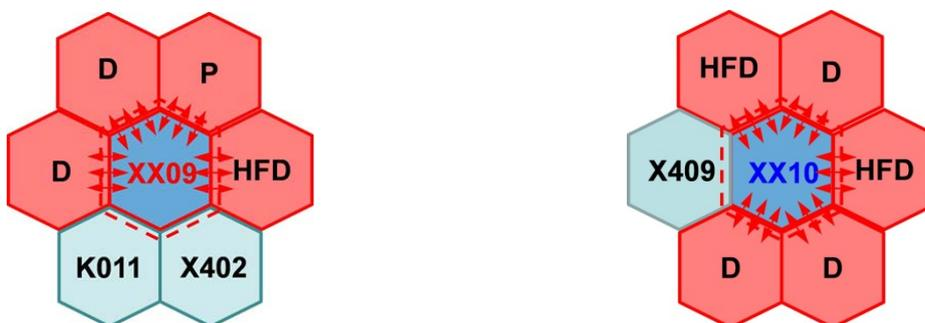
FIG. 296. The XX09 and XX10 instrumented subassemblies and their neighbouring subassemblies during SHRT-17.
