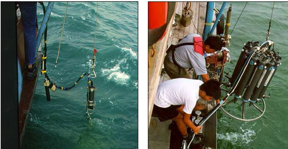
FIG. 13. Deployment of scintillation counters for in-situ measurement of  $^{198}\text{Au}$  and sampler for tritium analysis.
