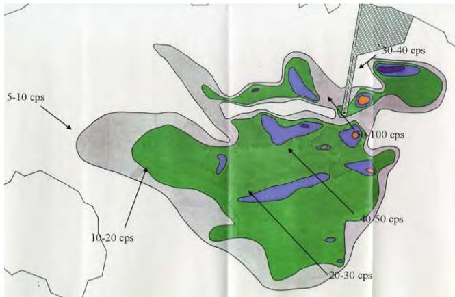
FIG. 4. Map of the tracer deposit on the sea bed 33 days after the beginning of the injection i.e. 2 days before its end (det 2).
