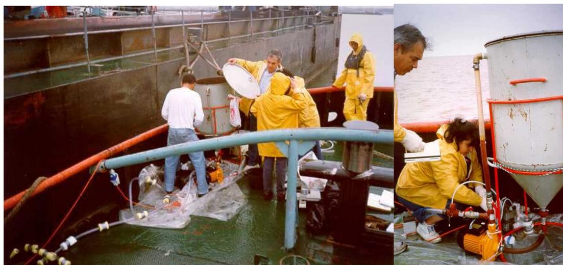
FIG. 9. Labelling and injection system used in Brazil and some countries in Latin America.
