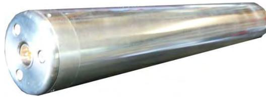
*FIG. 15. Example of a waterproof NaI(Tl)  $\phi$  38  $\times$  50 mm detector, waterproof 80 m water depth, aluminium or stainless steel housing.*
