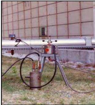
FIG. 6. A conventional injection device for chemical industry applications.
