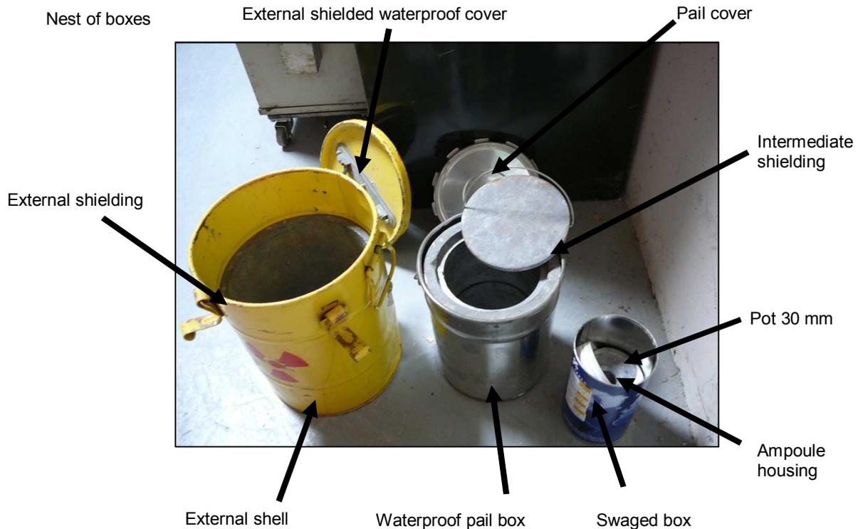
FIG. 3. Example of a transportation container.
