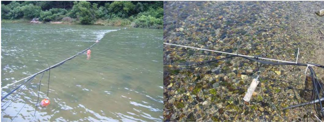
*FIG. 10. Installation of NaI scintillation detectors for the radiotracer experiment in a river.*
