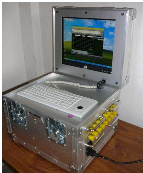
*FIG. 16. Multi probes (15) data acquisition system.*
