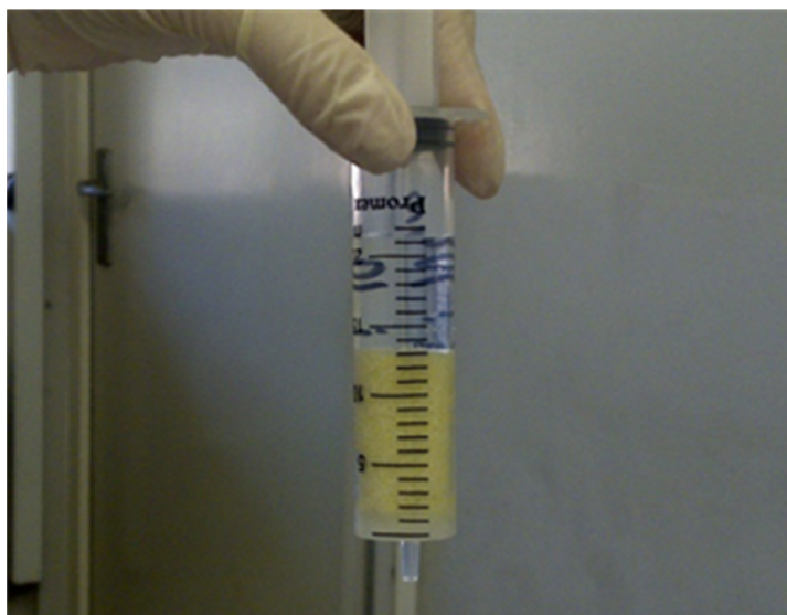
FIG. 9. Leaching studies of Cs-137 contaminated oil encapsulated into Nochar.
