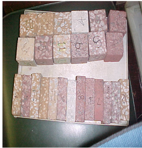
FIG. 3. Manufacturing of concrete cubes (cured for 28 days under water) for compression and tensile testing.
