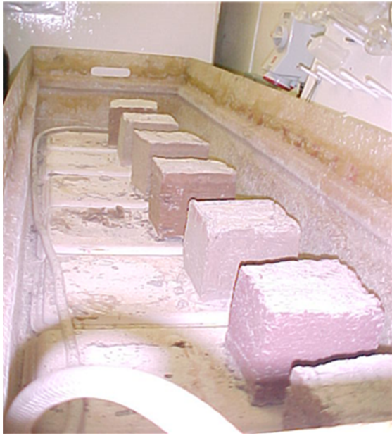
FIG. 3. Manufacturing of concrete cubes (cured for 28 days under water) for compression and tensile testing.
