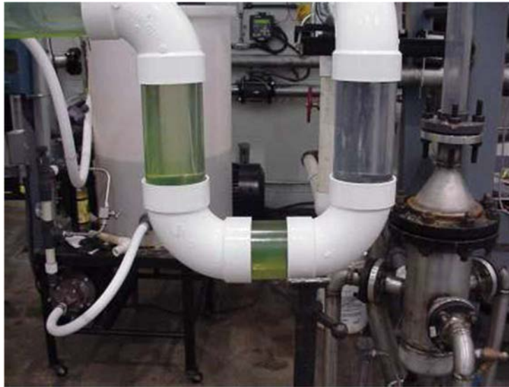
FIG. 27. Injected coolant mixing with fluid in a transparent loop seal [20].
