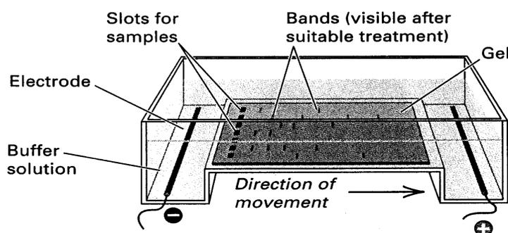
Figure 4.3. Apparatus for gel electrophoresis (Hartl and Jones, 1999).
