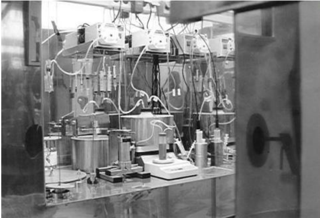
Inner layout of Hot cell of ^{99m}\text{Tc} Generator lab
