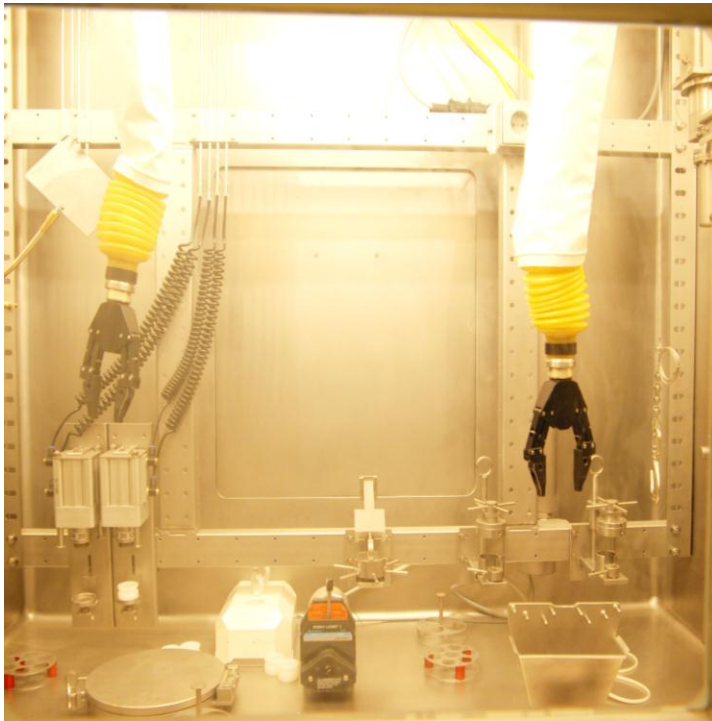
In-cell equipment of Hot cell-3
