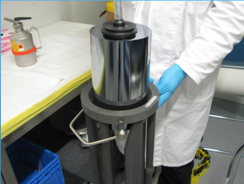
Insertion of Si ingots into the loading basket
