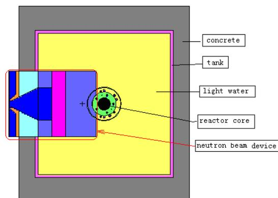
Fig. 7. The core configuration of MNSR-I.
