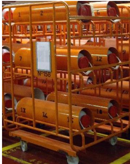
FIG. 2. Tubular carriage for the transfer of drums.
