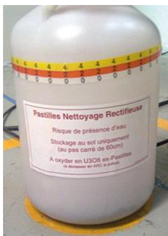
FIG. 1. Specific label for a 10-liters drum with wet fissile material.
