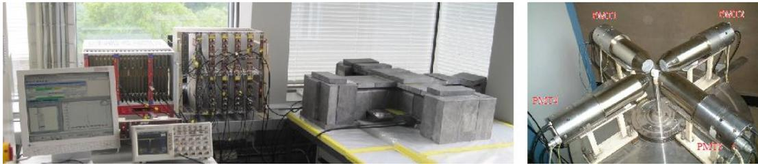
FIG.5. Four LaBr<sub>3</sub> detector positron lifetime spectrometer with & without Pb shielding.
