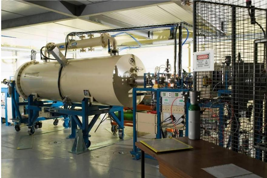
*FIG. 3. Picture of the third ion accelerator, JAPET (2 MV tandem) installed in the Jannus-Saclay facility in Nov. 2009.*
