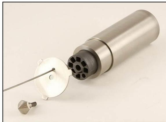
FIG. 9. An High Temperature irradiation capsule.
