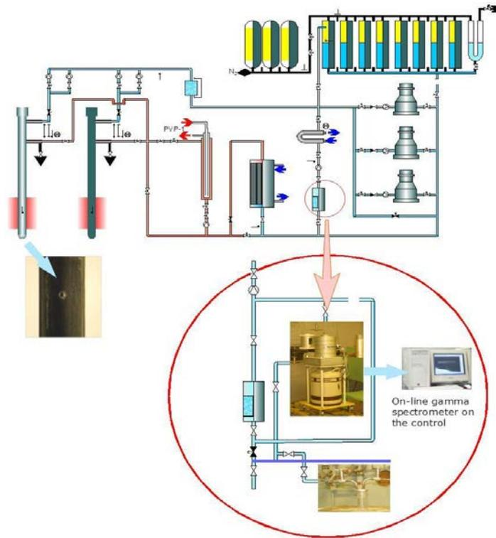
FIG. 12. Technique for investigation of fission products release in the coolant of leaking fuel rods at different burn-up.
