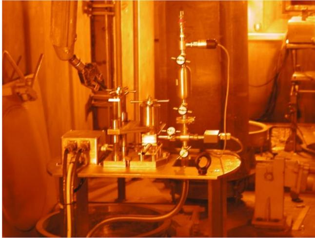
FIG. 27. Installation for punching of fuel element and measurement of released fission gas.
