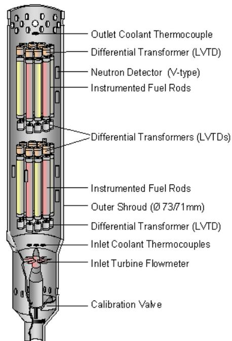
FIG. 5. Irradiation of instrumented fuel rods.
