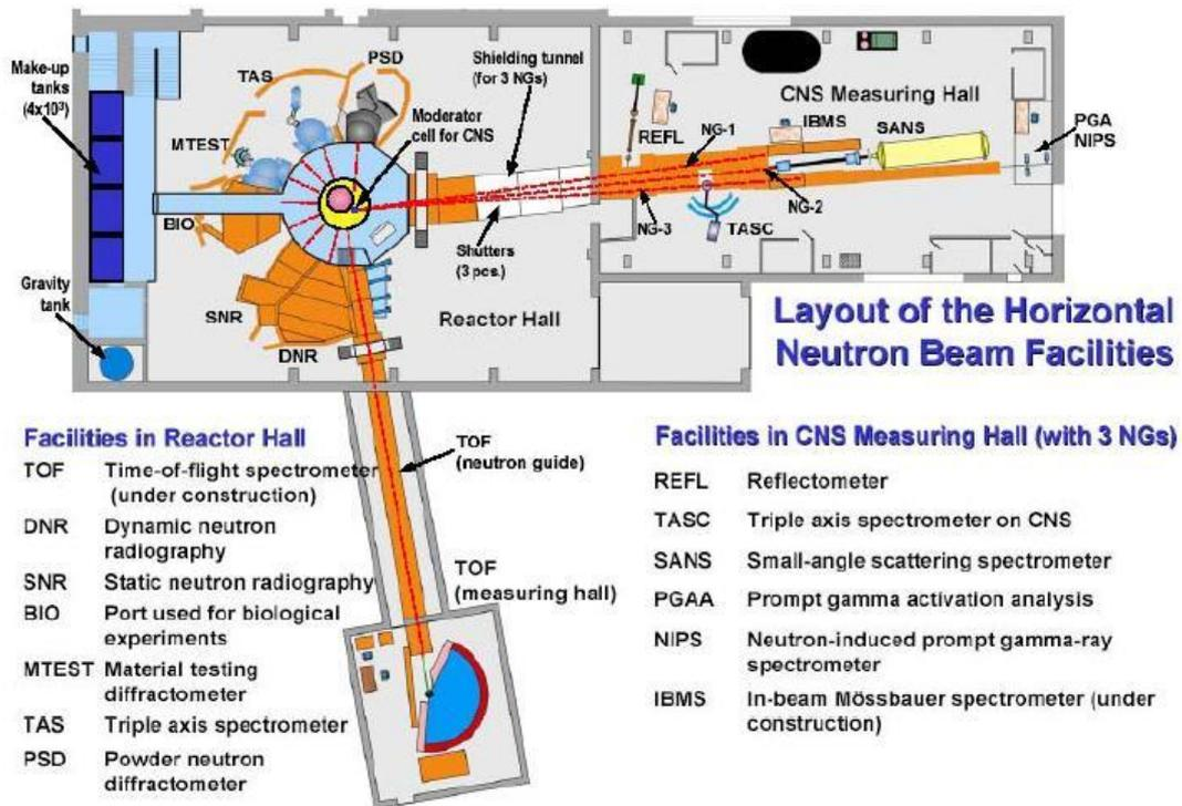
FIG. 1. Layout of the horizontal neutron beam facilities at the BRR.
