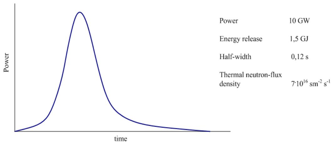
FIG. 3. Non-controlled pulse mode.
