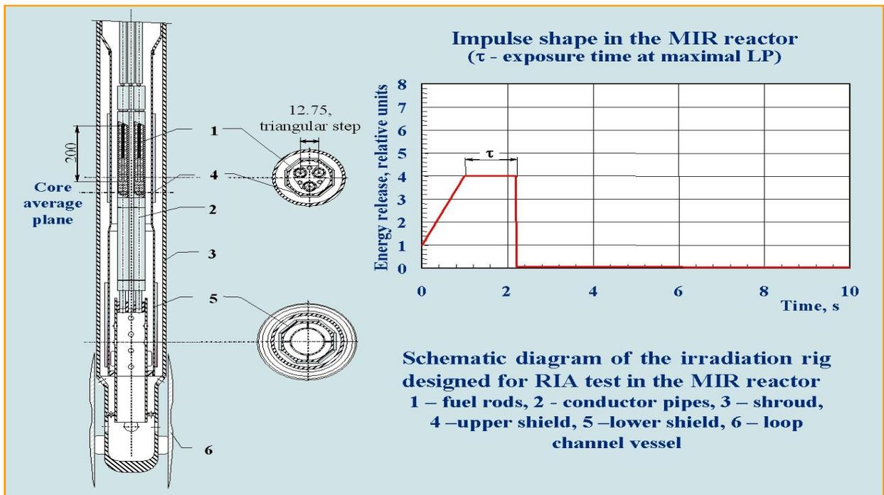
FIG. 11. Technique for simulation of reactivity inserted accident (RIA).
