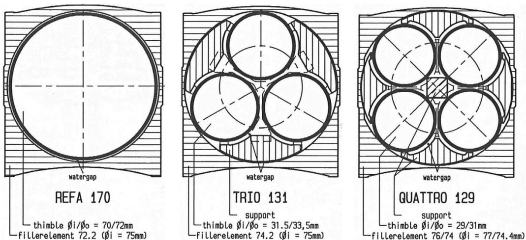
FIG. 3. Standard HFR irradiation rigs; outside water cooled, inside gas swept (mixtures of helium, neon, nitrogen); customisation possible.
