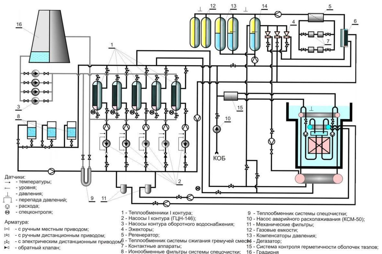
FIG. 4. Principle diagram of the primary circuit in reactor MIR.M1.
