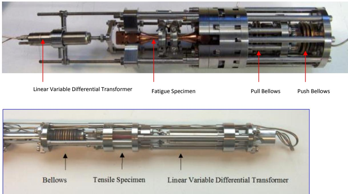
FIG. 9. COFAT: creep-fatigue test module.
