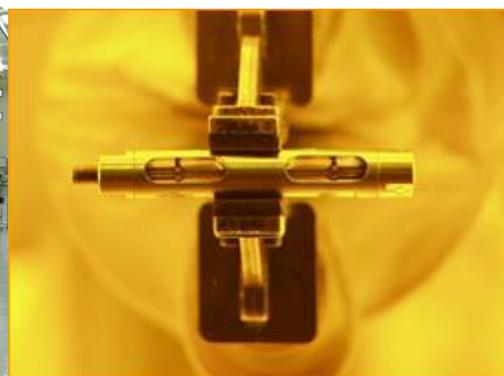
FIG. 5. Determination of the irradiation-induced stress relaxation behaviour of a bolt specimen.
