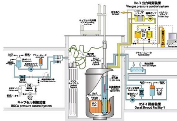
FIG. 5. Shroud irradiation facility.
