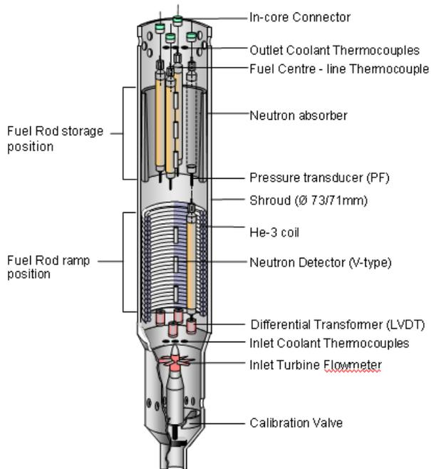
FIG. 4. Examples of irradiation rig for ramp testing.
