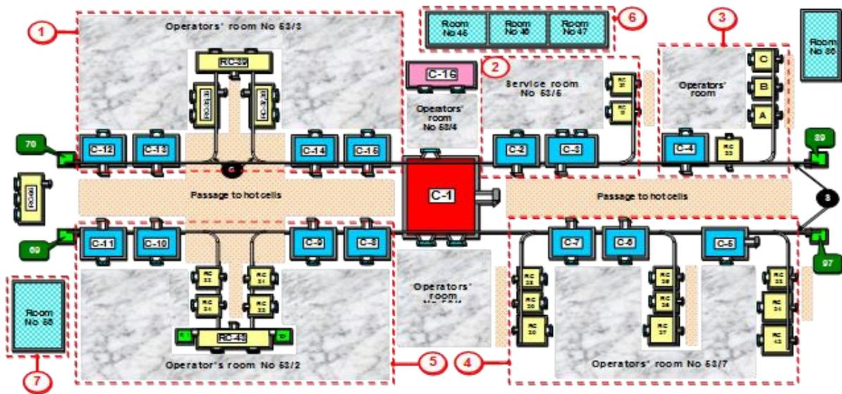
FIG. 9. Hot cells for destructive PIE.
