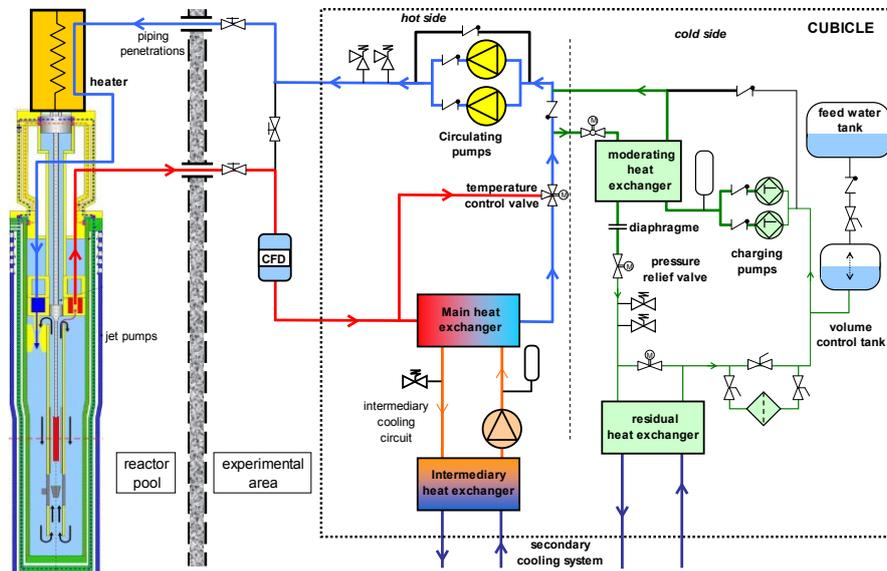
FIG. 6. Schematic diagram of the ADELIN loop.
