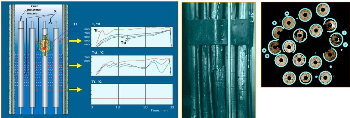
FIG. 10. Technique for simulation of loss of coolant and partial core dry-out accident (LOCA).
