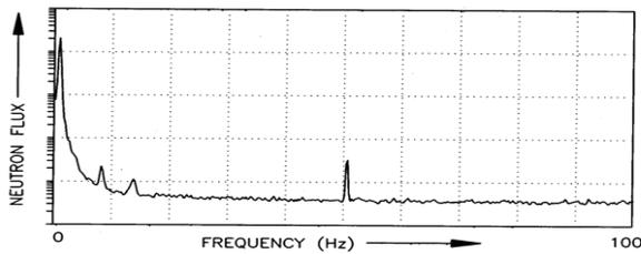
FIG. 9(a). Power spectrum of in-core neutron noise.
