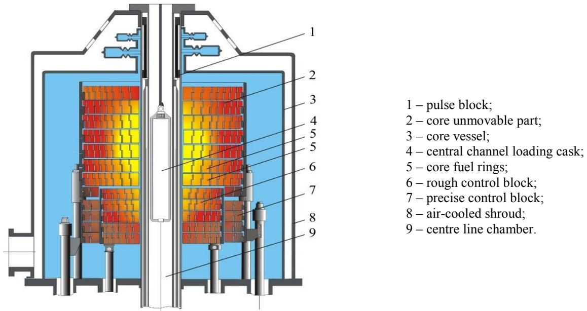
FIG. 2. BGR reactor section.
