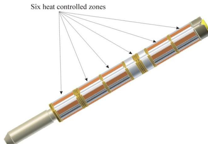
FIG. 2. Target holder, filled with specimens.
