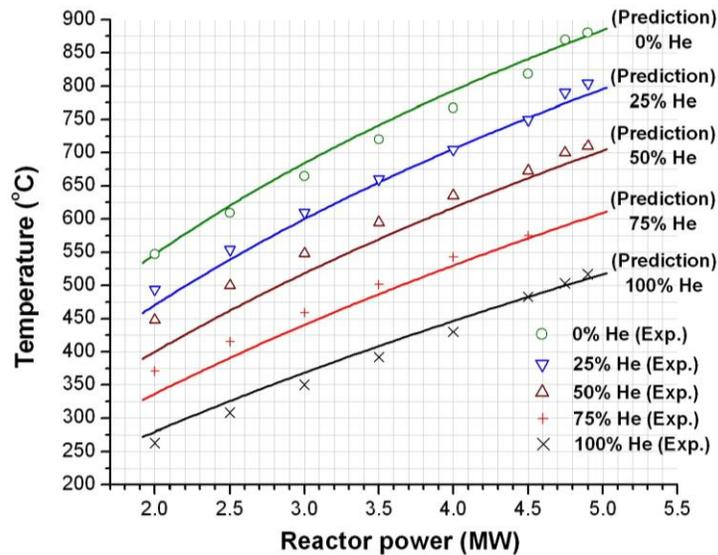
FIG. 8. Experimental verification ICSA with various gas mixtures.
