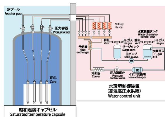
FIG. 6. SATCAP and water control unit.
