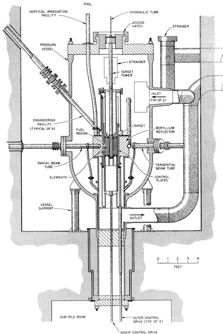
FIG. 3. Vertical cross-section through the reactor pool.
