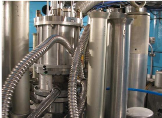
*FIG. 3. Assembled Bagira 3 in the reactor channel with the view of the rotating engine.*
