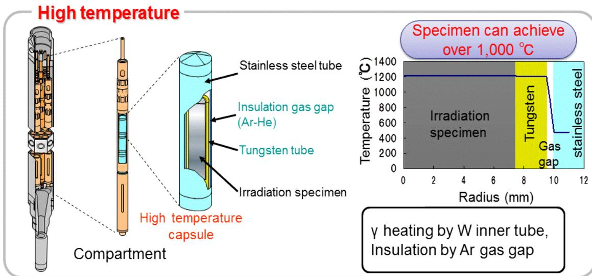
FIG. 6. Preliminary temperature calculation of high temperature irradiation capsule.
