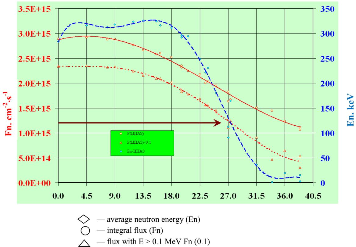
FIG. 5. Radial distribution of average neutron energy, total flux and flux with  $E > 0.1$  MeV.
