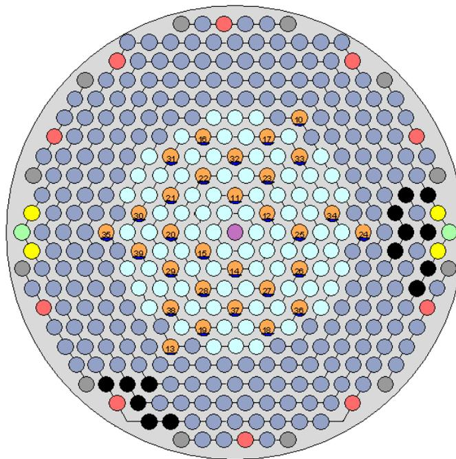
FIG. 2. Cross-section of Halden reactor core (light blue positions may contain experiments with fuel).
