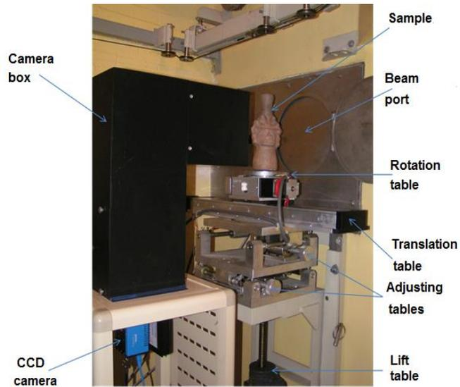
FIG. 7. ETRR-2 neutron radiography facility with its main components.
