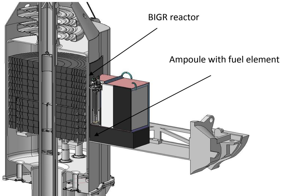
FIG. 5. Arrangement of RBM with an irradiating ampoule near the side surface of BIGR reactor.
