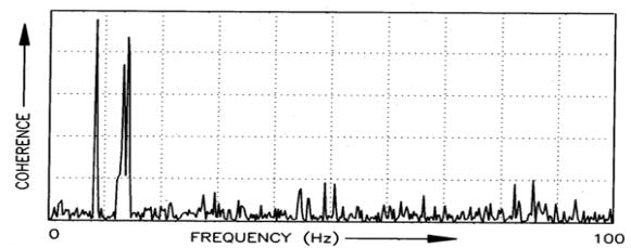
FIG. 9(b). Coherence of in-core neutron noise and mechanical vibration.
