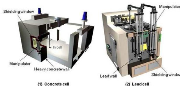
FIG. 14. Structure of the concrete cell and lead cell.
