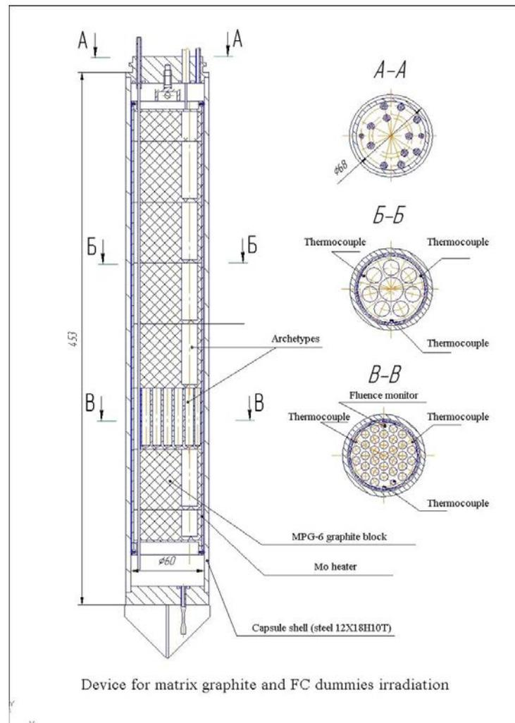
FIG. 5. Irradiation device for graphite testing.
