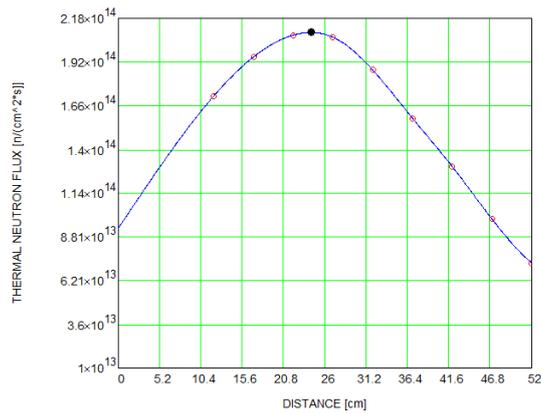
FIG. 4. Thermal neutron flux axial distribution in XC-1 channel ( $P = 11$  MW).
