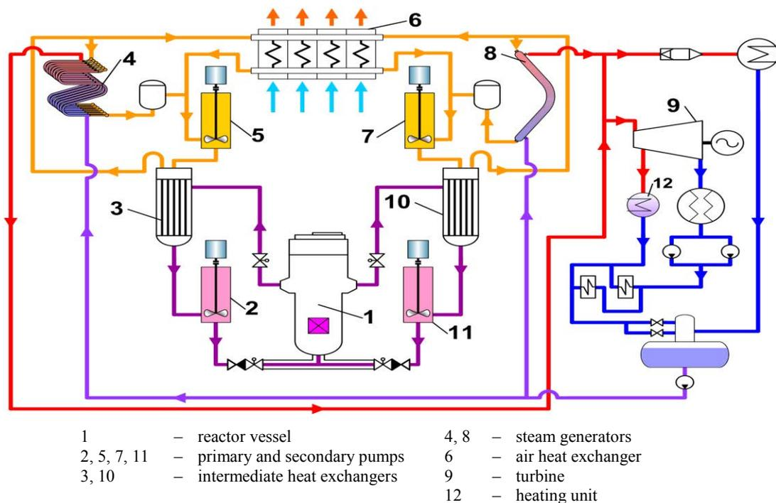
FIG. 2. The BOR-60 facility general circuit design.
