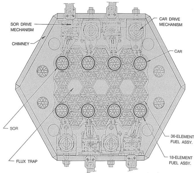
FIG. 4. Reactor core.
