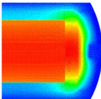
FIG. 9. Thermal calculation in OCCITANE device at 0.6 W/g.
