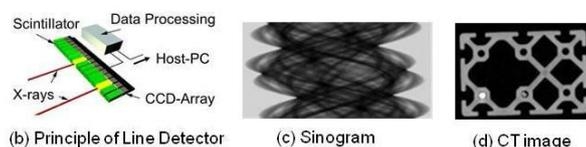
FIG. 15. Principle of X-ray CT.
