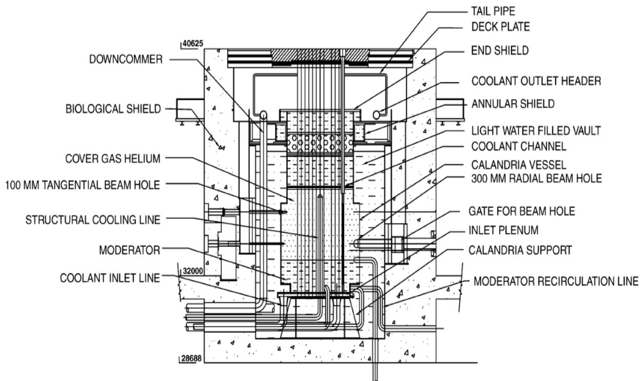
FIG. 1. General arrangement of DHRUVA reactor.
