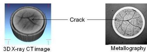
(c) Crack of the pellet
