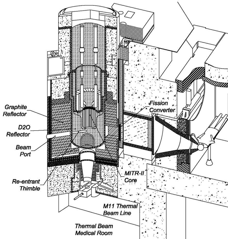
FIG. 2. Cutaway schematic of the MITR.
