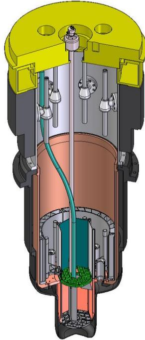
FIG. 4. Cutaway 3-D model of the MITR showing an ICSA (blue) and an in-core water loop installed in the reactor core (fuel elements removed for clarity).
