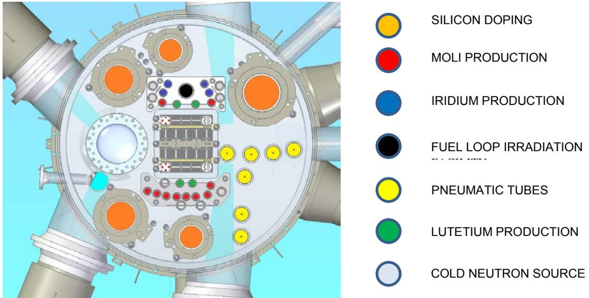
FIG. 2. The layout of RA-10 core.
