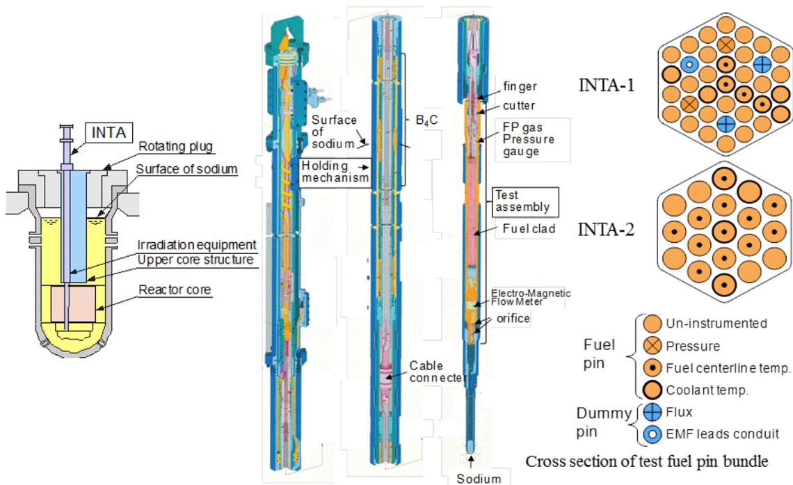
FIG. 8. Instrumented fuel test subassembly (INTA-1 and INTA-2).
