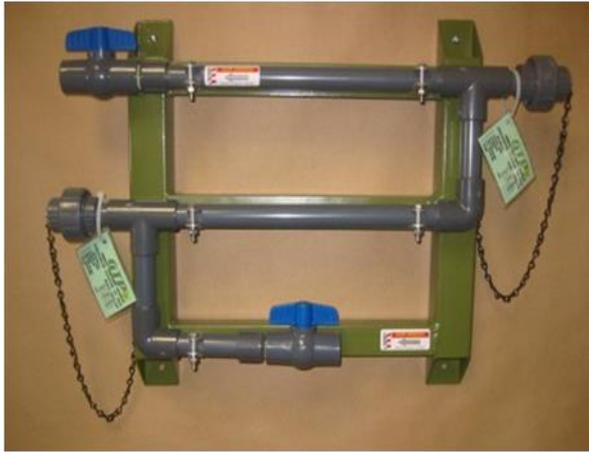
FIG. 9. Corrosion test rack.
