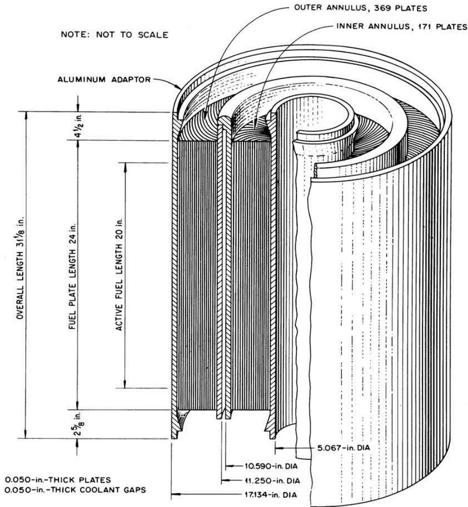
FIG. 4. HFIR fuel element assembly.
