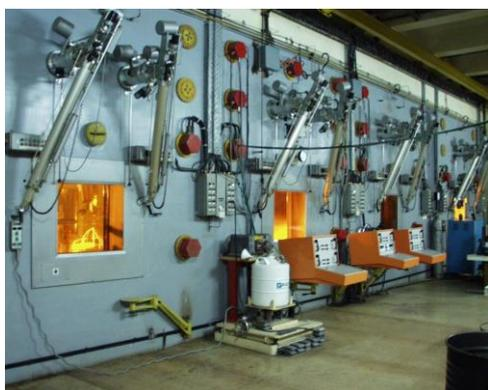
FIG. 18. Heavy concrete hot cell operating area.
