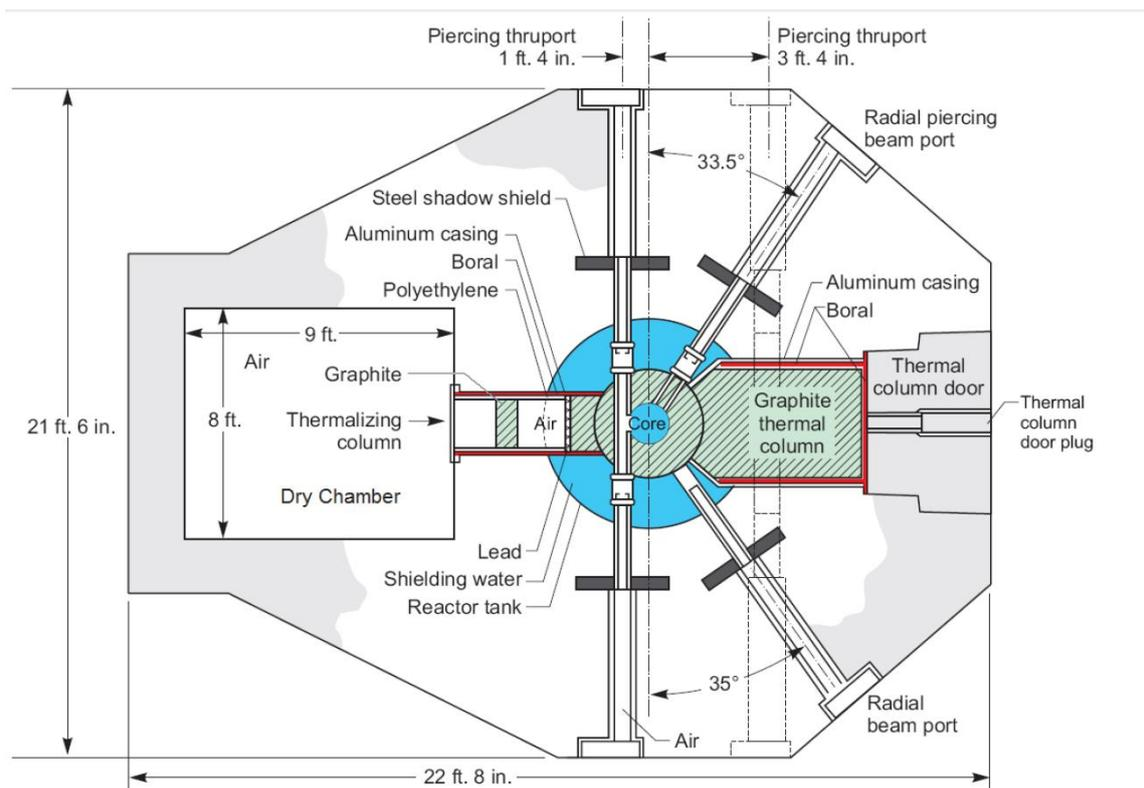
FIG. 1. Top view of the TRIGA reactor.
