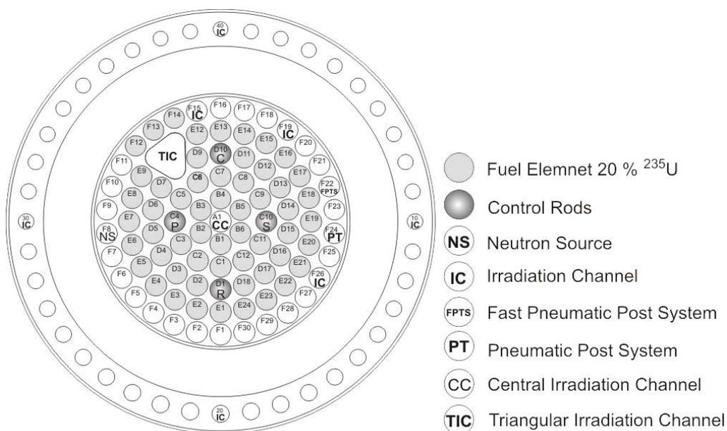
FIG. 2. Irradiation channels inside the reactor core and standard core configuration.
