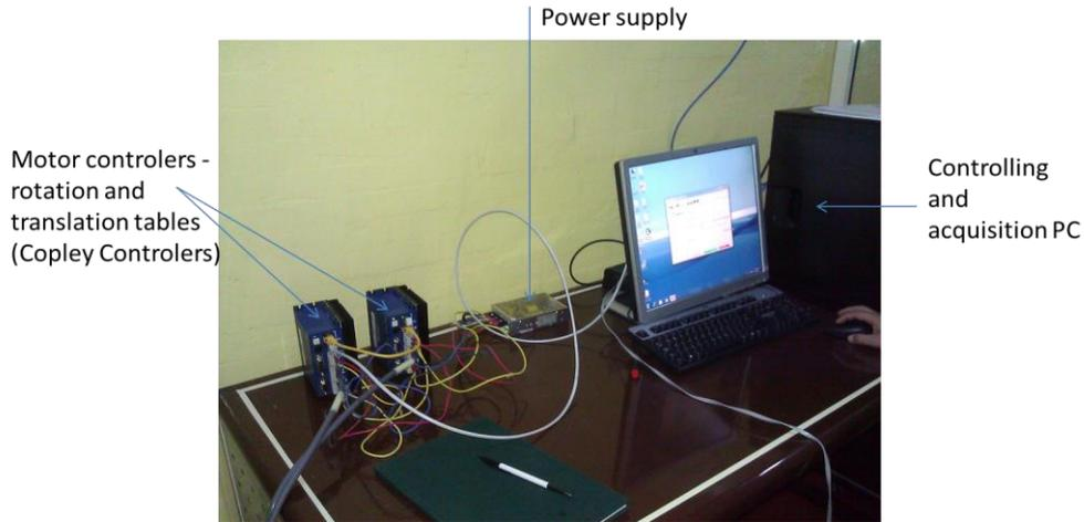
FIG. 8. Controlling and acquisition system of the neutron radiography.
