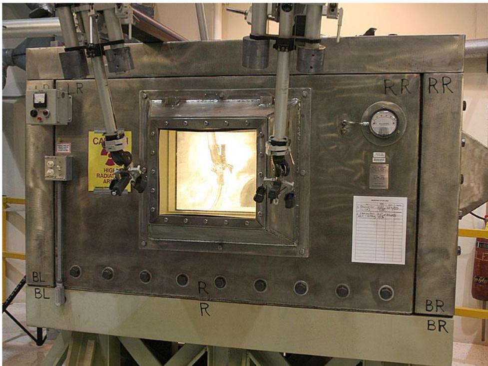
FIG. 13. Reactor floor hot box.
