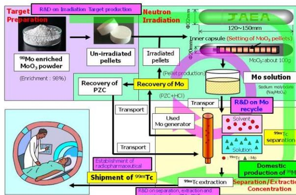
FIG. 21. Flow chart for the domestic production of  $^{99}\text{Mo}$ - $^{99\text{m}}\text{Tc}$  in JMTR.
