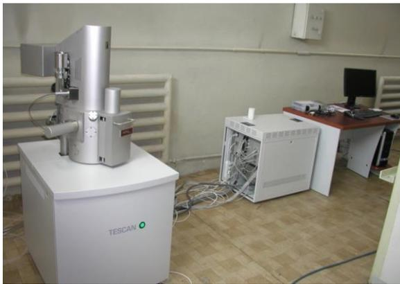
FIG. 25. TESCAN MIRA II LMU CS Schottky field emission variable pressure scanning electron microscope
