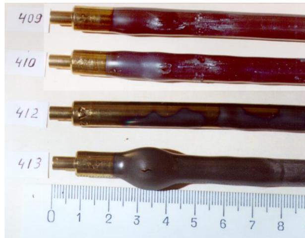
FIG. 5. WWER fuel samples after their irradiation in BGR reactor.
