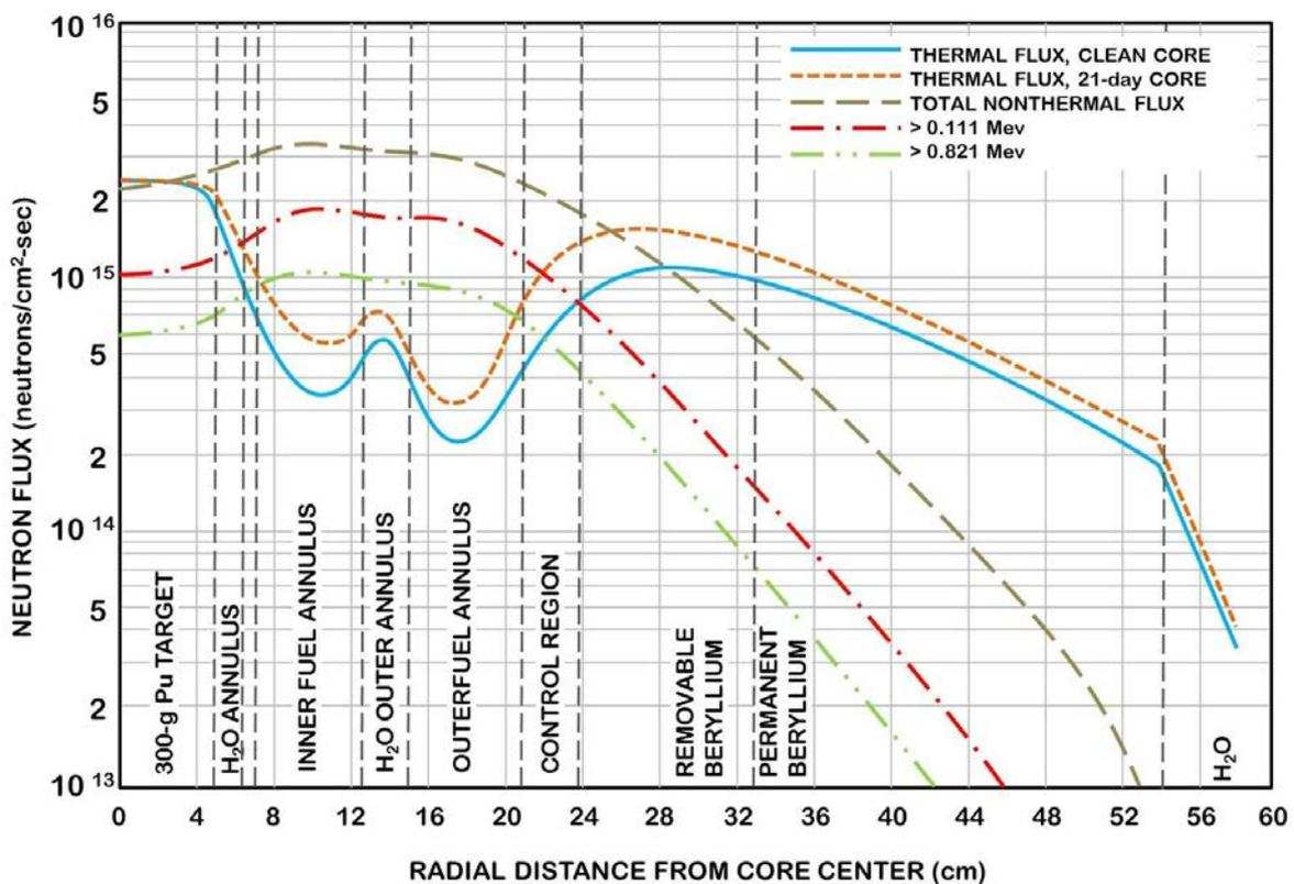
FIG. 6. HFIR neutron flux as a function of distance from the centerline of the core.
