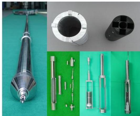
FIG. 9. Instrumented capsule for material test.
