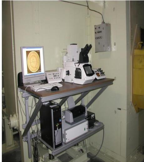
FIG. 24. Leica TELATOM 4, remote controlled inverted wide field metallographic microscope for radioactive materials.
