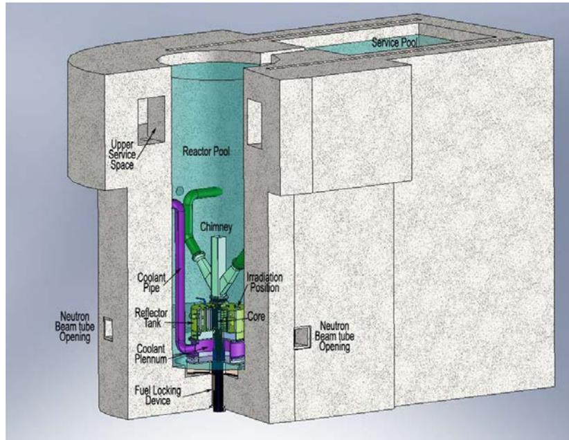
FIG. 3. Reactor pool block.
