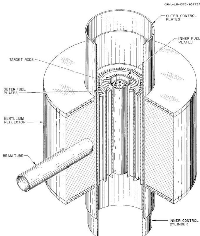
FIG. 4. Basic components of the HFIR core.
