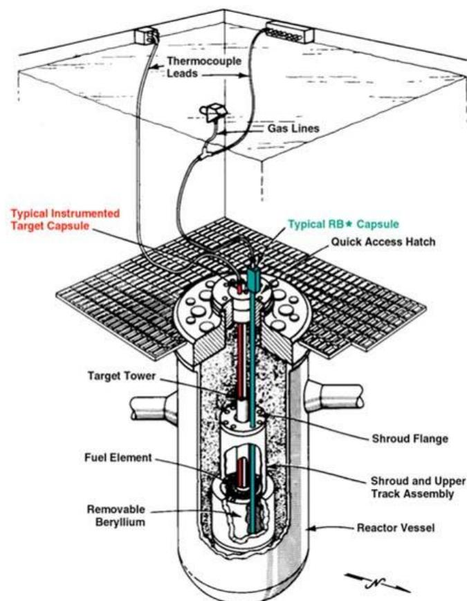
FIG. 12. Diagram of the HFIR materials irradiation facility (MIF).
