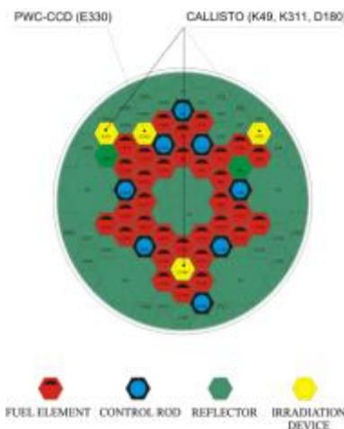
FIG. 2. BR-2 core cross-section.
