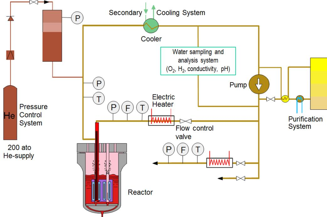
FIG. 3. Schematics of components in HBWR water loops.
