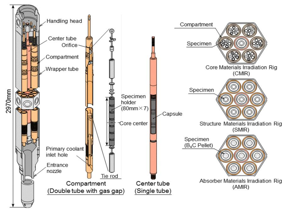
FIG. 5. Materials irradiation test rig.
