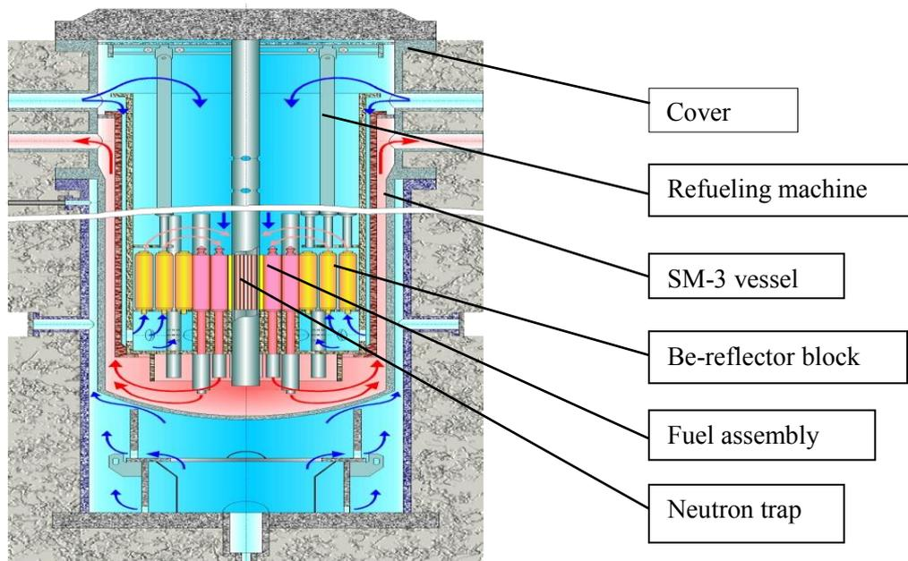
FIG. 2. The SM-3 longitudinal section.
