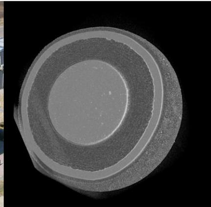
*FIG. 7. 3D XRT (X-ray tomography) visualization of a TRISO particle (PYCASSO experiment).*
