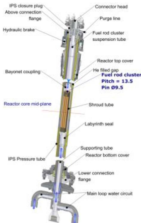
FIG. 3. View of CALLISTO experimental facility.
