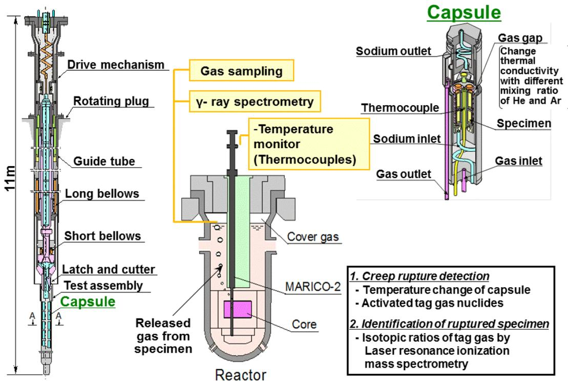
FIG. 9. Material testing rig with temperature control for in-pile creep investigation.
