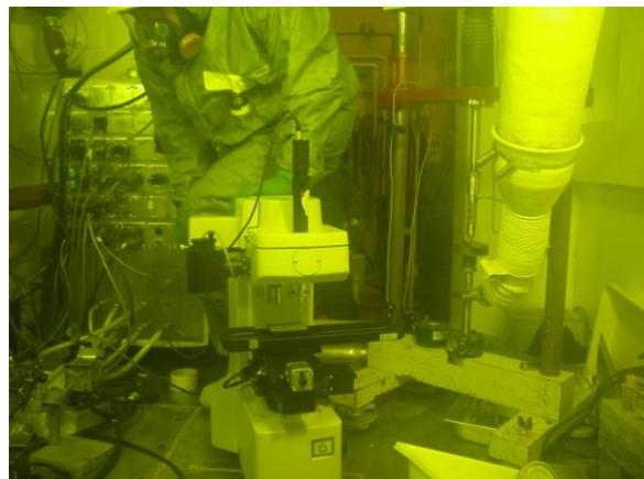
FIG. 14. In-cell creep testing (left) and in-cell hardness testing (right).
