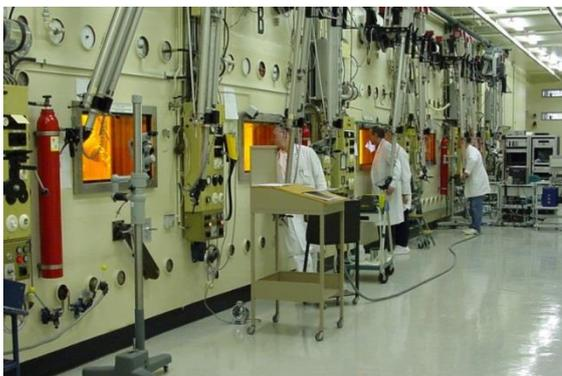
FIG. 4. Overview of part of the NRG hot cell facilities.
