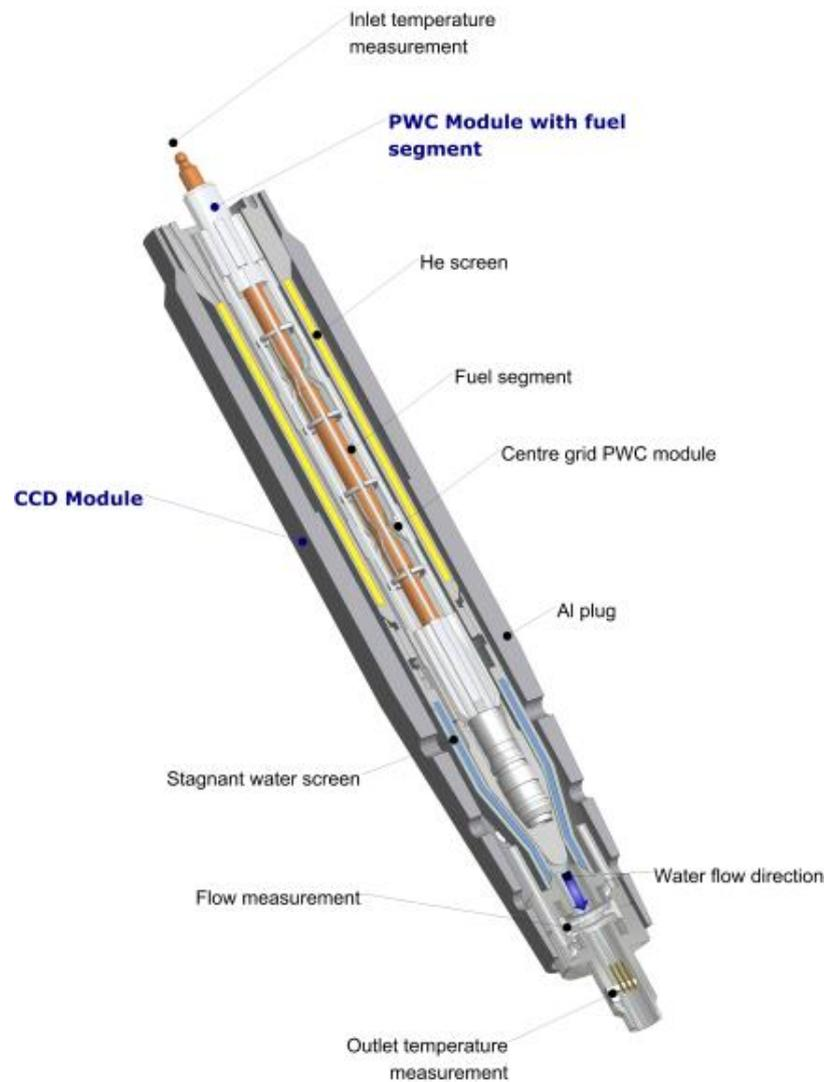
FIG. 10. The PWC/CCD irradiation rig.
