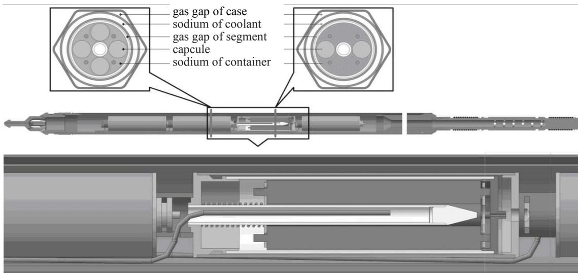
FIG. 7. General view of instrumented irradiation device.
