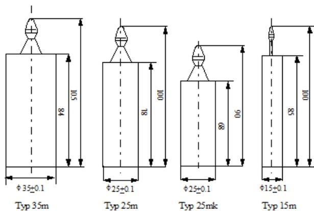
FIG. 1. Standard cans for irradiation target materials.
