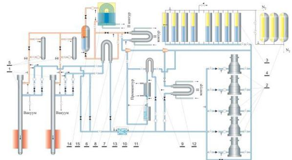
FIG. 6 (b). PVK-2 loop facility circuit.
