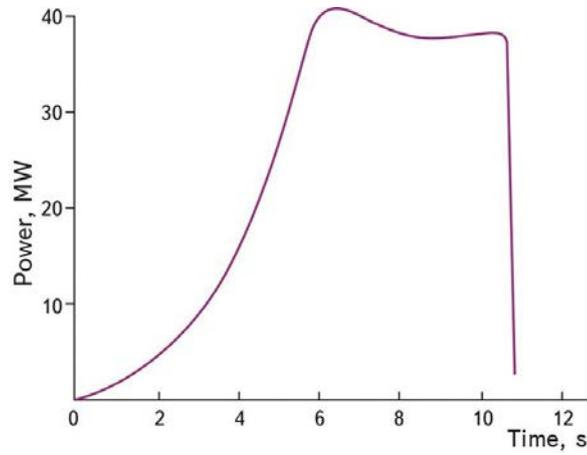
FIG. 4 (c). BGR quasi-pulse shape with runaway period 1.3 s and with power control.
