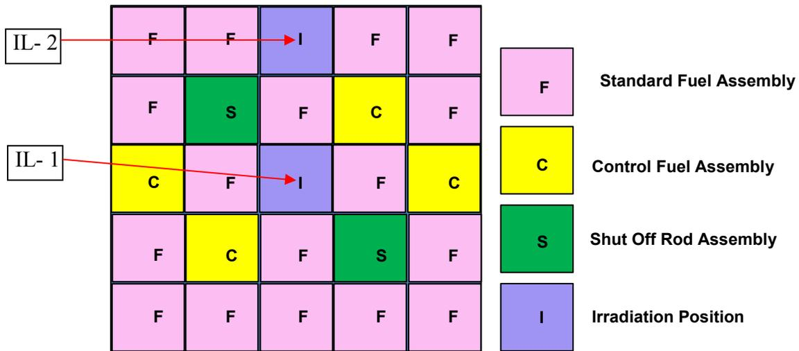
FIG. 1. Reactor core layout.
