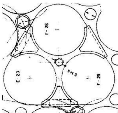
FIG. 14. Removable grid cavity.
