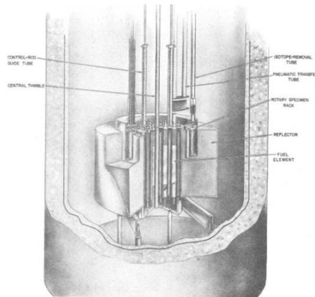
FIG. 11. Rotary specimen rack.
