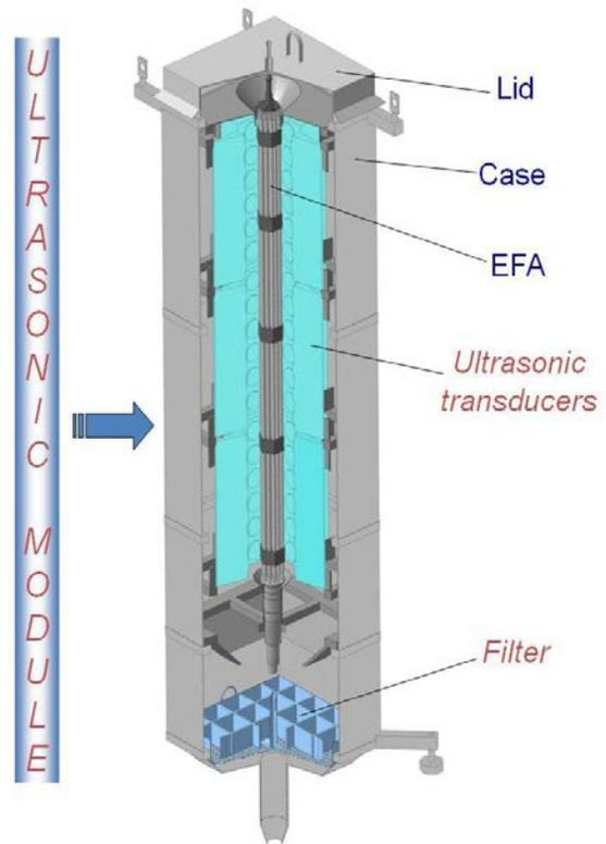
FIG. 13. Technique for irradiated fuel rods inspection and fuel rods ultrasonic cleaning facility in the MIR reactor storage pool.
