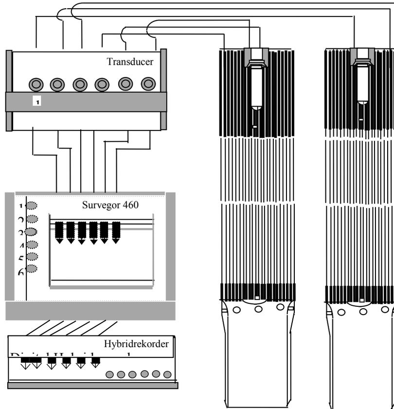
FIG. 7. Thermocouple located in instrumented fuel for temperature measurement.
