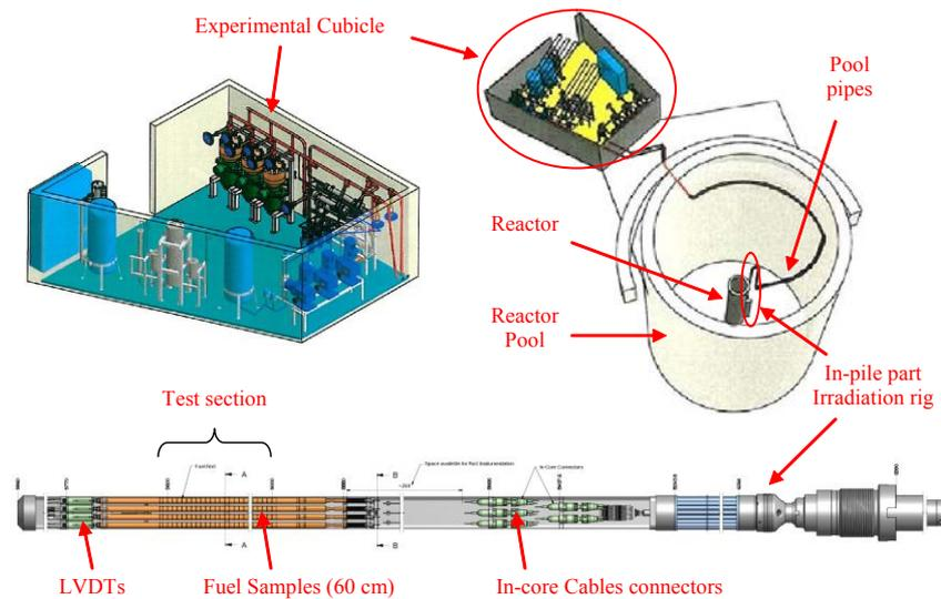
FIG. 5. View of the MADISON experimental device in the JHR facility with focus on the water loop in the experimental cubicle and on the first irradiation rig.
