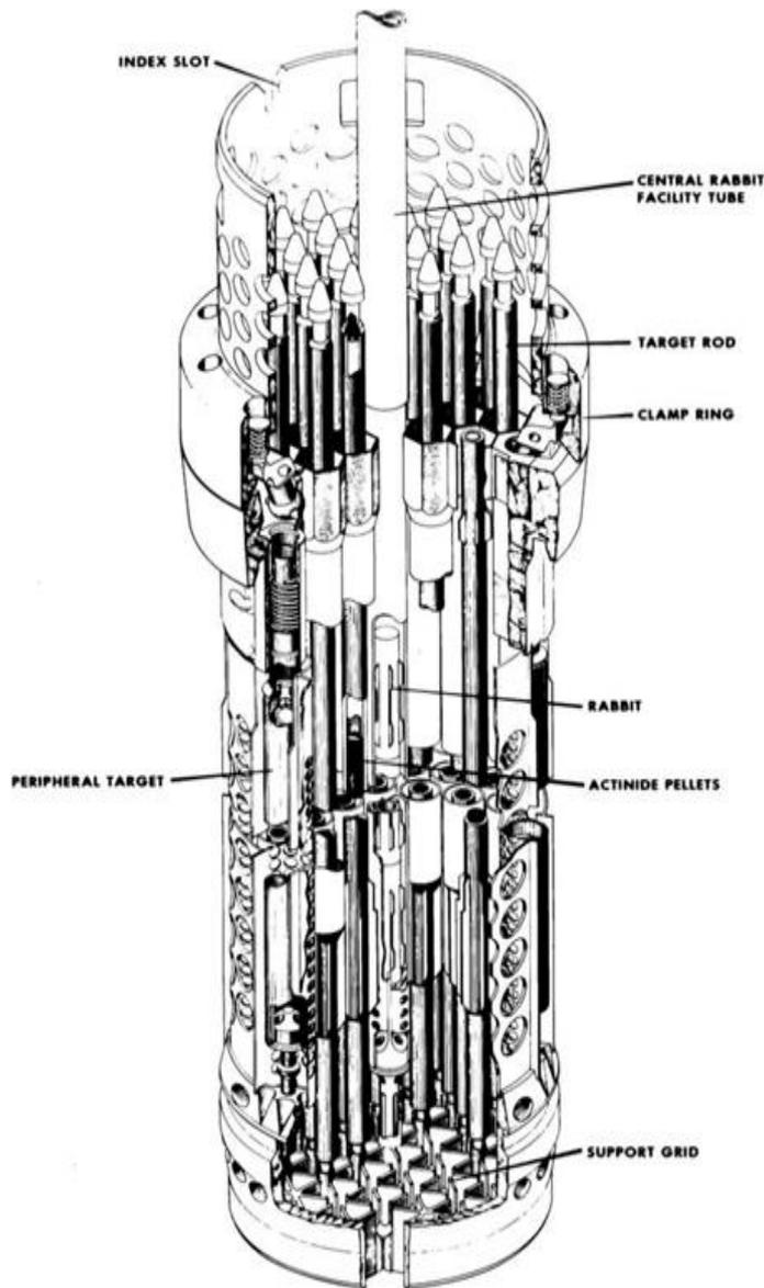
FIG. 10. Target basket in the HFIR flux trap.
