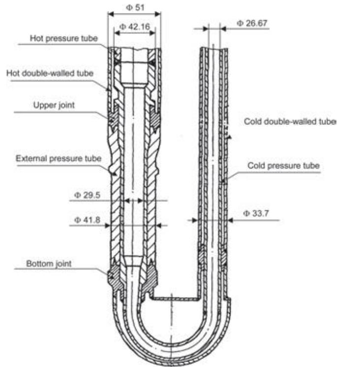
FIG. 13. Capsule C1/C2 in-pile section.
