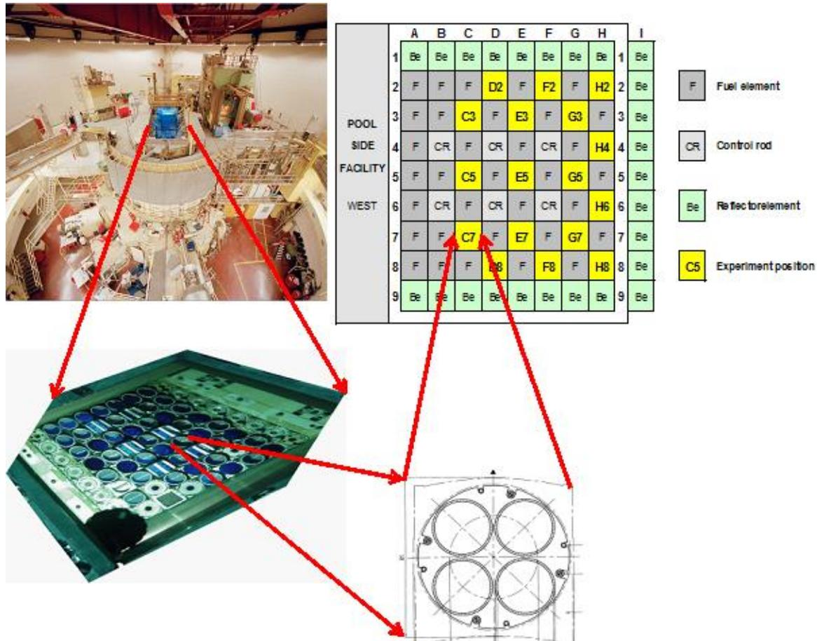
FIG. 2. Overview of the reactor hall, the basin, the core and the positioning of irradiation experiments.
