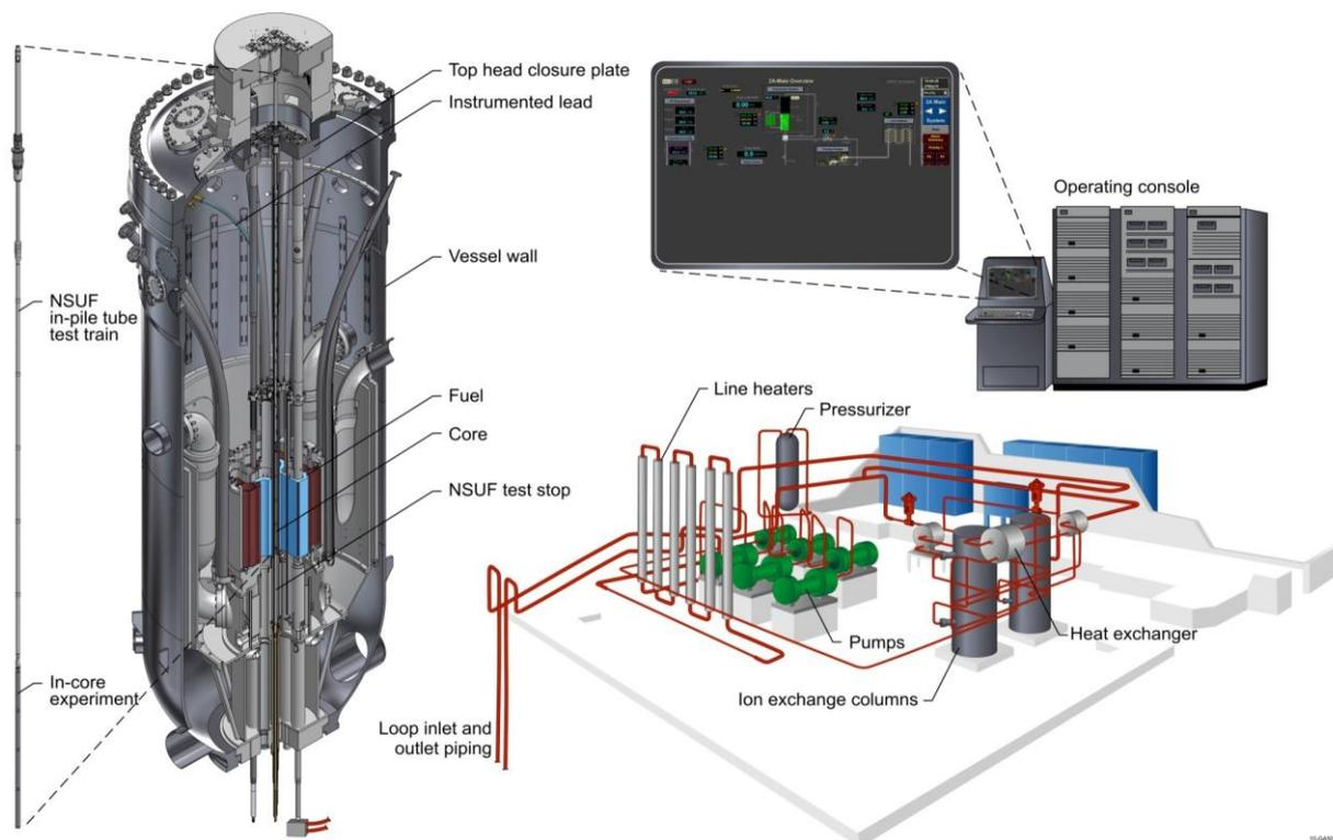
FIG. 3. In-pile tube (loop) in ATR with supporting systems.
