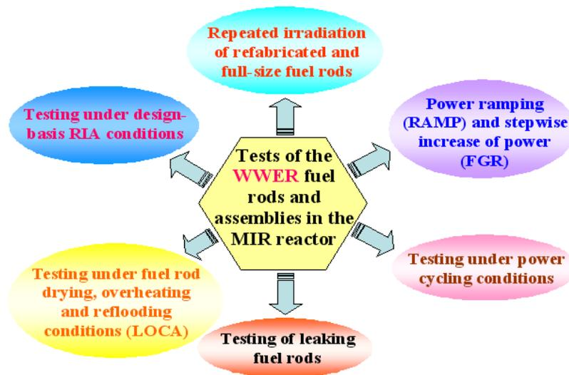
FIG. 15. Diagram of testing and investigation for improving WWER reactor fuel in the MIR reactor.
