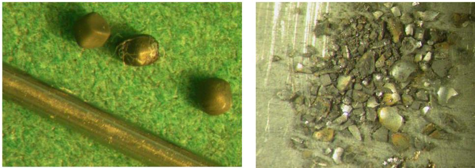
FIG. 6. Coated particle fuel before and after its irradiation in BGR reactor.
