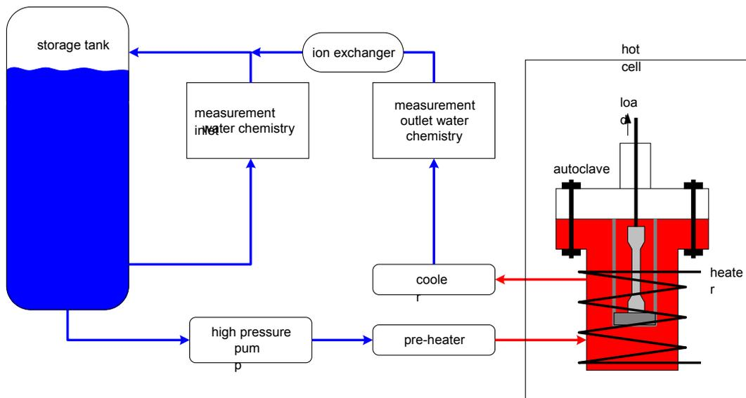
FIG. 8. Schematic of the hot cell installation.
