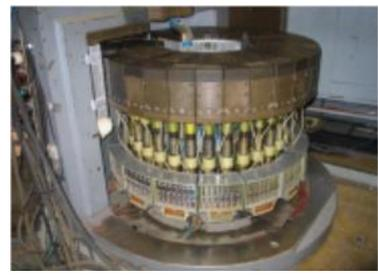
FIG. 4(c). DISK diffractometer.
