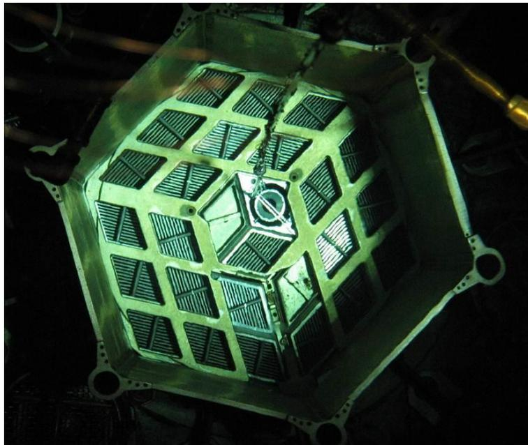
FIG. 3. Photograph of the MITR core with two solid dummy fuel elements and in-core experimental facility installed.
