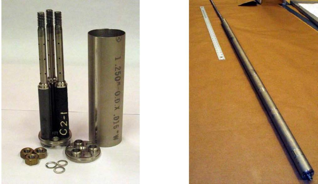
FIG. 6. Photographs of a sample module during assembly and the fully assembled sample stack before insertion into the autoclave.
