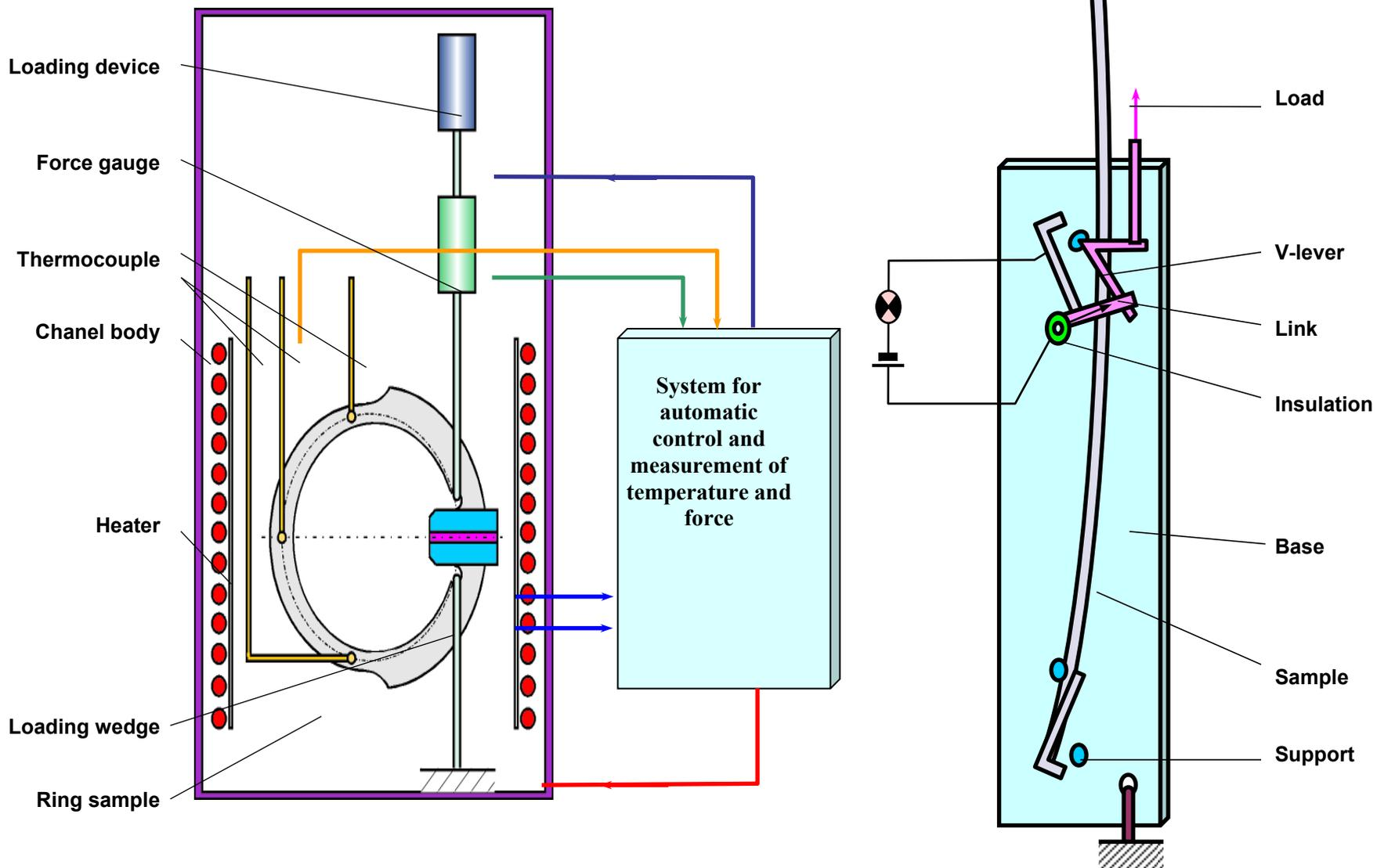
FIG. 3. Facility to test stress relaxation under bend in the ring or flat samples under irradiation.
