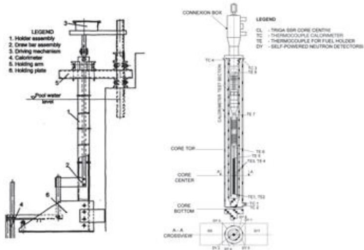
FIG. 16. Mechanical structure and instrumentation of capsule C9.
