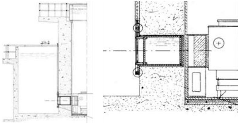
FIG. 10. Sections of the shielding tank and of thermalizing column.
