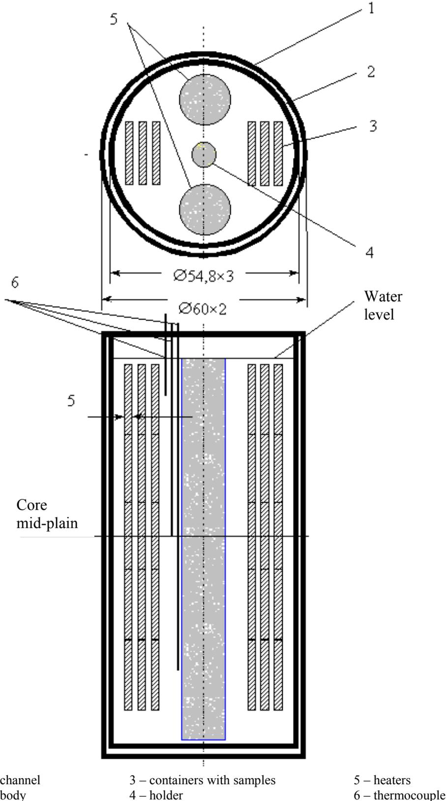
FIG. 7. Capsule to irradiate copper alloys for ITER divertor.
