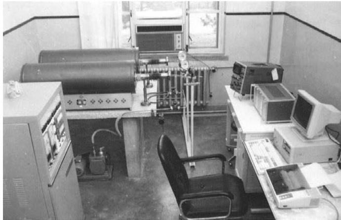
FIG. 7. Photo of Fuel-Cladding chemical interaction out-of-pile test facility.
