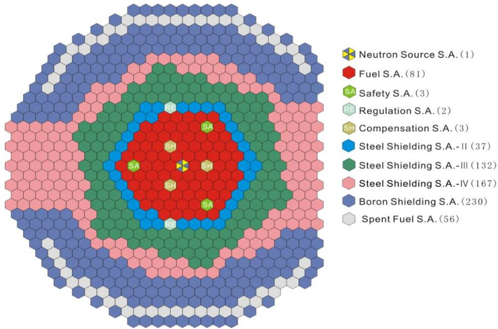
FIG. 1. The layout of CEFR core.
