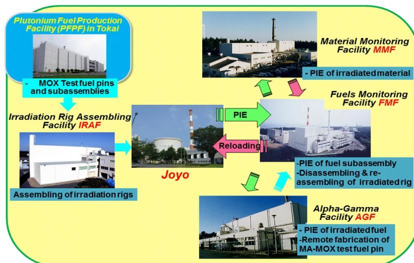
FIG. 11. Test fuel fabrication and hot laboratories related to JOYO.
