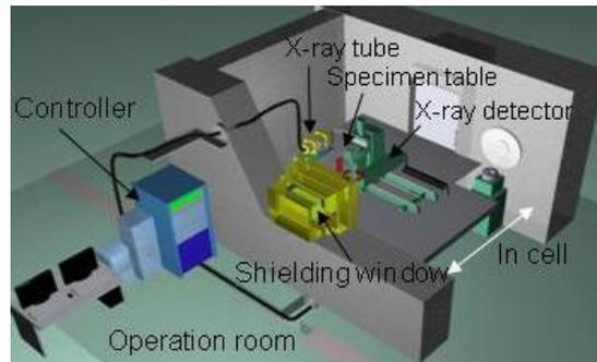
FIG. 16. Schematic drawing of 3D X-ray CT.
