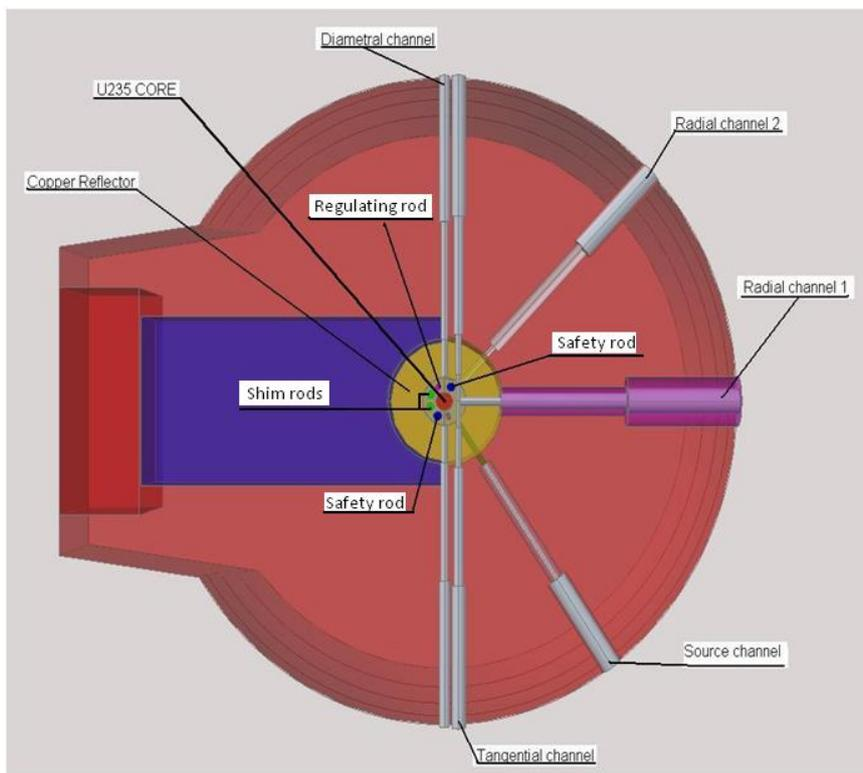
FIG. 5. Horizontal reactor section.
