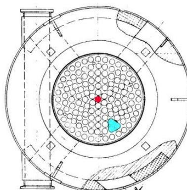
FIG. 15. Core position of the removable grid cavity.
