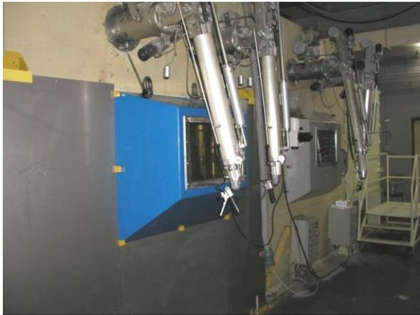
FIG. 20. Steel hot cell operating area.
