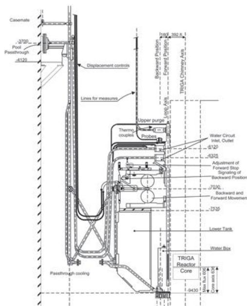
FIG. 10. The in-pile section of Loop A.
