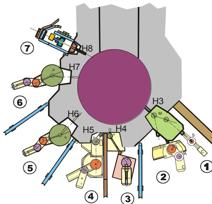
FIG. 7. Horizontal neutron beam channels.
