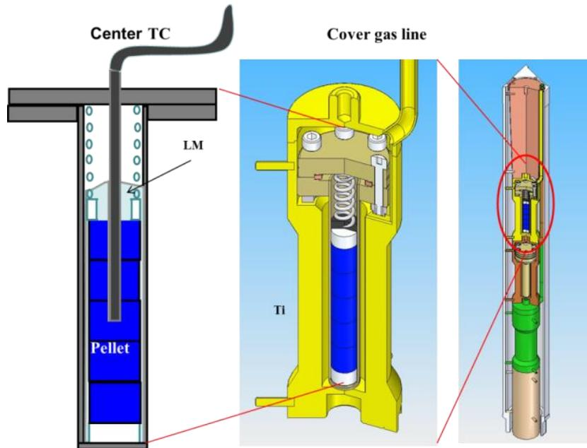
FIG. 7. HYFI fuel rod, capsule, and loaded dummy element cross sections.
