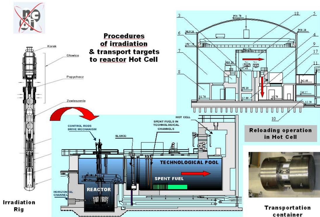
FIG. 6. Technology irradiation uranium targets (HEU) for <sup>99</sup>Mo production.
