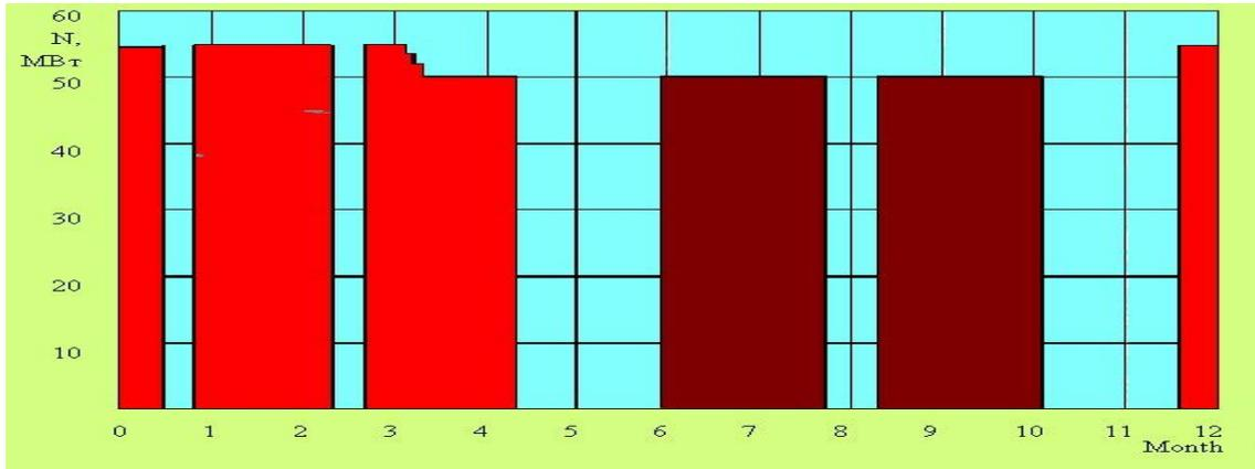
FIG. 4. Typical annual diagram of the BOR-60 reactor operation.
