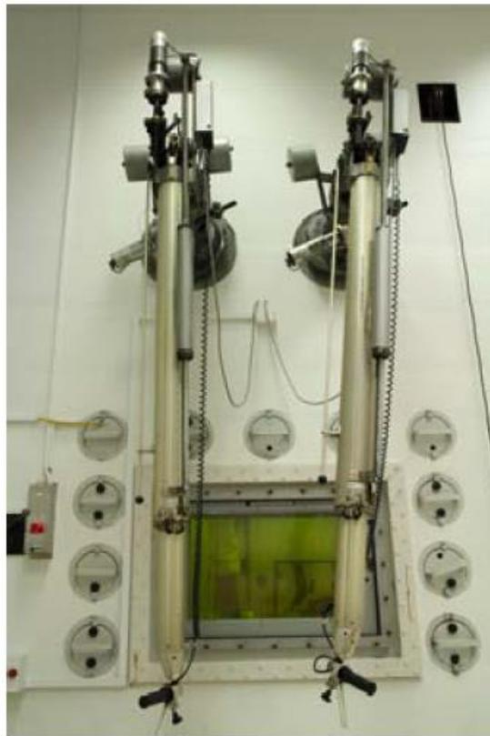
*FIG. 3. Master-slave manipulators in hot cell.*
