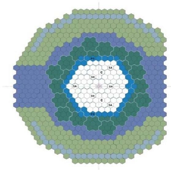
FIG. 3. The layout of CEFR core.
