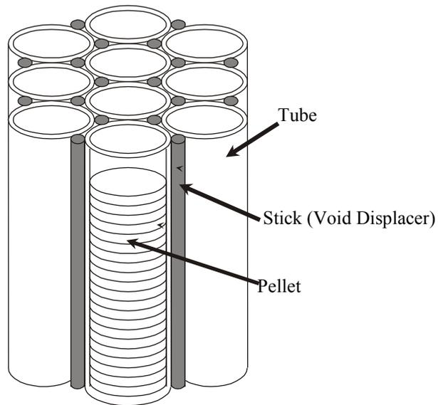
FIG. 4. Sample rod structure of the BFS assemblies.
