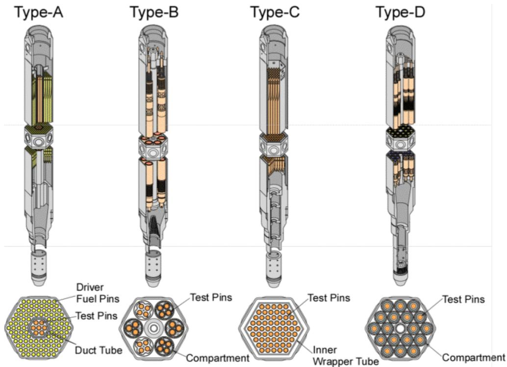
FIG. 3. Fuel irradiation rigs lineup in JOYO.
