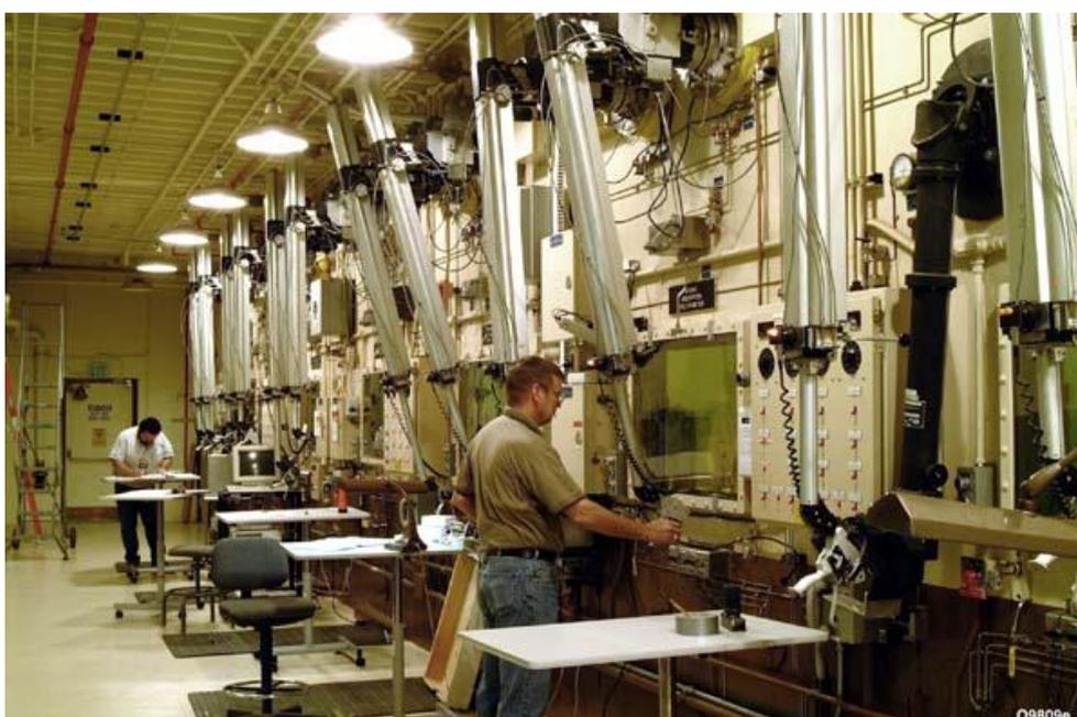
FIG. 8. Hot cells within the Analytical Laboratory.
