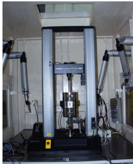
FIG. 26. INSTRON 5569 50 kN tensile testing machine.
