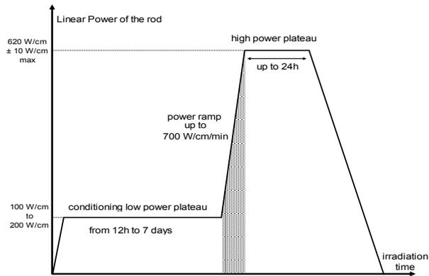
FIG. 7. Standard power ramp test time history.
