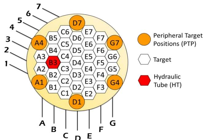
FIG. 9. Target region irradiation positions.
