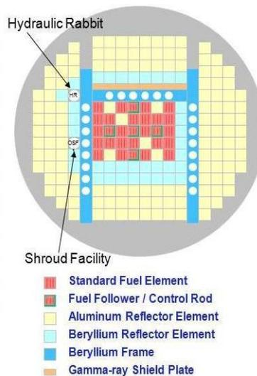
FIG. 2. Cross section of the core.
