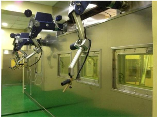
FIG. 10. Semi-hot cell for mechanical testing.
