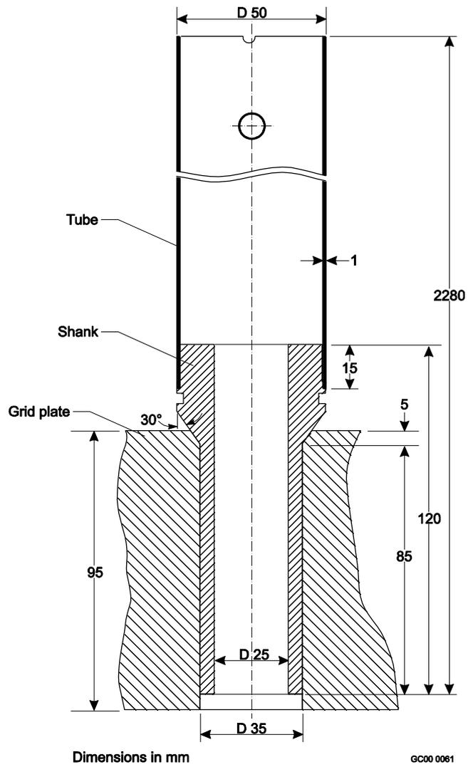
FIG. 5. Tube fixed in grid plate.
