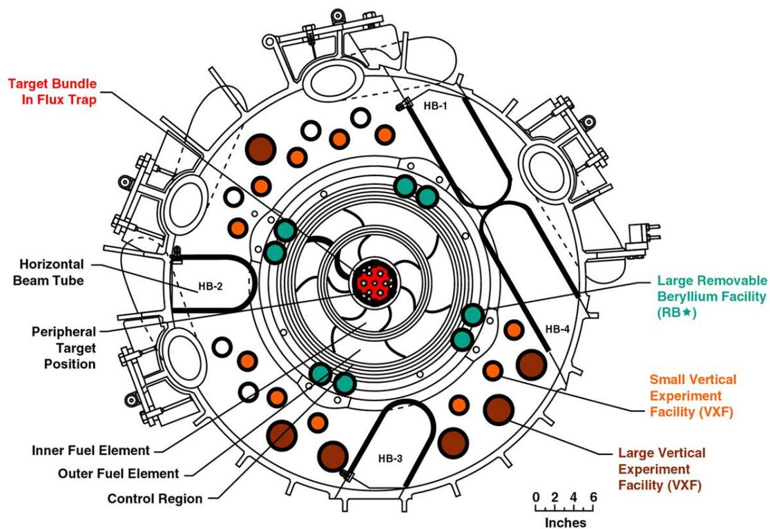
FIG. 7. Experiment positions at HFIR.
