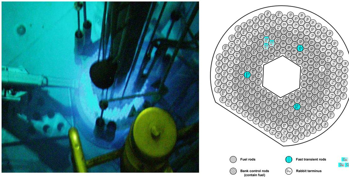
FIG. 7. ACPR reactor core in operation and core map.
