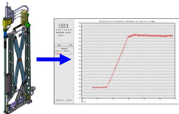
FIG. 3. View of a displacement system in the Beryllium reflector and an example of a realistic power ramp profile achievable in the JHR facility.
