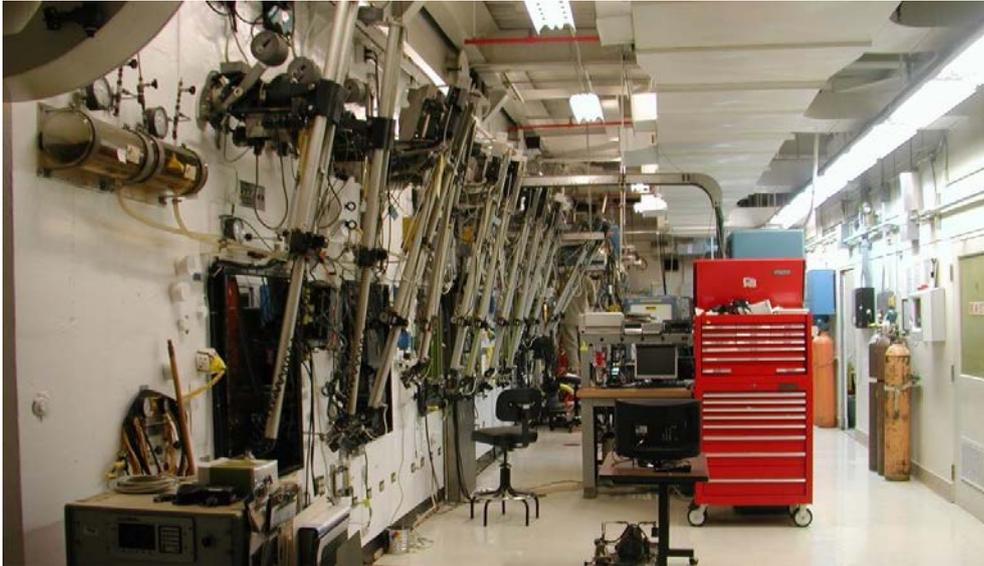
FIG. 13. Cell bank at the irradiated material examination and testing facility (IMET).
