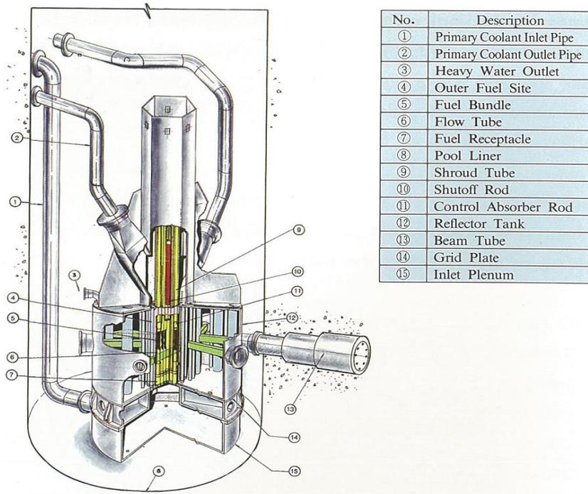
FIG. 3. Reactor structure assembly.
