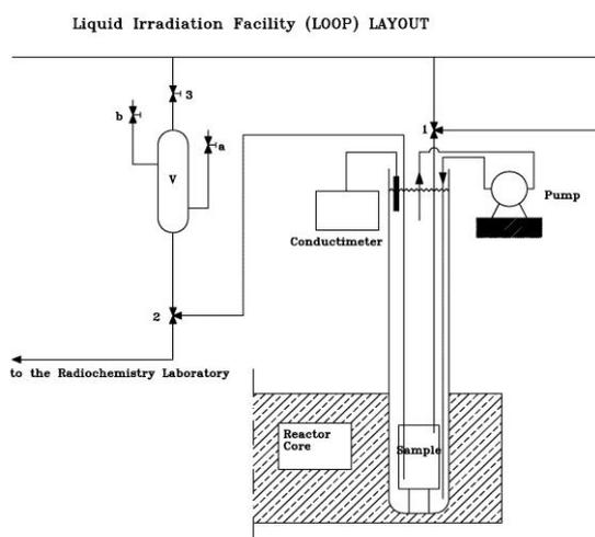
FIG. 16. Layout of the liquid irradiation facility (LOOP).
