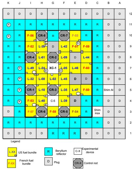
FIG. 3. Layout of TRIGA14MW reactor core.
