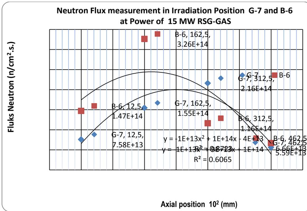
FIG. 6. Axial power distribution represented by flux neutron measurement (done at the 64<sup>th</sup> silicide reactor cycle).
