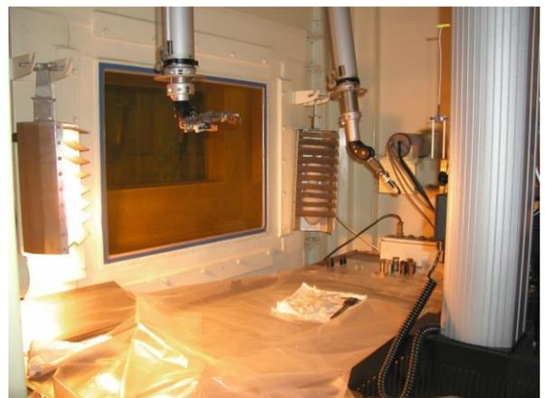
FIG. 23. Working station No.2 inside lead hot cell.
