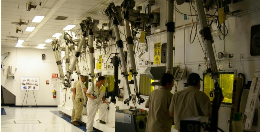
FIG. 15. Irradiated fuels examination laboratory (IFEL).
