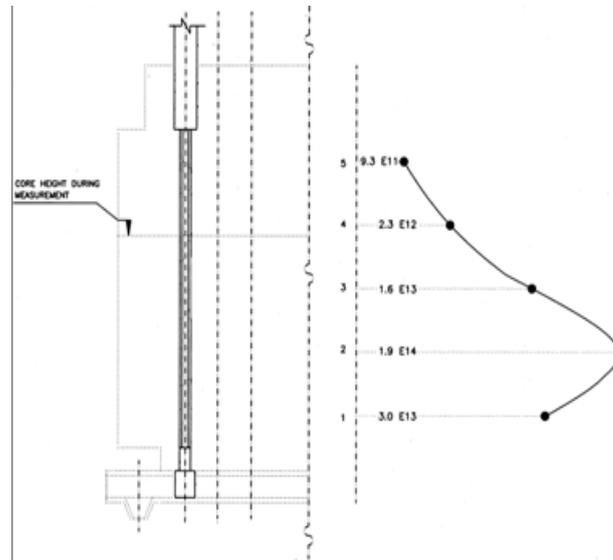
FIG. 8. Axial flux pattern.
