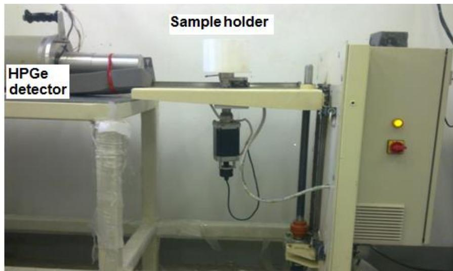
FIG. 14. Counting facility for LSNA at ETRR-2.
