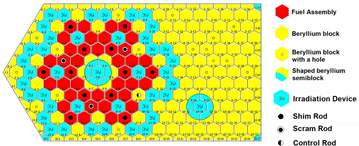
FIG. 1. IVV-2M reactor core with an experimental device in the central cell.
