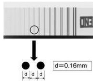
FIG. 17. Resolution performance test.
