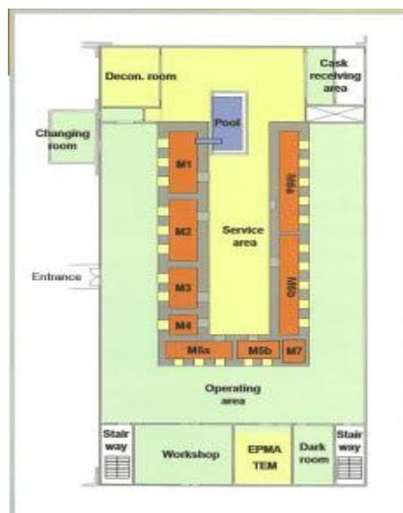
FIG. 12. IMEF hot cell layout.
