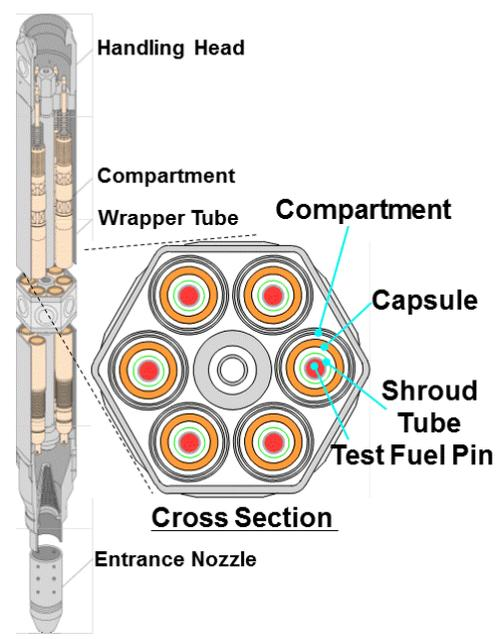
FIG. 4. Capsule type fuel irradiation rig.
