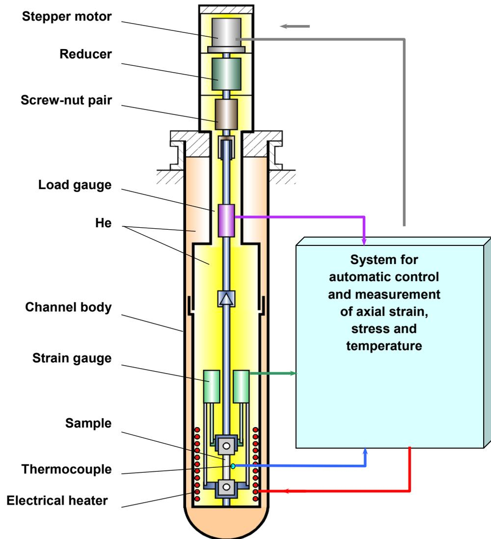
FIG. 2. 'Neutron' facility for tensile tests.
