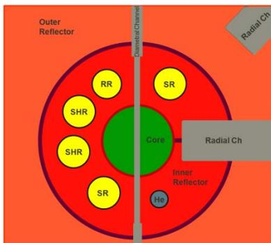
*Control rods* — five control rod made of copper with a driving distance of 150 mm
