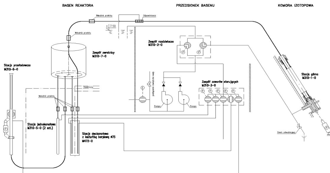
FIG. 3. Irradiation channel equipped with hydraulic system.
