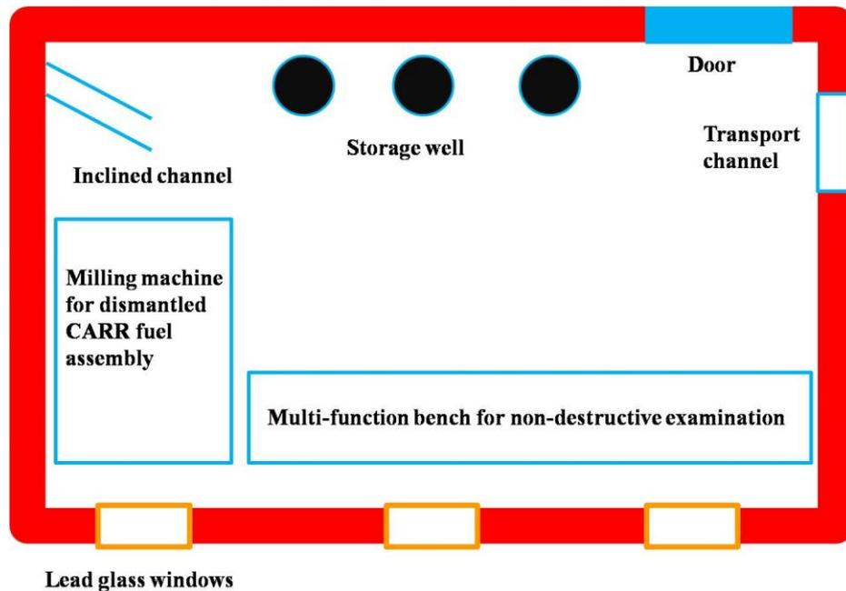
FIG. 4 Layout of CARR hot cell
