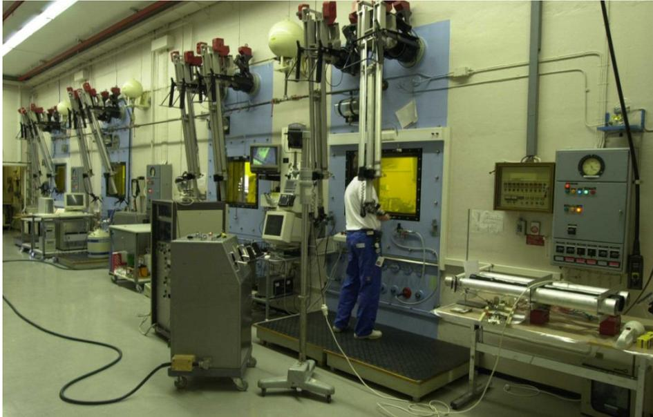
FIG. 5. Shielded cells for re-fabrication of irradiated fuels and post-irradiation examinations.
