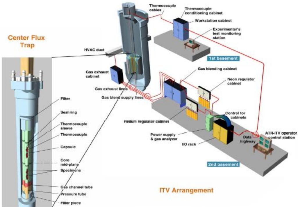
FIG. 4. ITV and online control and data acquisition systems.
