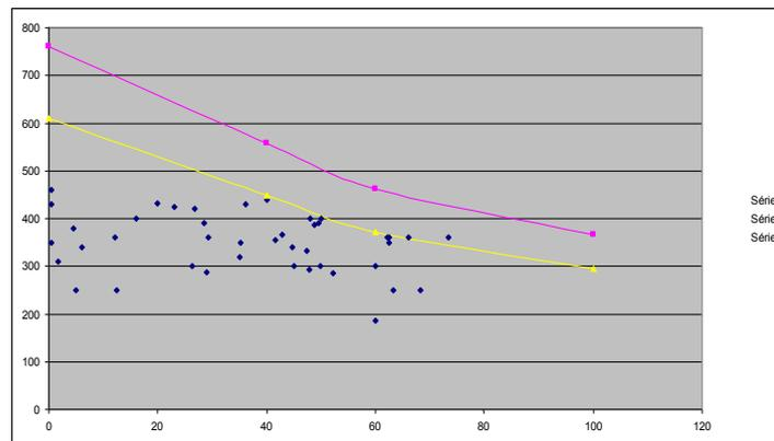
**Note:** Comparison of former PWR fuel experiments performed in MTRs (blue dots) with MADISON calculated performances:
