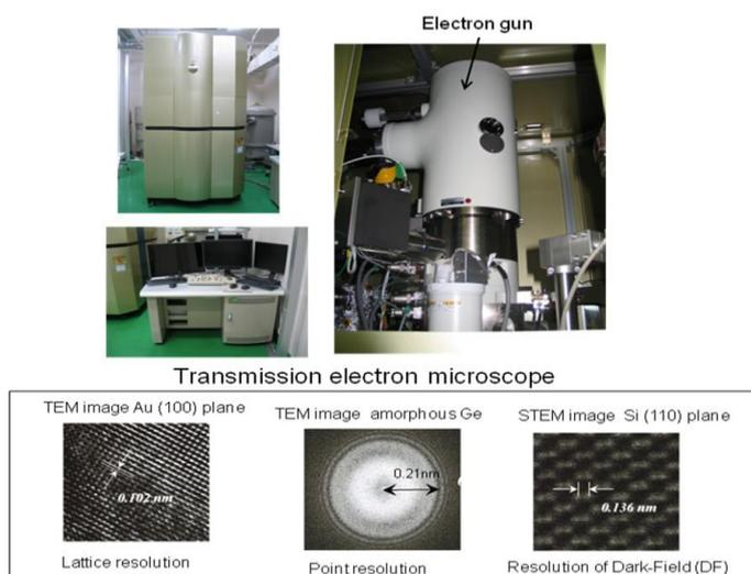
FIG. 19. Photo of TEM and typical obtained image.
