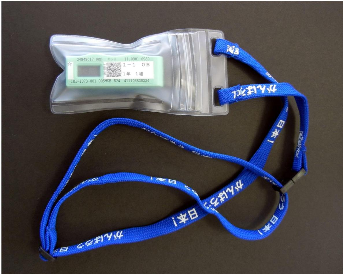
FIG. I-2. Glass badge used for personal measurement of external dose [I-5]. (Photograph courtesy of Chiyoda Technol Corporation).
