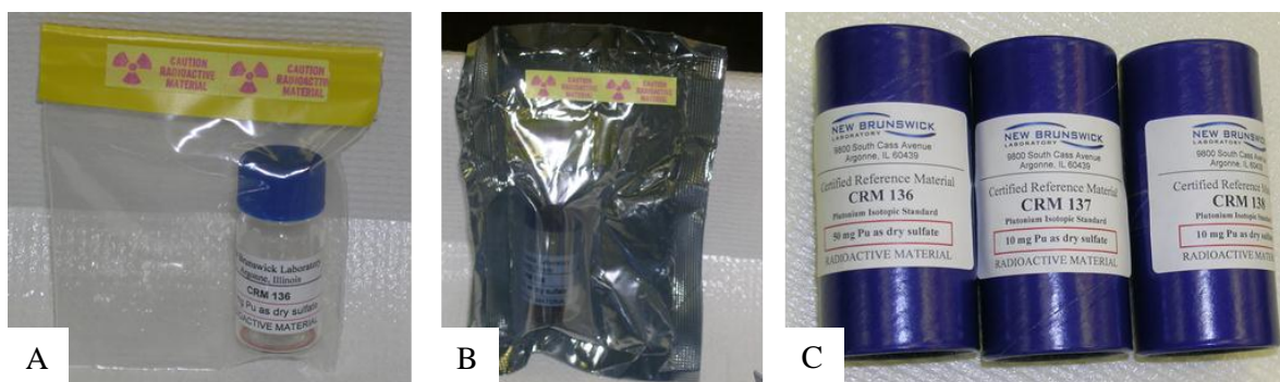
Figure 2: Newly re-packaged standards in A) first tape sealed, zip lock bag, B) second, heat-sealed, Mylar bag, and C) final container ready for shipping.
