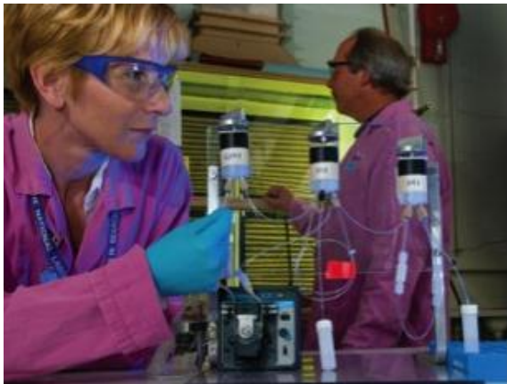
Figure 5. Gas Pressurized Extraction Chromatography (GPEC) that was used for Cs/Ba separations.
