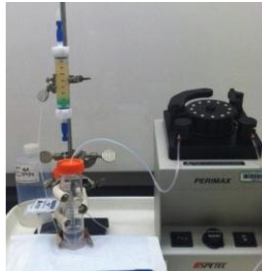
Figure 6. Omnifit column system with DOWEX 1x8 resin that was used for Co/Ni separations.
