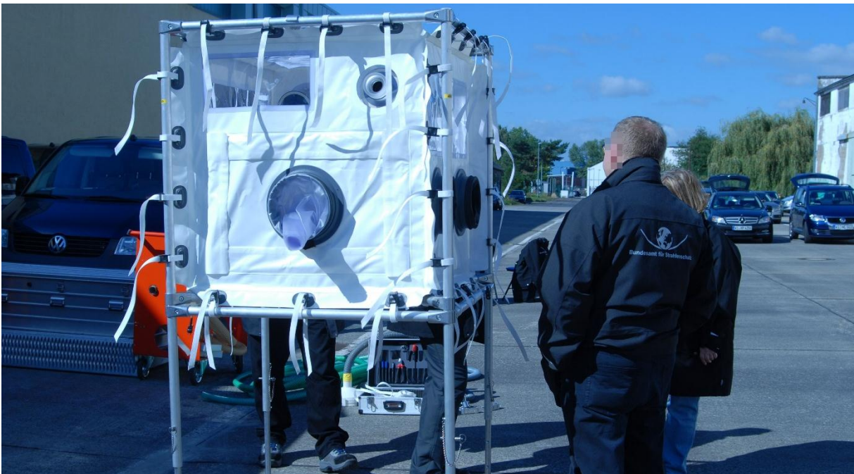
FIG. 3. Glove box for the examination of contaminated evidence from the crime scene. The evidence gets introduced through the round opening visible at the front of the picture. A panel providing multiple connections for electronic equipment can be attached to the other side of the glove box in case a laptop or mobile phone need to be examined and data extracted.
