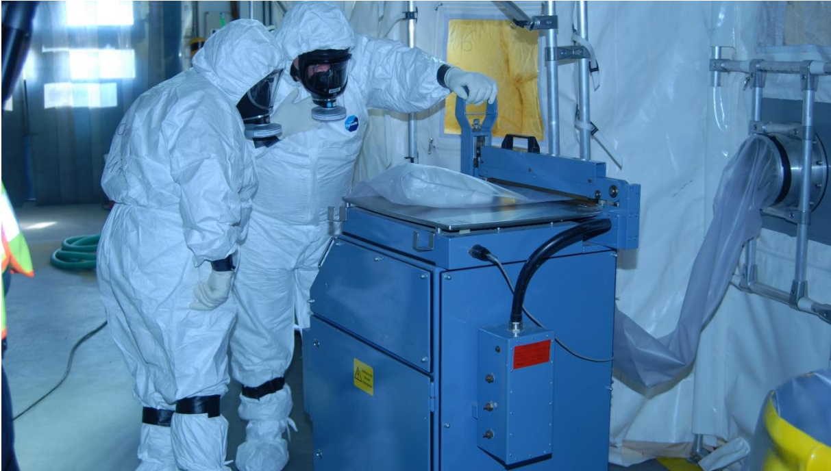
FIG. 2. Airlock with a plastic sleeve in which the contaminated evidence from the crime scene can be heat sealed by means of the heat sealing machine. The heat sealing machine is set up on wheels so it can be transferred to the glove box when necessary.
