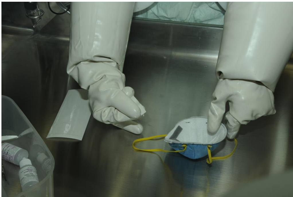
FIG 4. One of the forensic science practitioners trained to operate in the CFAC laboratory demonstrating the ability to perform a taping procedure of an exhibit in one of the glove boxes during a mock casework exercise.
