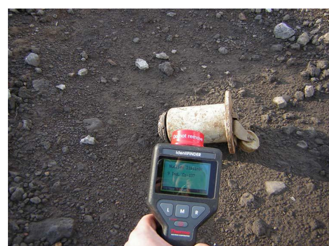
Dose rate measurement in contact with the source
