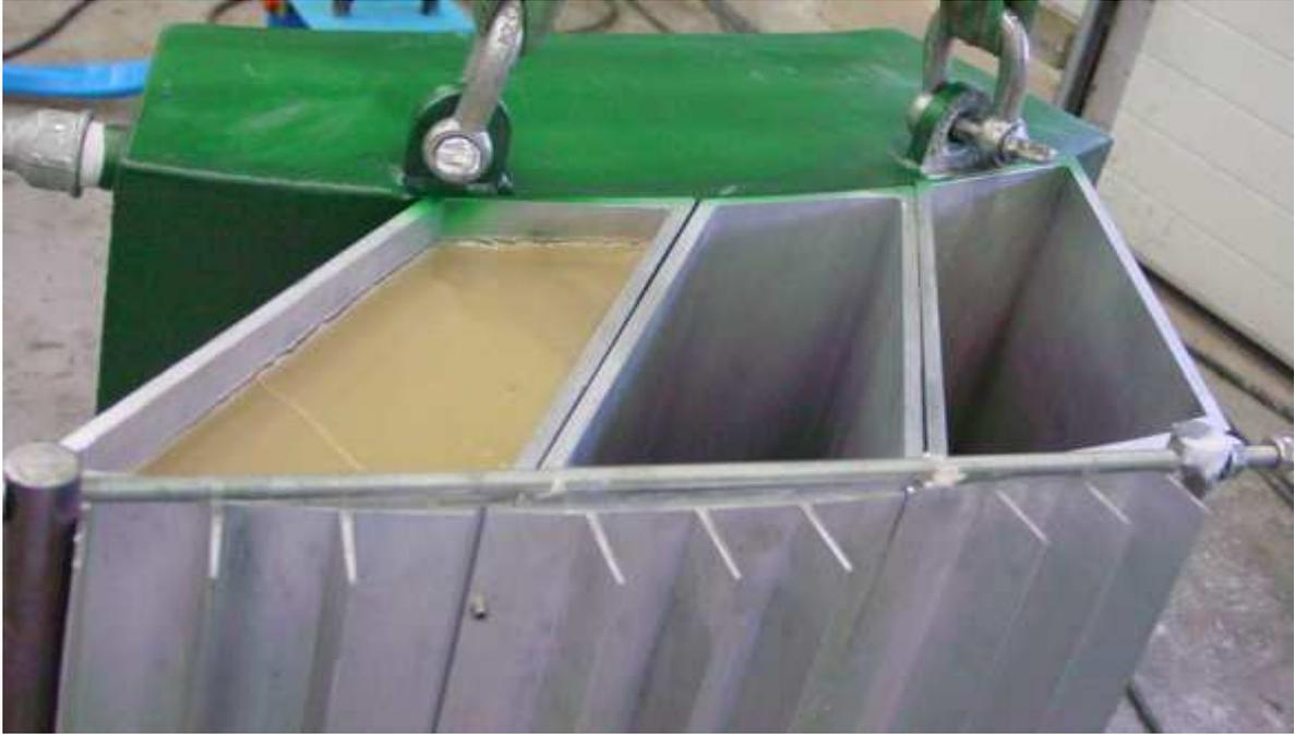
*FIG. 4. Neutron shielding (TN Vyal B<sup>TM</sup>).*
