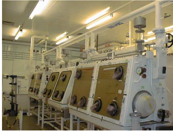
FIG. 5 Example of three interconnecting gloveboxes in laboratory room 2.
