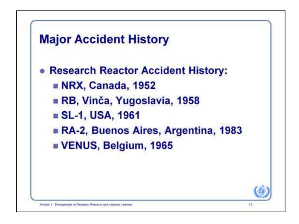
NRX – core destroyed by erroneous control rod withdrawal VINCA – power excursion, exposures of 2.0 to 4.3 Sv SL-1 – power excursion due to design deficiency and operator error, 3 fatalities RA-2 – Criticality due to operator error, 1 fatality VENUS – power excursion due to design deficiency and operator error, 5 Sv to one worker
