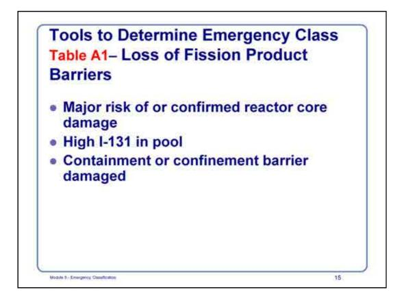
These are the types of events in the category of Loss of Fission Product Barriers. The pool water is treated as a barrier because of the ability to retain many of the fission products if the fuel cladding was damaged. Also, I-131 in the pool confirms that that has occurred.
