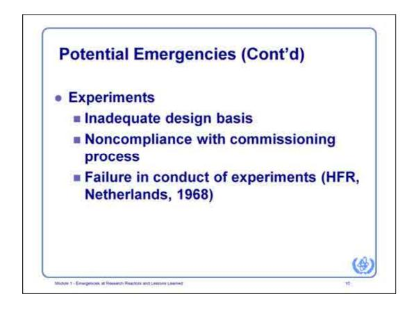
Experiment facilities need the same level of attention to safety as do reactor components. An inadequate design may fail and release radioactive material or cause damage to reactor components.
