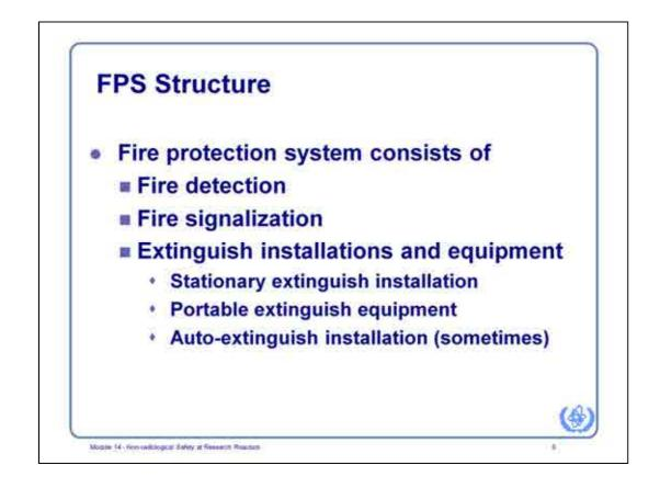
A fire hazard analysis of the reactor facility is carried out to determine the necessary rating of the fire barriers. The analysis results the fire protection system structure then the reactor facility is provided with fire detection and fire fighting systems of the necessary capability.
