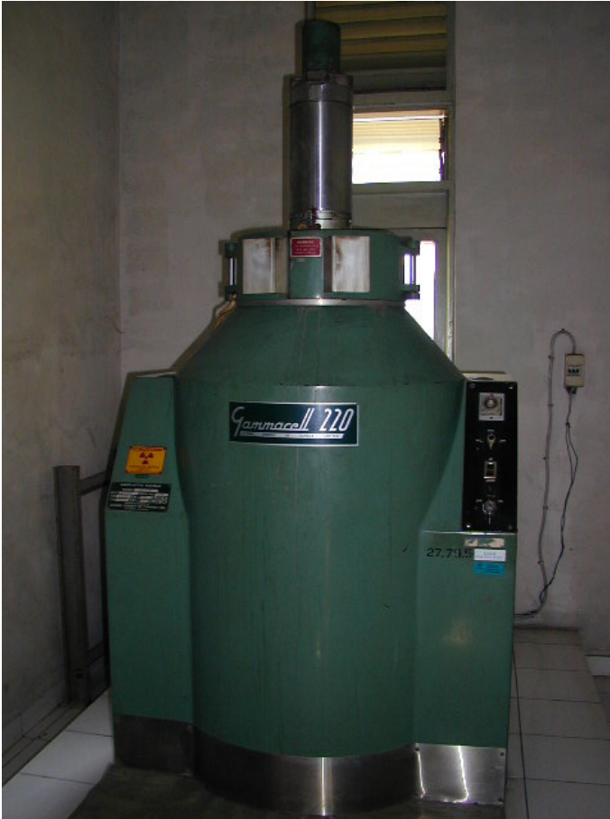
FIG. 4. Model of the gamma cell model 220 (shown to the victims for identification).
