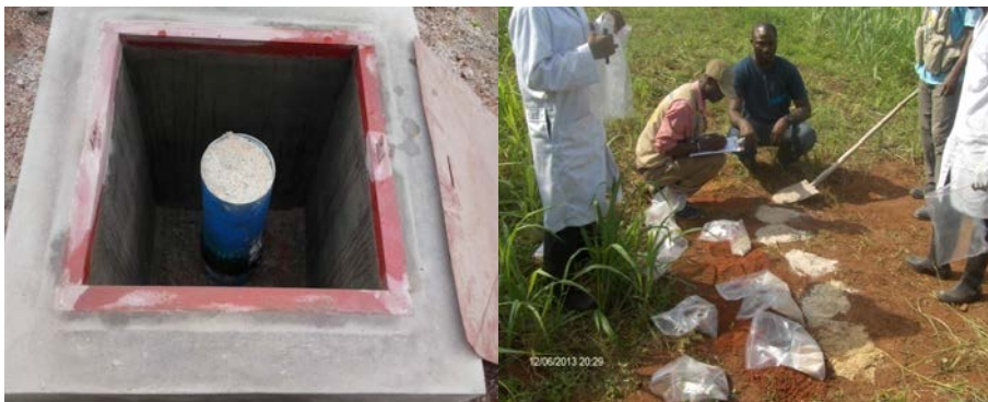
FIG. 6. Drilled investigatory borehole for site characterization and geological logging exercise carried out during the drilling process.
