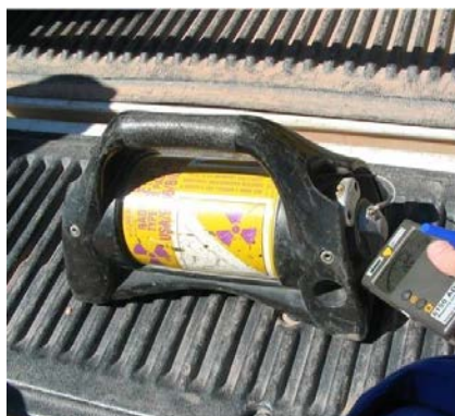
FIG. 4. Shielding used to transport sealed radioactive source in industrial radiography.
