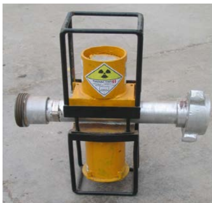
FIG. 2. Nuclear gauge used to measure density of cement and hydraulic fracture.
