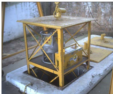
FIG. 3. Shieldings used to transport sealed radioactive sources in well logging applications.
