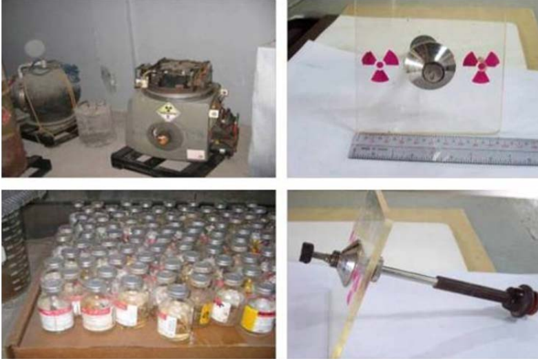
FIG. 4. Radioactive waste from medical applications: teletherapy, brachytherapy, media culture and eye applicators (courtesy of RPS, NSTD and PNRI).
