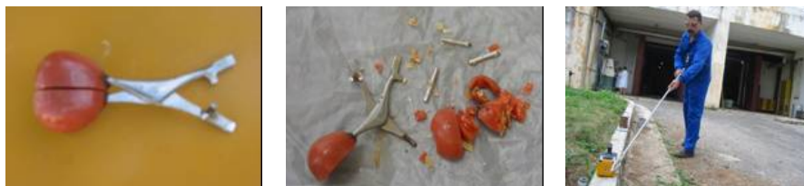
FIG. 3. Recovering sources from applicators: characterizing ^{226}\text{Ra} sources.
