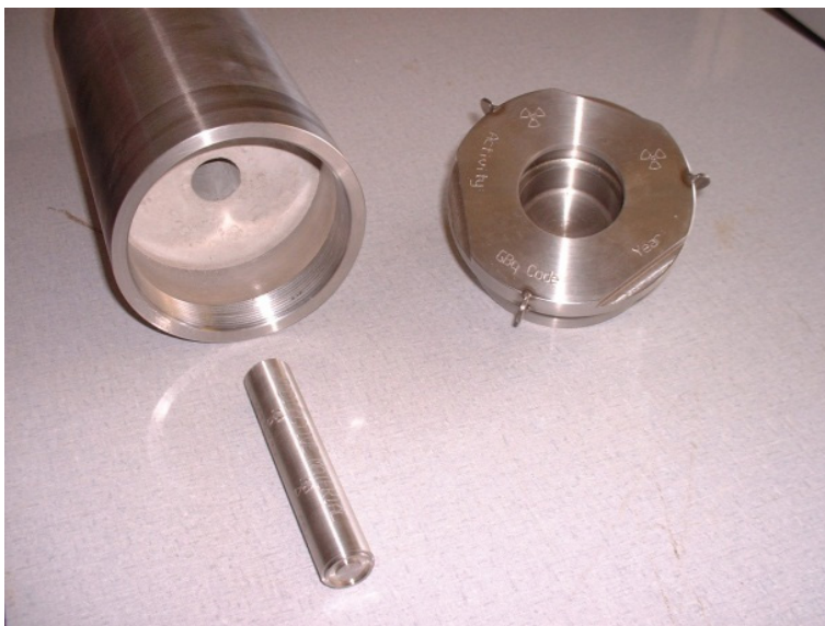
FIG. 5. Source capsule and disposal container.
