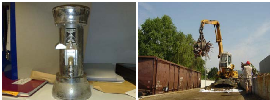
FIG. 4. A source with ^{226}\text{Ra} (i.e. so called 'radium apparatus') identified at the border crossing with Croatia (left) and unloading of scrap from a carriage causing enhanced dose rate in order to find a source or radioactive waste (right).
