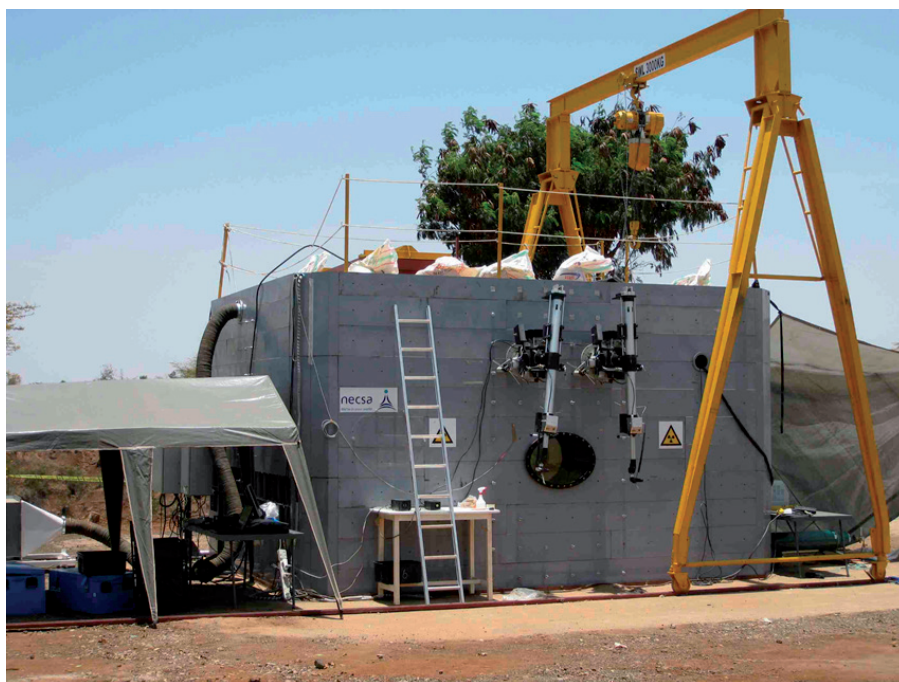
FIG. 6. Mobile hot cell deployed in the United Republic of Tanzania.
