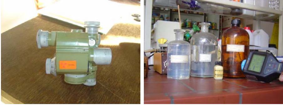
FIG. 5. Abandoned sources found during the inspections of the SNSA: (left) ^3\text{H} source with an activity of 129 GBq, installed in military equipment abandoned in a storage facility; (right) radioactive waste with ^{232}\text{Th} , including liquids stored in a research and educational laboratory at one of the faculties.
