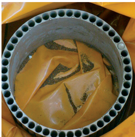
FIG. 5. Dismantled gamma cell at Mayapuri scrap shop (source cage and source).
