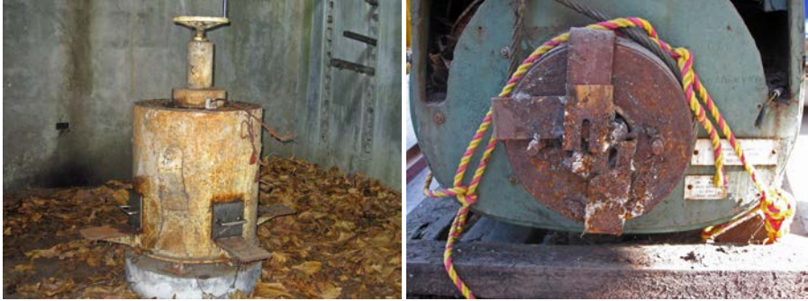
FIG. 1. Badly corroded, high activity source containing devices from an operation in 2013.
