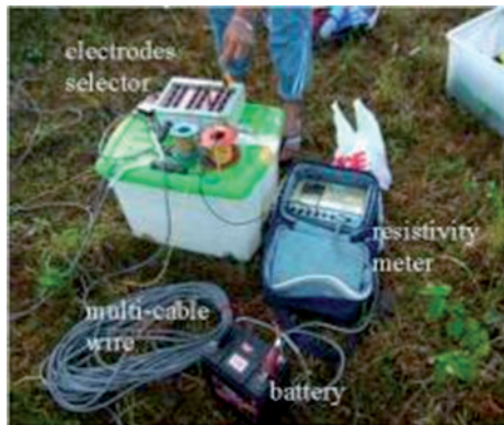
FIG. 11. Sets of resistivity equipment used.
