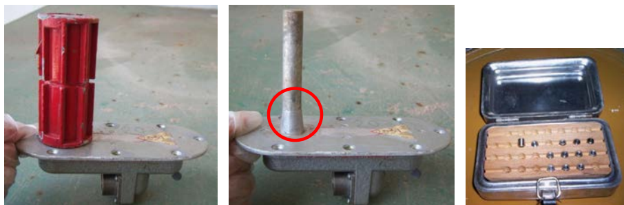
FIG. 2. Ice detectors used in aircraft and the contained ^{90}\text{Sr} radioactive sources.
