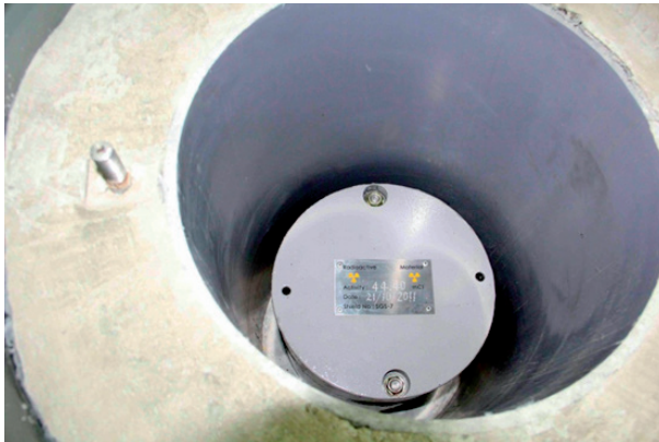
FIG. 5. Lead shield containing capsules placed in concrete lined drum.
