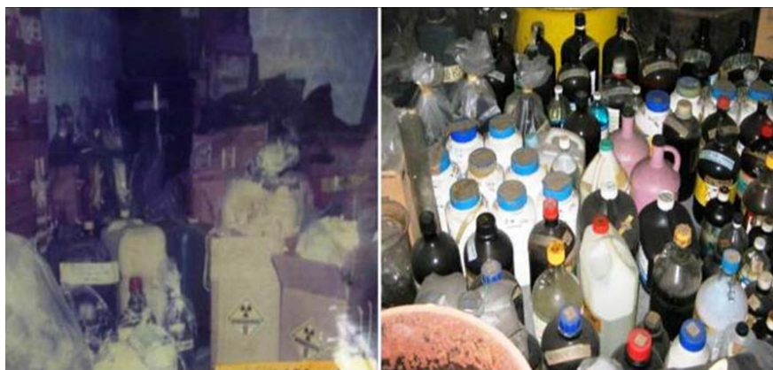
FIG. 3. Radioactive waste in research and educational institutions: std/check/reference sources, rugs, paper towels and vials (courtesy of RPS, NSTD and PNRI).
