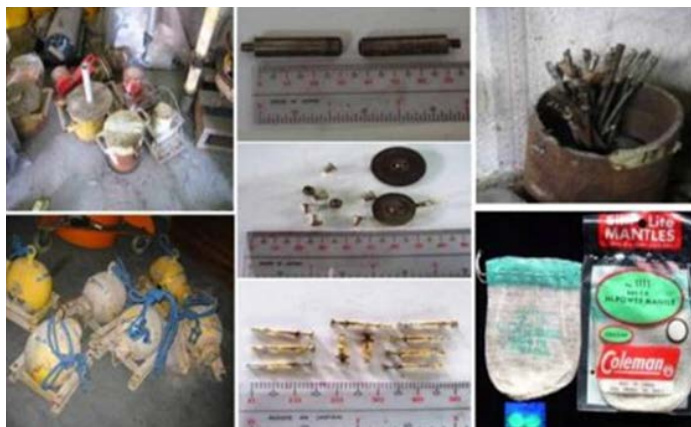
FIG. 2. Radioactive waste in industry: gauges, static eliminators, radiographic sources, smoke detectors and gas mantles (courtesy of RPS, NSTD and PNRI).
