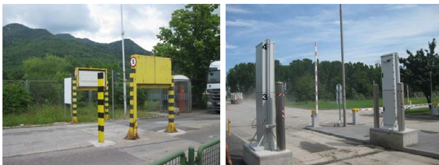
FIG. 1. Portal monitor systems in order to identify uncontrolled sources at an entrance of a factory (left) and at a scrap yard (right).
