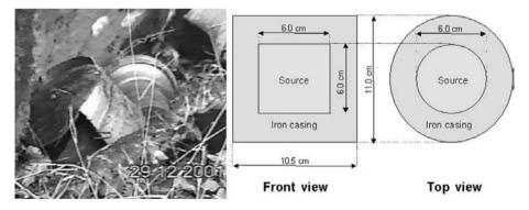
FIG. 79. Radioactive sources in the recovery location (left) and front and top view of the radioactive sources (right) (reproduced from Ref. [6] with permission courtesy of Oxford University Press).
