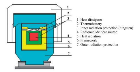
FIG. 2. Radioisotope thermoelectric generator, Beta M type.
