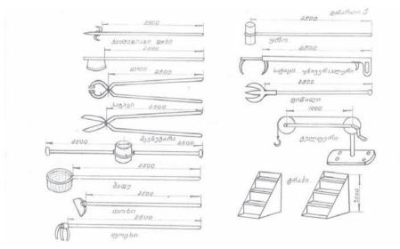
FIG. 5. Sketch of the manipulating devices used in the recovery operation.
