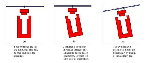
FIG. 12. Different relative orientations of the container and its lid.
