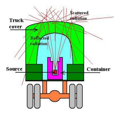
FIG. 13. The open container with the radioactive source on the vehicle.
