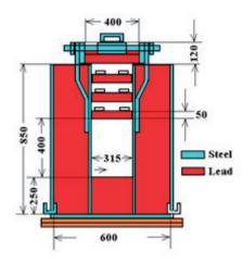
FIG. 4. Shielding container for the radioactive sources.
