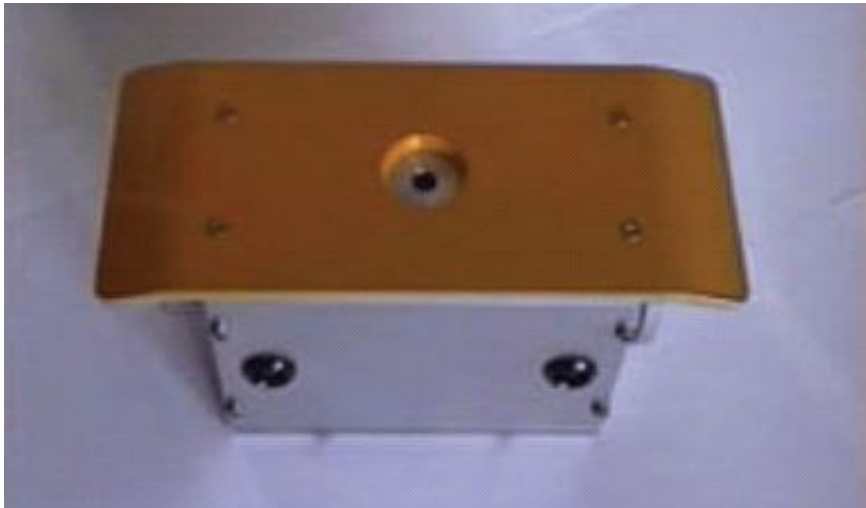
FIG. 32. A detail of a beta gauge source holder.
