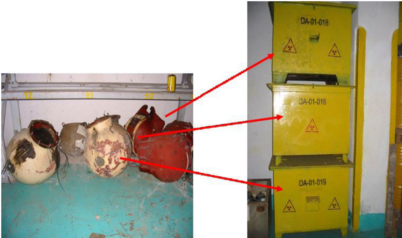
FIG. 91. Teletherapy units before and after being conditioned inside metallic boxes.
