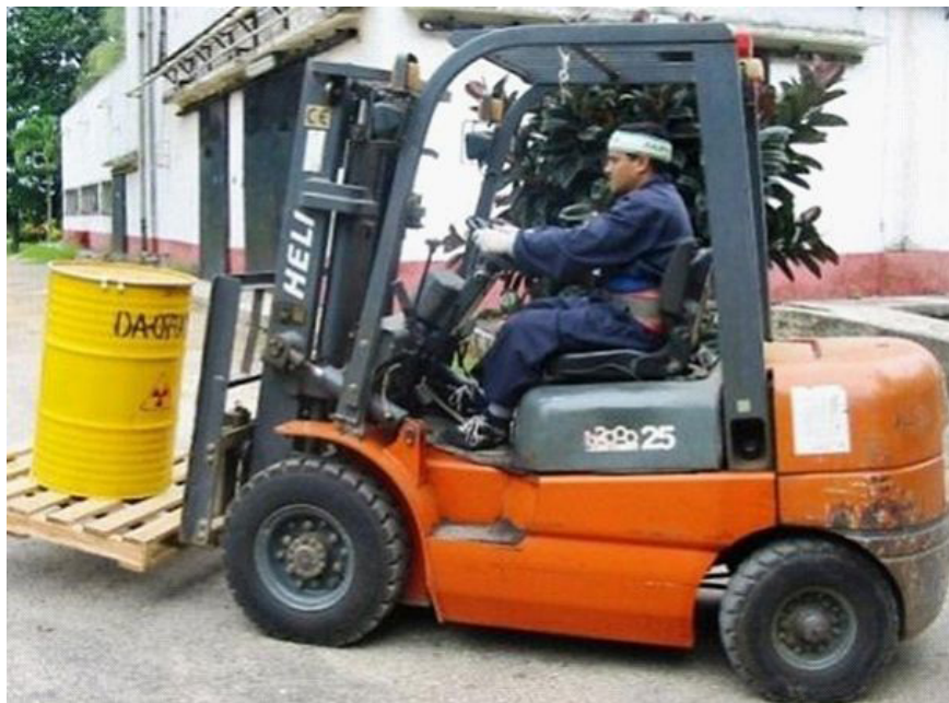
FIG. 57. Handling a 200 L waste drum with a forklift truck.
