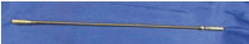
FIG. 21. A typical modern gamma radiography source/pigtail assembly.
