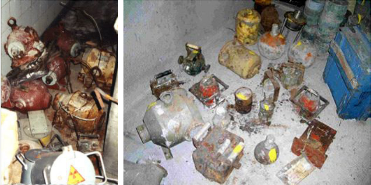
FIG. 73. Inadequate storage of DSRs.
