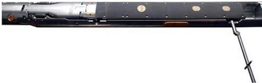
FIG. 31. Atlas Densilog, which uses a vitrified ^{137}\text{Cs} source for wireline density measurements. The rod extending downward is a source handling device. The light coloured circles are windows for the source and detectors.
