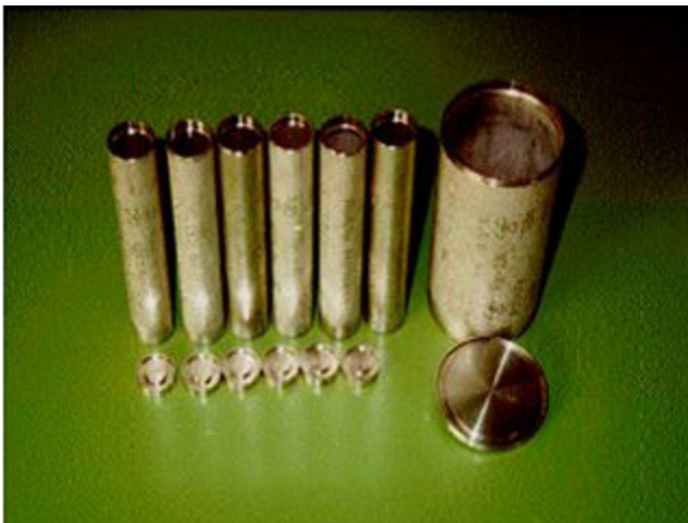
FIG. 83. Typical stainless steel capsules.
