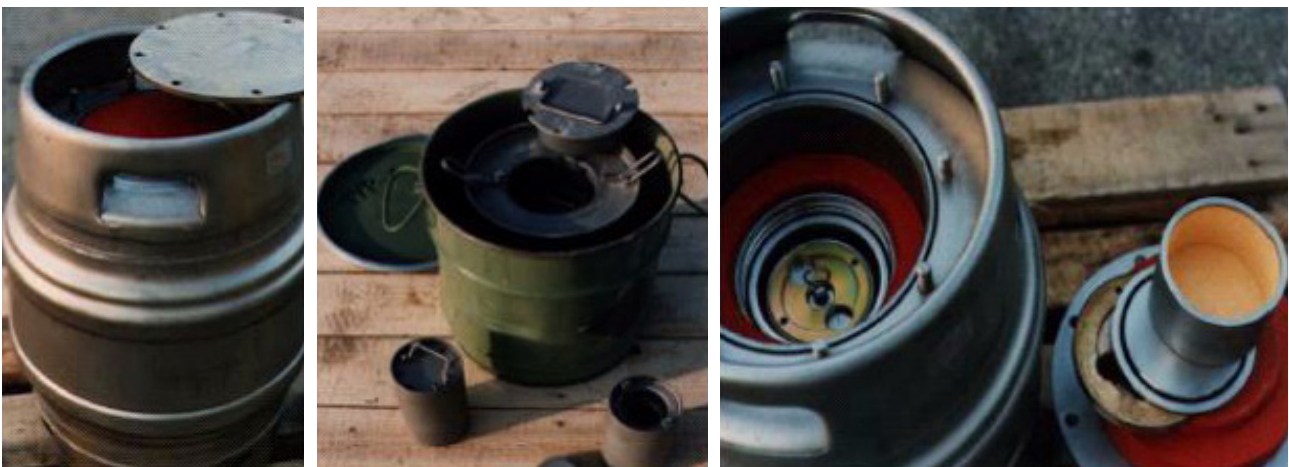
FIG. 98. For small sources, depending on the source size, geometry and activity, a special container should be used for transport.
