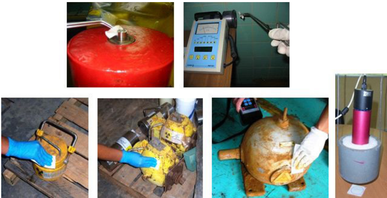
FIG. 45. Smear tests for contamination control.
