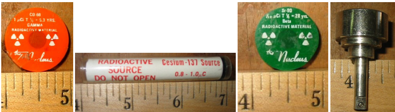
FIG. 25. Examples of low activity ^{60}\text{Co} , ^{137}\text{Cs} , ^{90}\text{Sr} and ^{226}\text{Ra} calibration sources.
