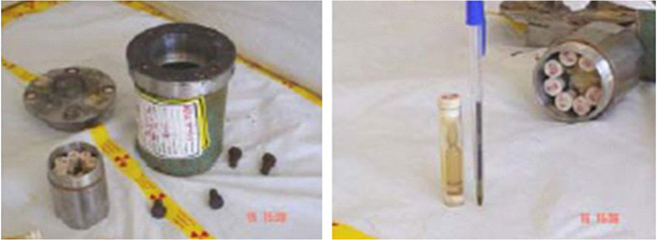
FIG. 4. ^{226}\text{Ra} liquid sources in glass vials.
