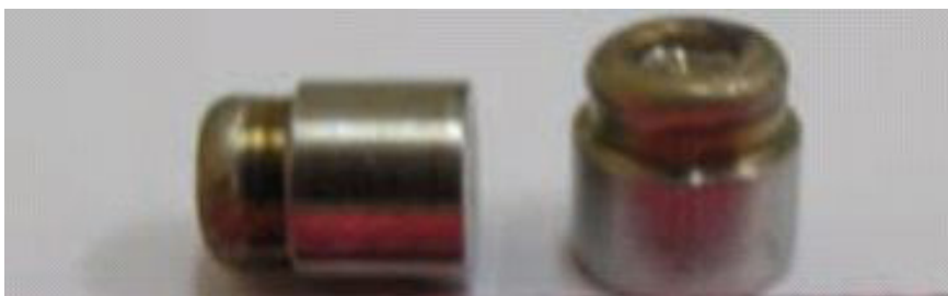
FIG. 22. A typical gamma radiography inner source capsule prior to encapsulation in the pigtail.
