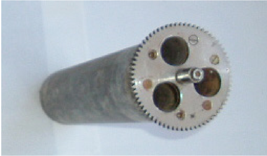
FIG. 81. An inner rotating part of a B(U) type loading/unloading container.
