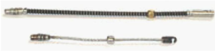
FIG. 20. Typical old gamma radiography source/pigtail assemblies.
