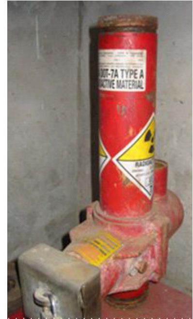
FIG. 97. Examples of an original radioactive source holder used as a transport package.
