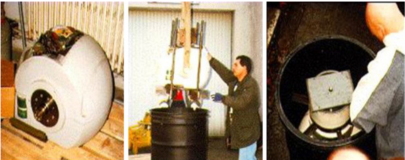
FIG. 90. A teletherapy head before being conditioned inside a metal drum.
