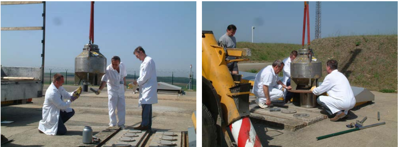
FIG. 75. Preparation and loading of ^{60}\text{Co} DSRs in a well type storage unit.
