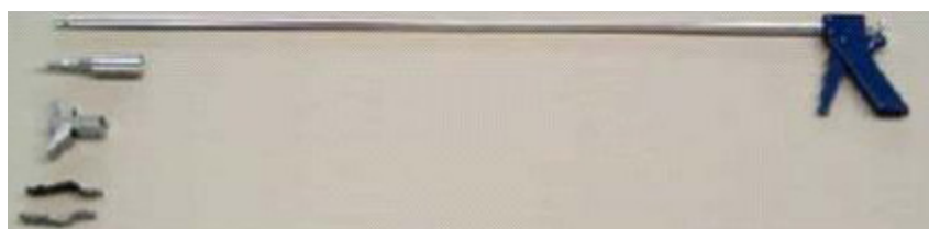
FIG. 49. Long tongs and manipulation of source with them.
