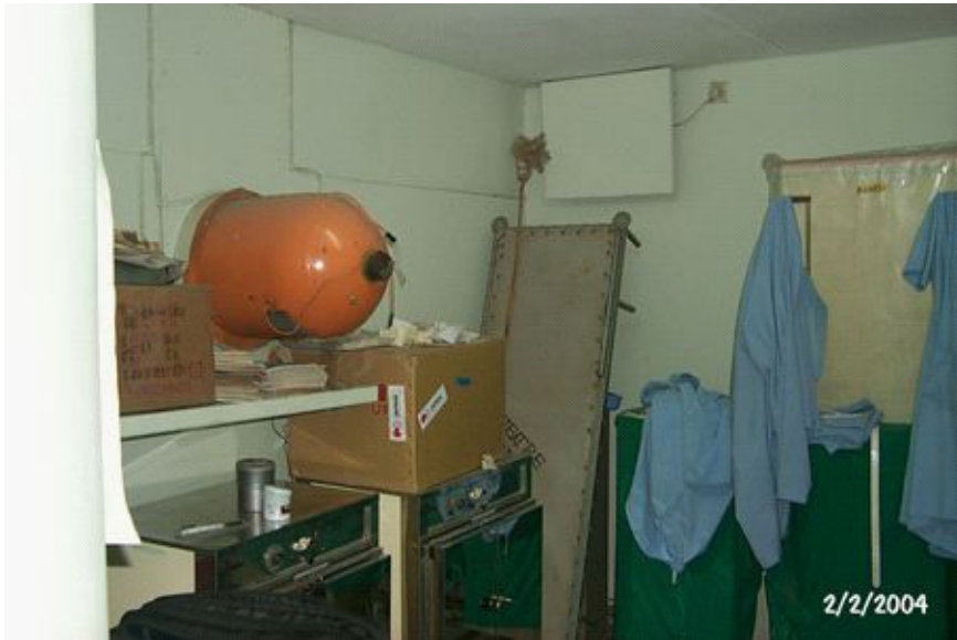
FIG. 68. The drawer containing a ^{60}\text{Co} source was not removed from the teletherapy machine.
