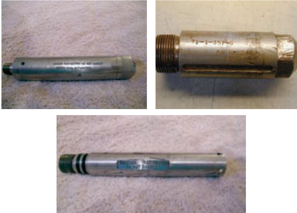
FIG. 30. Typical ^{241}\text{Am} -Be neutron oil well logging sources.
