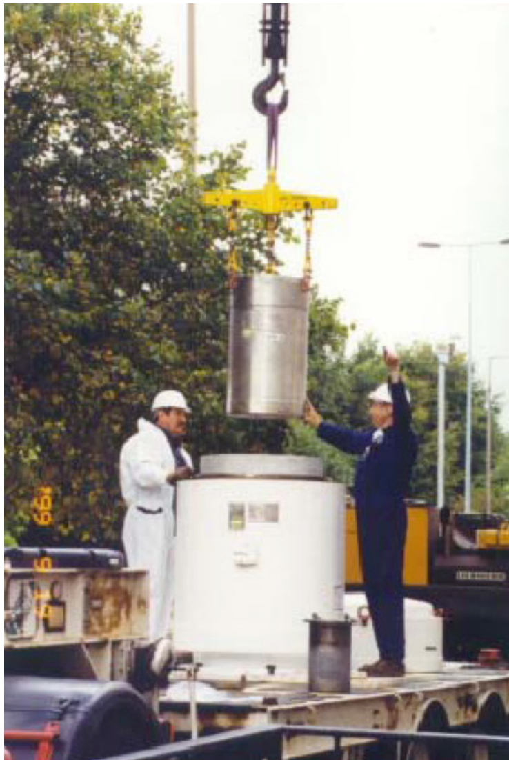
FIG. 104. ^{137}\text{Cs} shielded inner container being loaded into a Type B package, following removal of ^{137}\text{Cs} sources from a research irradiator.
