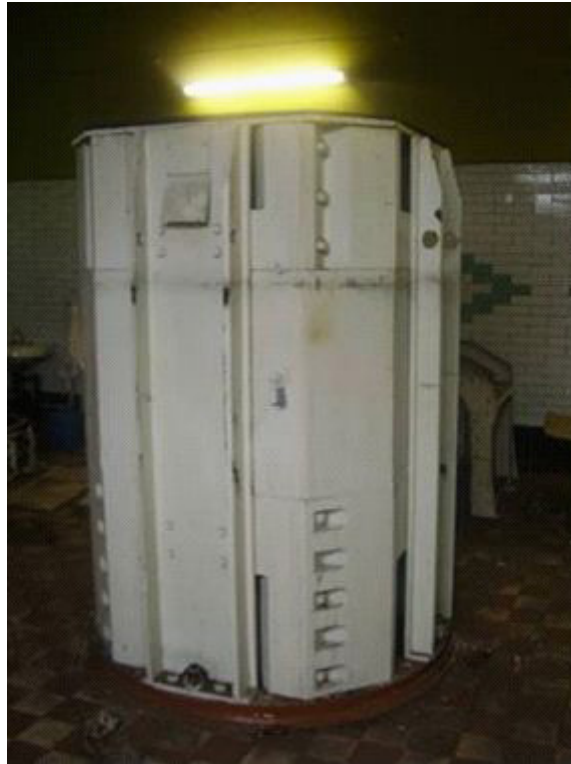
FIG. 106. An irradiator loaded with ^{137}\text{Cs} DSRs ready for transport to the disposal facility.
