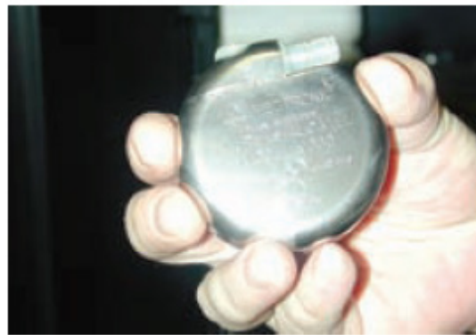
FIG. 6. An RTG powered heart pacemaker.
