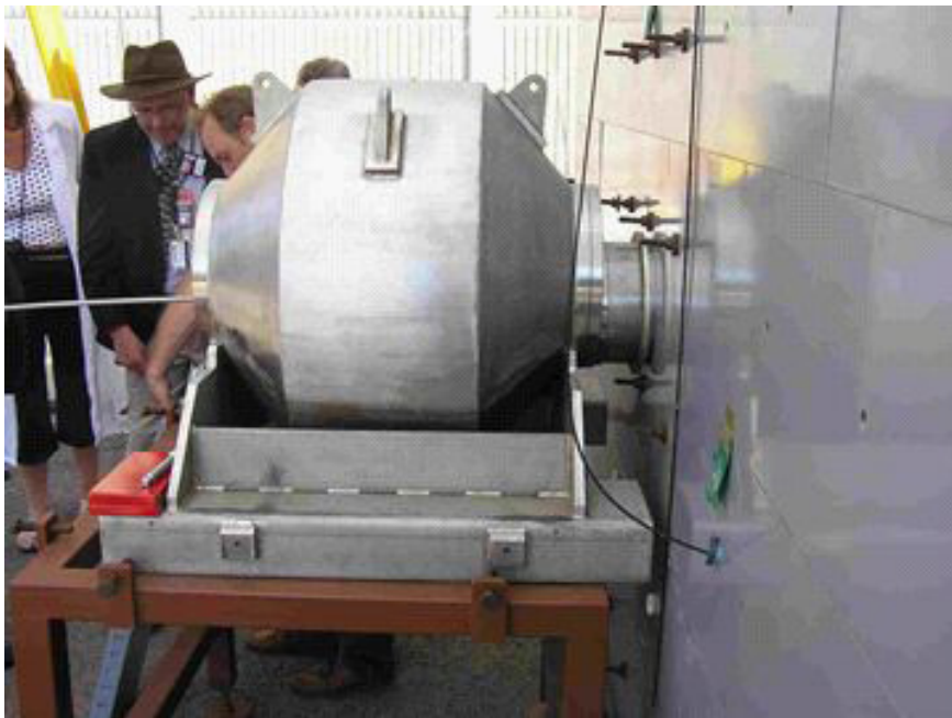
FIG. 94. The long term storage shield fully attached to the transfer port on the IAEA Mobile Hot Cell Facility.
