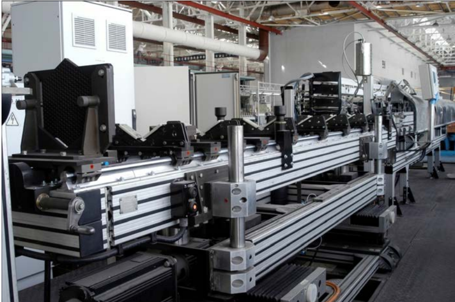
FIG. 28. Assembly hoist system (courtesy of TVEL).
