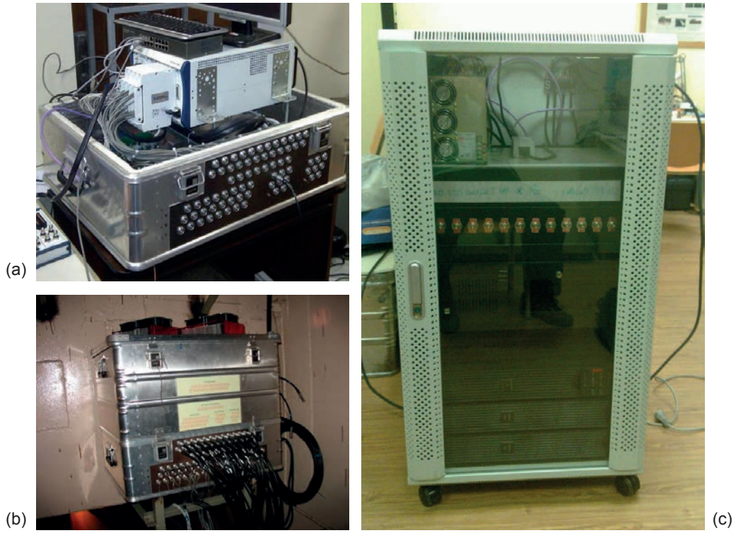
FIG. 38. Hardware of the monitoring system. (a) and (b) Data acquisition and processing block; (c) Data storage and transfer block.
