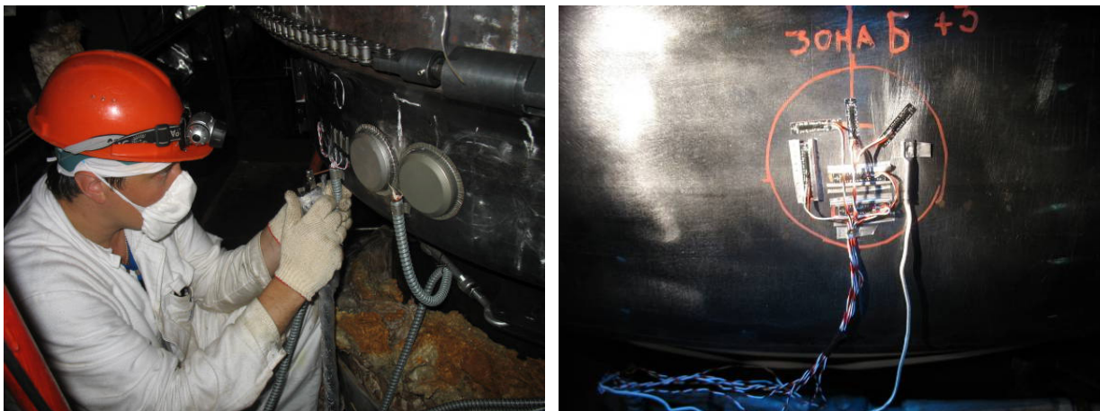
FIG. 42. Mounting of the strain gauges and thermocouples.
