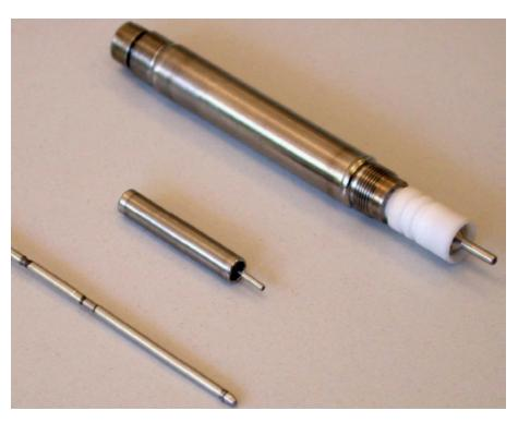
FIG. 12.1. Examples of fission chambers with different diameters for the measurement of neutron flux (courtesy of the French Alternative Energies and Atomic Energy Commission).
