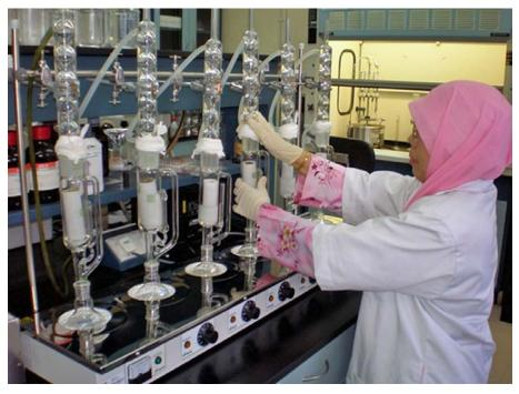
FIG. 3.1. Sample preparation for instrumental neutron activation analysis (courtesy of the Malaysian Nuclear Agency).
