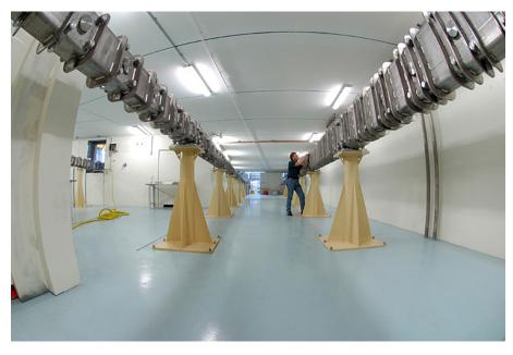
FIG. 9.5. Thermal neutron beam guide tubes at the 20 MW OPAL research reactor (courtesy of ANSTO).
