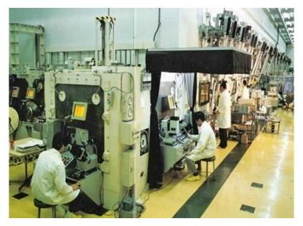
FIG. 12.3. Hot laboratory for material post-irradiation examination at the Japan Materials Testing Reactor (courtesy of the Japan Atomic Energy Agency).
