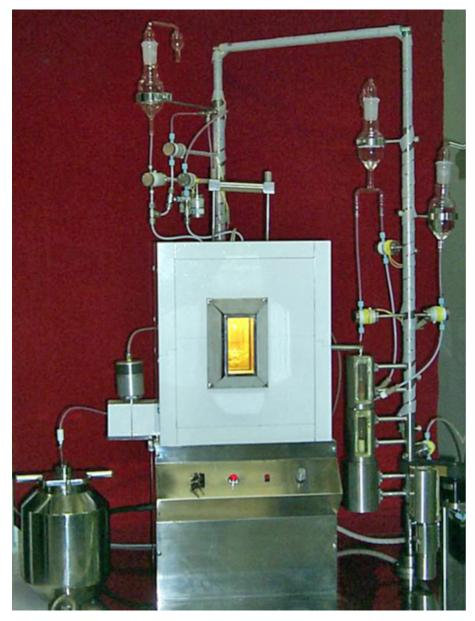
FIG. 5.5. Technetium-99m solvent extraction unit (courtesy of the Korea Atomic Energy Research Institute).
