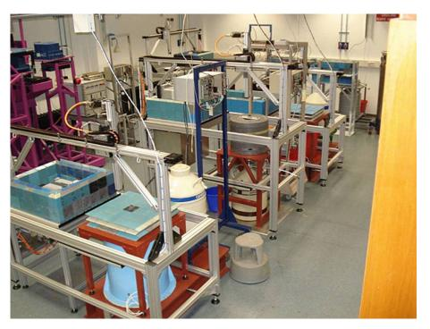
FIG. 3.5. Automatic sample changers in the laboratory for instrumental neutron activation analysis (courtesy of Delft University of Technology).
