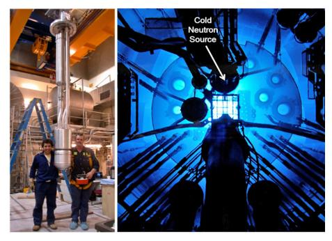
FIG. 9.3. The 20 L cold neutron source before (left) and after (right) being positioned in the OPAL research reactor (courtesy of ANSTO).
