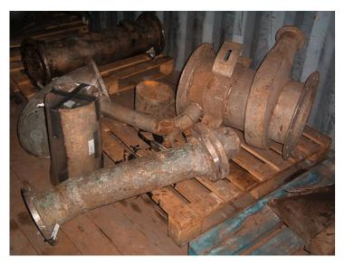
FIG. 4. Objects contaminated with NORM.
