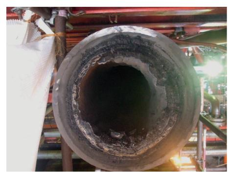
FIG.1. NORM contaminated pipe.
