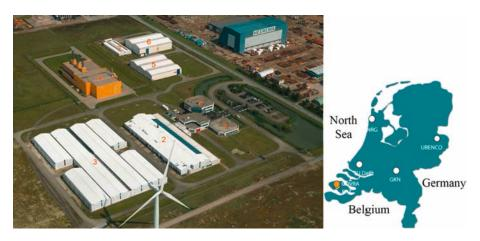
FIG 1. The COVRA site. (1) Office building and exhibition centre; (2) Building for the treatment of low and medium level waste (AVG); (3) Storage building for conditioned low and medium level waste (LOG); (4) Storage building for high level waste (HABOG); (5) Storage building for low level material from the enrichment industry (VOG); (6) Storage building for low level NORM waste from the ore processing industry (COG); (7) Storage building for scrap material (SOG).
