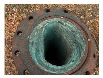
FIG. 3. Uranium process residues in scrap pipework.
