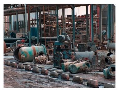
FIG. 2. NORM contaminated items in storage prior to cleaning or disposal.
