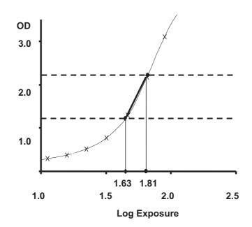
FIG. 47. Sensitometric data used for estimation of film gradient.
