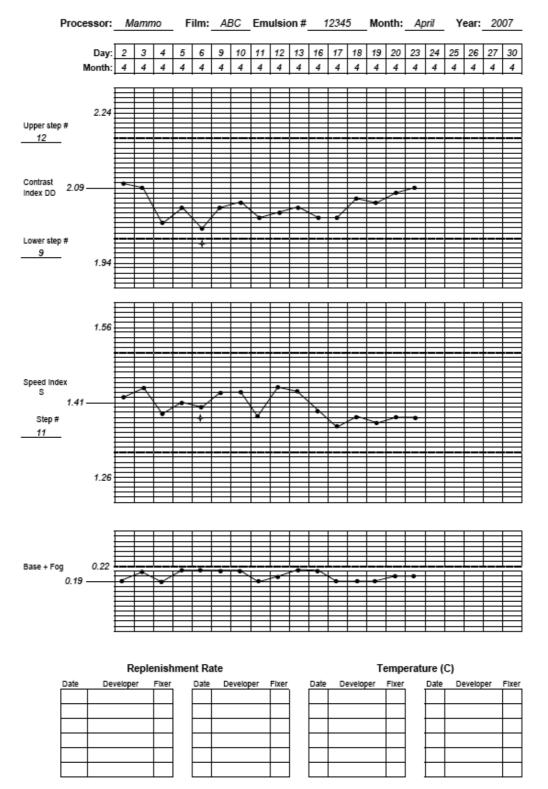
FIG. 42. Sample film processor QC chart. Note that the measurement on 6 April 2007 was repeated because the initial value of DD was outside the action level.
