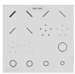
FIG. 46. Schematic representation of the ACR phantom – the chest wall edge is at the bottom.
