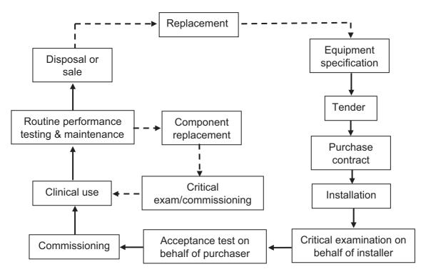
FIG. 1. Life cycle of a piece of equipment.
