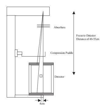
FIG. 45. Set-up for HVL measurement.
