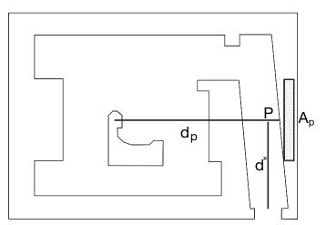
FIG. 5. Schematic diagram showing the scatter path for the primary radiation beam to the maze entrance (gantry rotation axis parallel to the maze axis).
