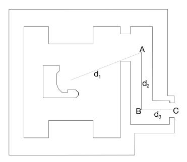
FIG. 9. Room with two bends in the maze showing distances used to determine the capture gamma dose.
