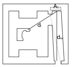
FIG. 6. Schematic diagram showing the path of scattered head leakage to the maze entrance.
