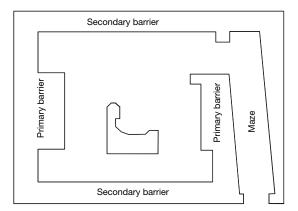
FIG. 2. Typical room layout where the gantry rotation axis is parallel to the maze axis.
