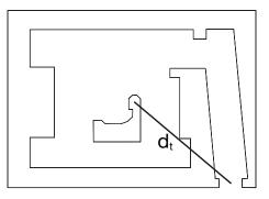
FIG. 7. Schematic diagram showing the path of head leakage radiation transmitted through the maze wall to maze entrance.
