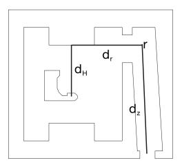
FIG. 4. Schematic diagram showing the scatter path for the primary radiation beam to the maze entrance (gantry rotation axis perpendicular to the maze axis).
