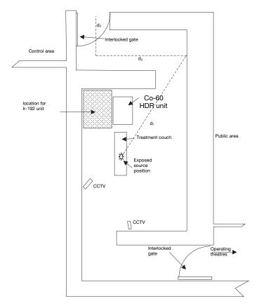
FIG. 18. Plan of an HDR <sup>60</sup>Co treatment room.
