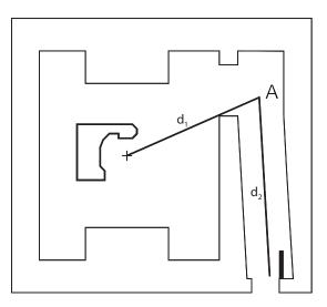
FIG. 8. A typical accelerator room with a maze, showing the distances used to determine the capture gamma dose.
