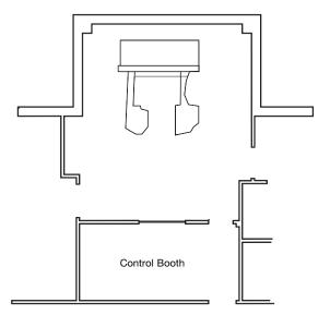
FIG. 15. A typical room for a simulator with fluoroscopy capability.
