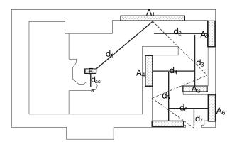
FIG. 3. Schematic diagram to show the scatter paths to the maze entrance.
