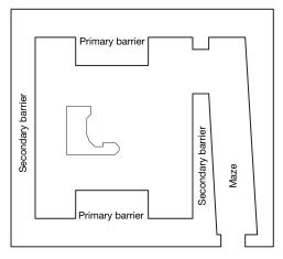
FIG. 1. Typical room layout where the gantry rotation axis is perpendicular to the maze axis.
