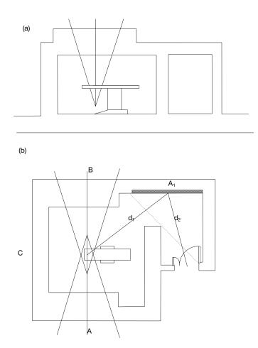
FIG. 10. Schematic layout of a <sup>60</sup>Co room showing (a) elevation and (b) plan.
