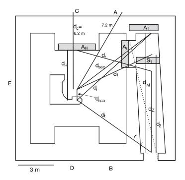
FIG. 12. Schematic layout of an 18 MV facility.
