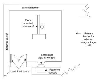
FIG. 17. Example layout of an orthovoltage room.
