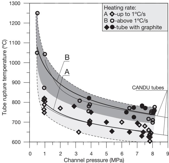
FIG. 6. Pressure tube rupture temperature as a function of internal pressure.
