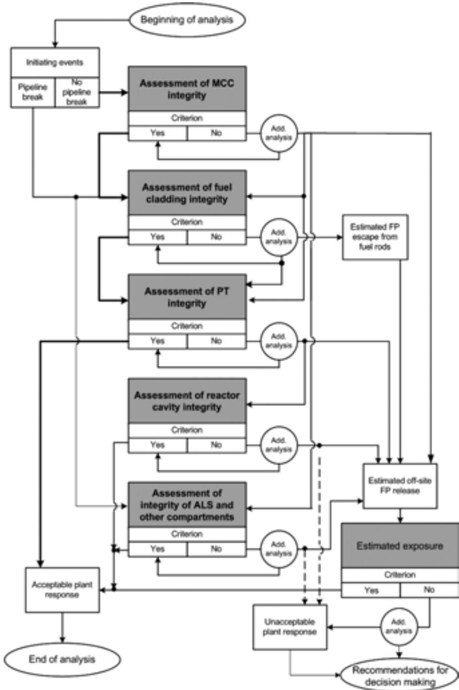
FIG. 2. Flow chart for accident analysis (FP, fission power; PT, pressure tube).
