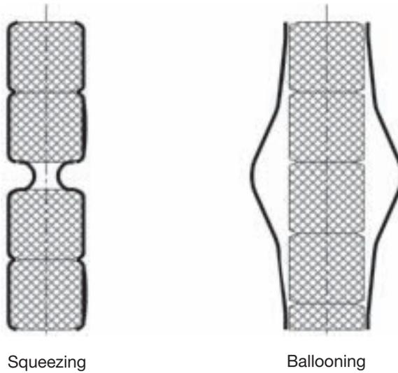
FIG. 3. Cladding deformation modes.
