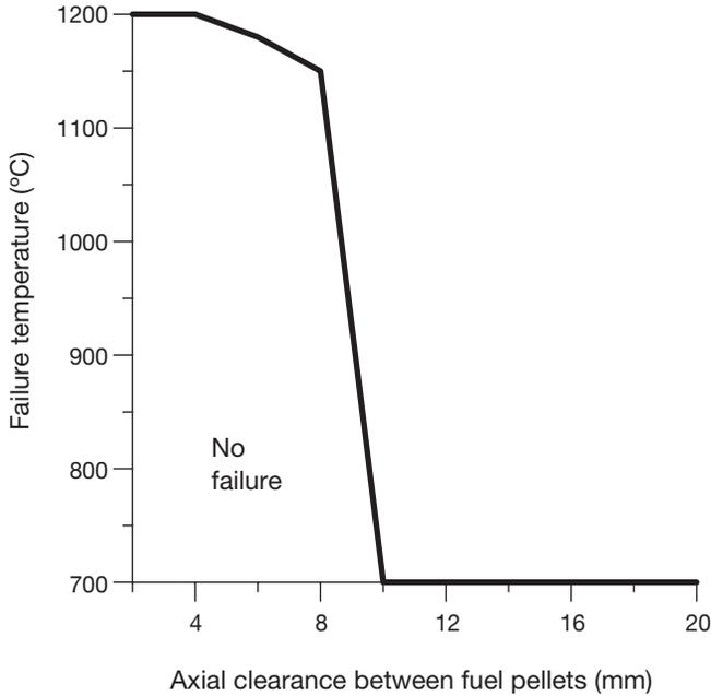
FIG. 4. Cladding failure under squeezing.
