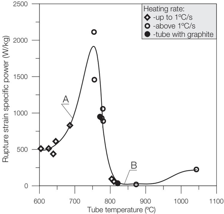
FIG. 7. Specific rupture strain power as a function of tube temperature: A, first polynomial in Table 6,  $T \leq 780^\circ\text{C}$ ; B, second polynomial,  $T > 780^\circ\text{C}$ .
