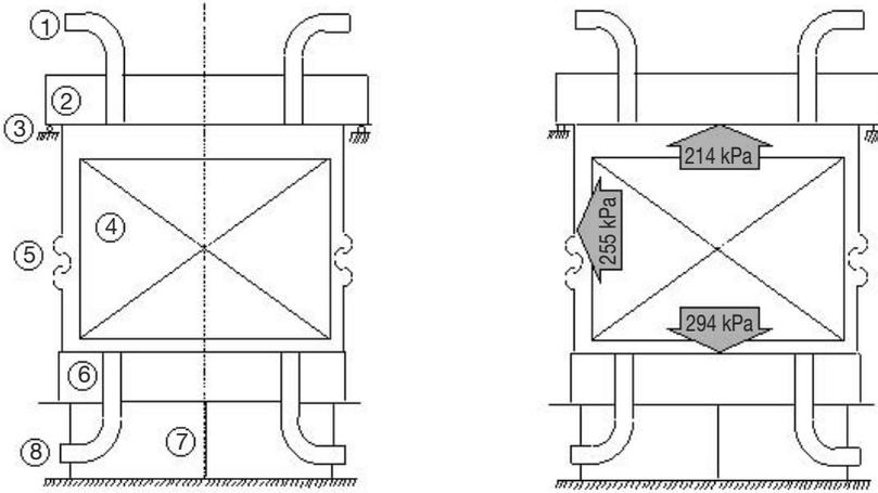
FIG. 9. Reactor cavity components and ultimate pressures: 1, upper steam dump pipes; 2, top plate; 3, roller support; 4, core; 5, barrel; 6, bottom plate; 7, support; 8, lower steam discharge pipes.
