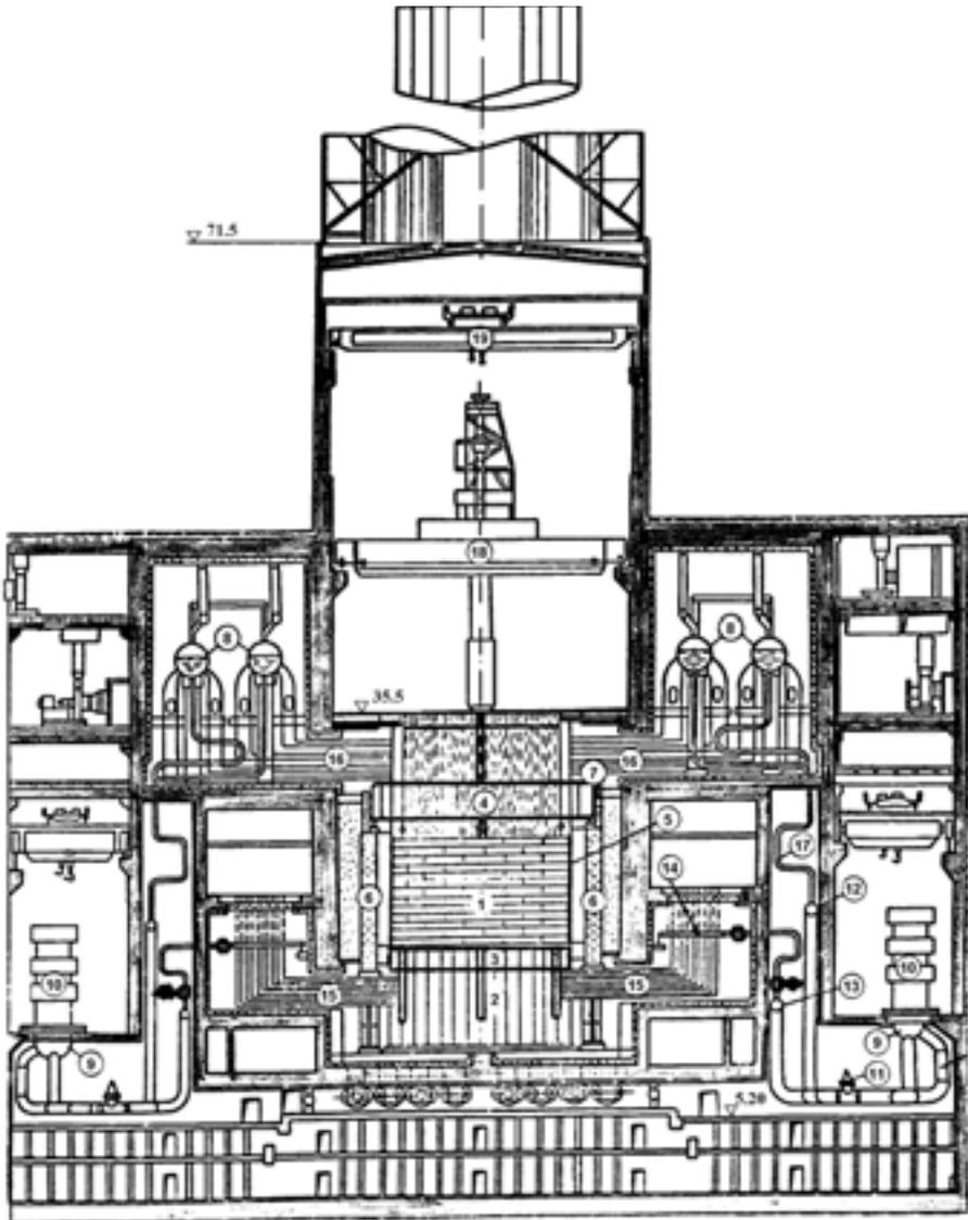
FIG. 1. Schematic diagram of an RBMK reactor: 1, graphite stack; 2, structure S; 3, structure OR; 4, structure E; 5, structure KZh; 6, structure L; 7, structure D; 8, drum separator; 9, MCP casing; 10, MCP motor; 11, pressure gate valve; 12, suction header; 13, pressure header; 14, distribution group header; 15, water lines; 16, steam and water lines; 17, downcomers; 18, refuelling machine; 19, central hall crane.
