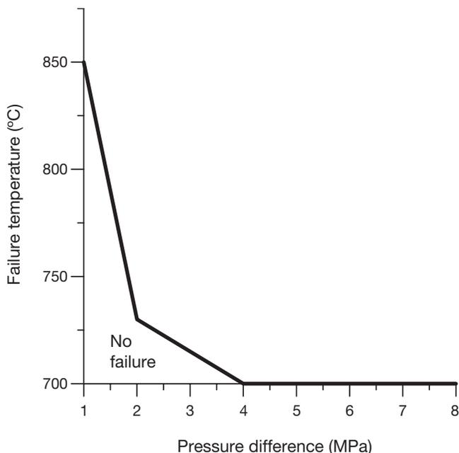
FIG. 5. Cladding failure under ballooning.
