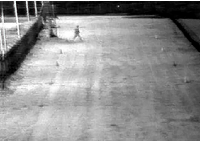
FIG. 15. Scene with a low light-to-dark ratio of approximately 4:1. (Courtesy of Sandia National Laboratories).
