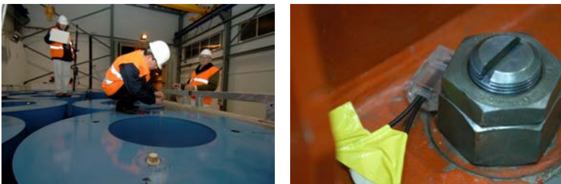
FIG. 9. Examples of seals that are used by the IAEA to maintain continuity of knowledge.
