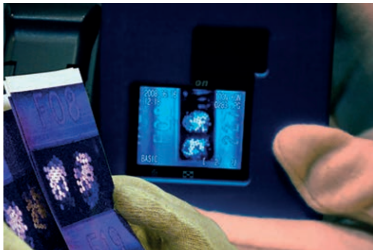
FIG. 21. A fibre optic seal being interrogated.
