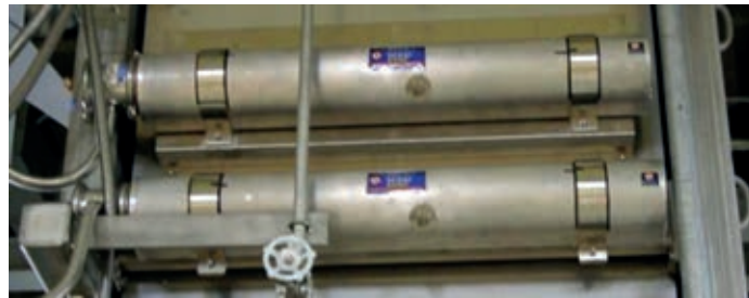
FIG. 18. Plutonium inventory measurement system 3 He neutron sensor enclosures on glove boxes.
