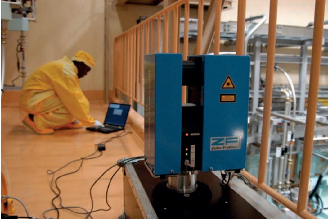
FIG. 12. IAEA design verification using a 3D laser rangefinder.
