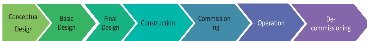
FIG. II-1. Facility life cycle stages.
