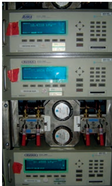
FIG. 14. Solution measurement and monitoring system electromanometer.
