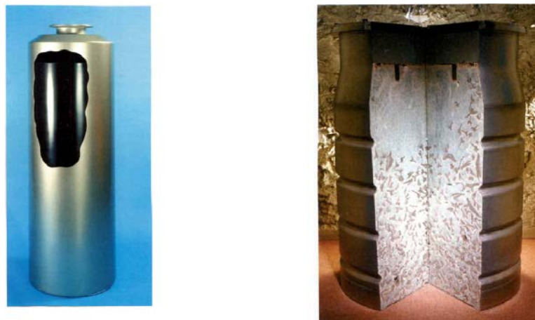
FIG. 4. Solid radioactive waste forms. Left: Cutaway showing simulated vitrified HLW in a stainless steel production container. The container is 1.3 m high and holds about 150 L of glass. Right: Cutaway showing simulated cement encapsulated intermediate level waste from reprocessing of spent fuel (metallic fuel cladding waste) in a 500 L stainless steel drum. Several such drums might be placed in a steel or concrete box, surrounded by an additional cement matrix, for disposal (courtesy of BNFL).
