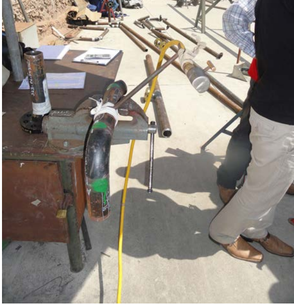
FIG. 5. Set-up for the test of the 2 in (5.1 cm) pipes, area A.
