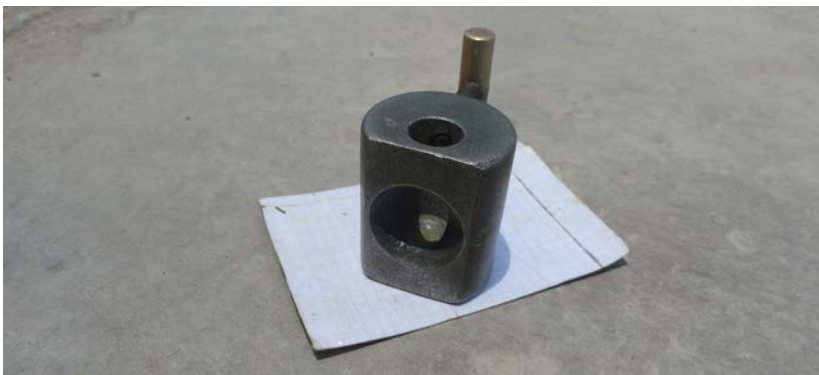
FIG. 2. Collimator used during radiography of the pipes.
