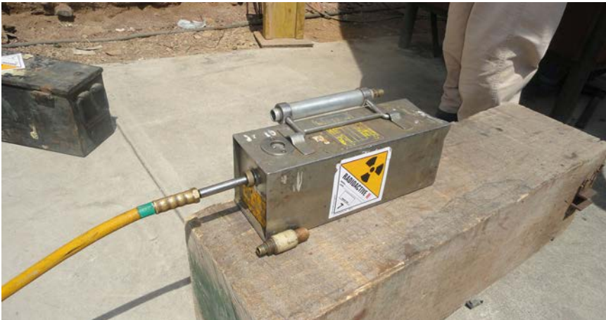
FIG. 1. The radiography camera involved in the accident.
