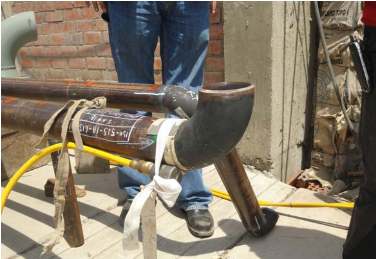
FIG. 6. Set-up for the test of the 3 and 4 in (7.6 and 10.2 cm) pipes, area B.
