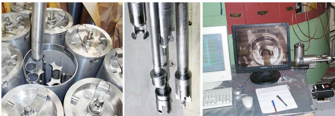
FIG. 1. ‘Untight’ canisters and equipment for repackaging of the damaged Vinca SNF.
