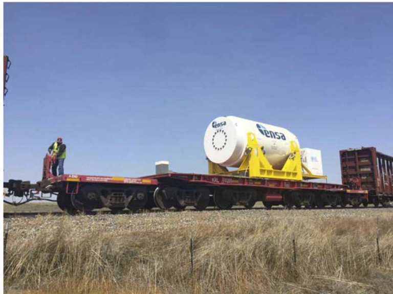
FIG. 8. Kasgro 12-axle railcar used for rail transport.
