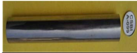
FIG. 1. Typical Vitrified Cs Glass Pencil.
