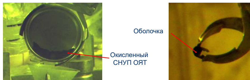
FIG 2. Oxidized MNIT SNF.
