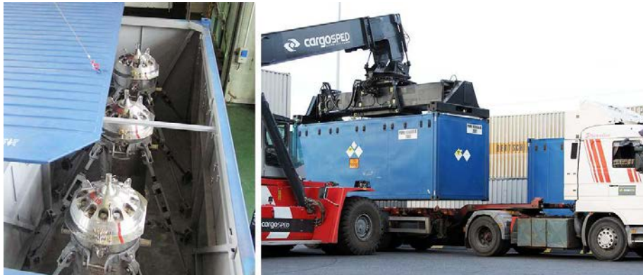
FIG. 4. Overpack for multimodal transportation of TUK-19 casks.
