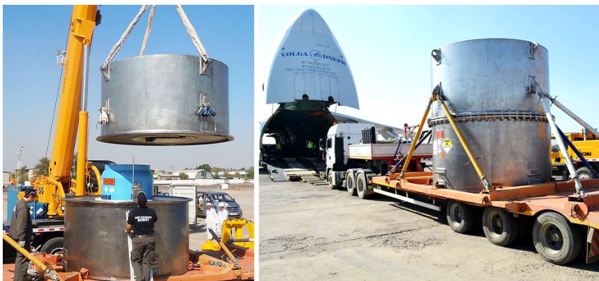
FIG. 5. TUK-145/C for air transport of the spent fuel.
