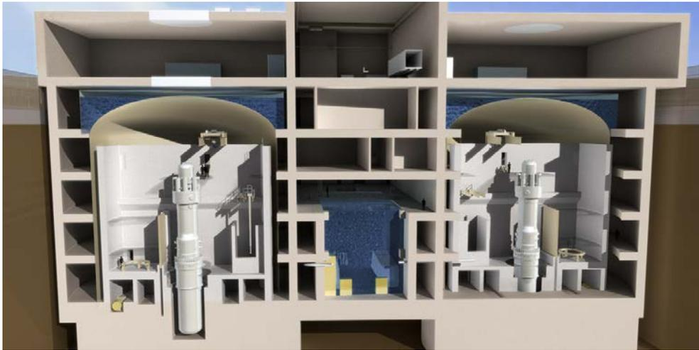
FIG. A-13. A two-unit SMR nuclear power plant (courtesy of Babcock and Wilcox Nuclear Energy).
