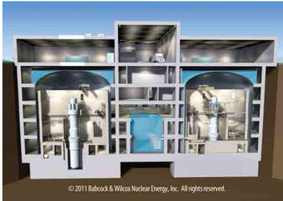
FIG. 188. Babcock and Wilcox mPower small modular reactor containment (courtesy of Babcock & Wilcox).
