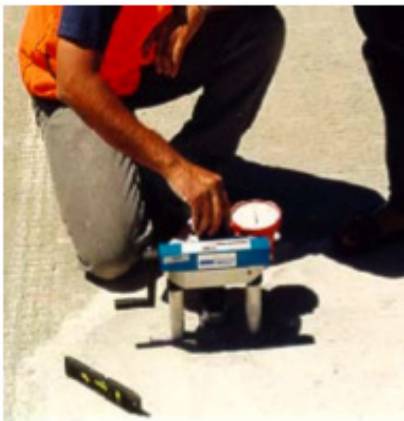
FIG. 94. Pull-off test: equipment (left); schematic of test to determine bond strength of overlay (right) [402].
