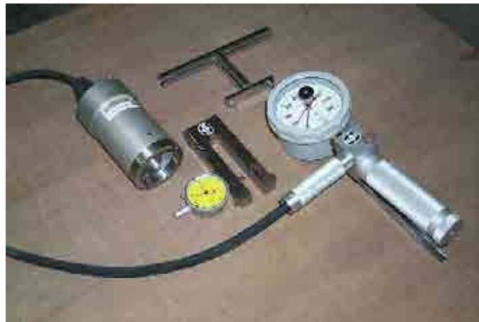
FIG. 87. Break-off test equipment [393].
