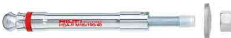
FIG. 14. Example of post-installed undercut anchor for NPP applications (keying effect provides secure hold even in cracked concrete under dynamic loading) [26].
