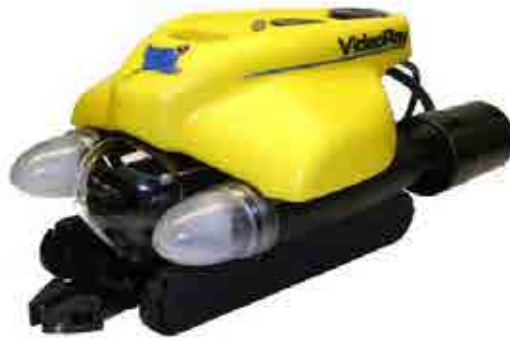
FIG. 59. Typical remotely operated vehicle for nuclear applications (courtesy of Atlantia Marine).
