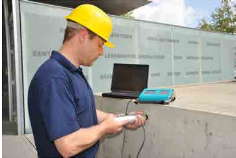
FIG. 80. Rebound hammer test, Digi-Schmidt test hammer (courtesy of Proceq SA).
