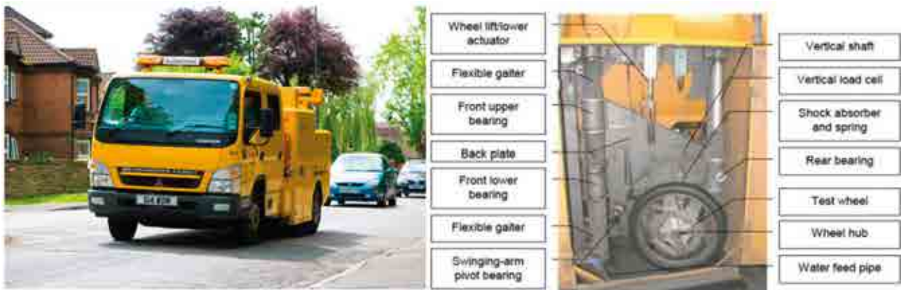
FIG. 191. SCRIM test vehicle (left) (courtesy of W.D.M. Ltd) [708]; test wheel (right) (courtesy of TRL Ltd) [709].
