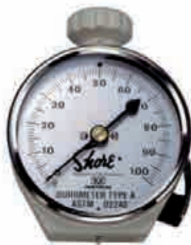
FIG. 127. Durometer for testing elastomeric materials (courtesy of Instron).
