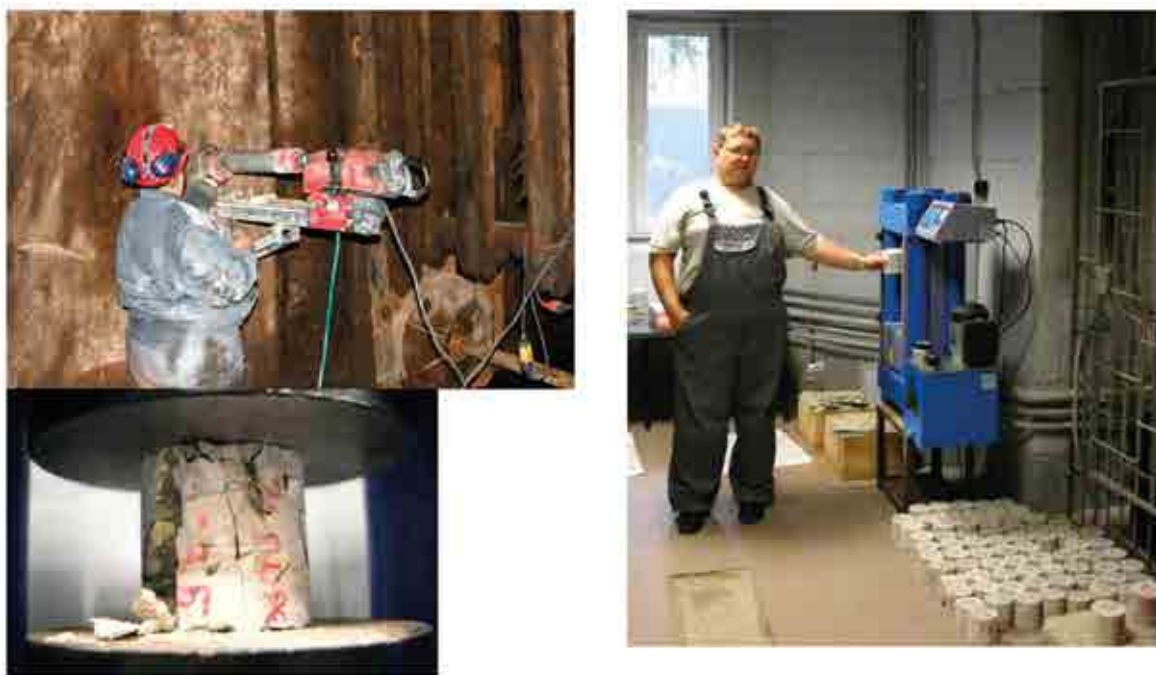
FIG. 86. Obtaining and compression testing a concrete core sample [391].
