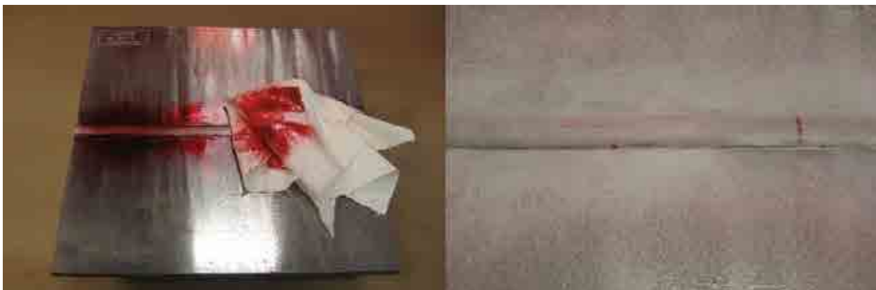
FIG. 114. Flaw revealed by liquid penetrant testing [450].
