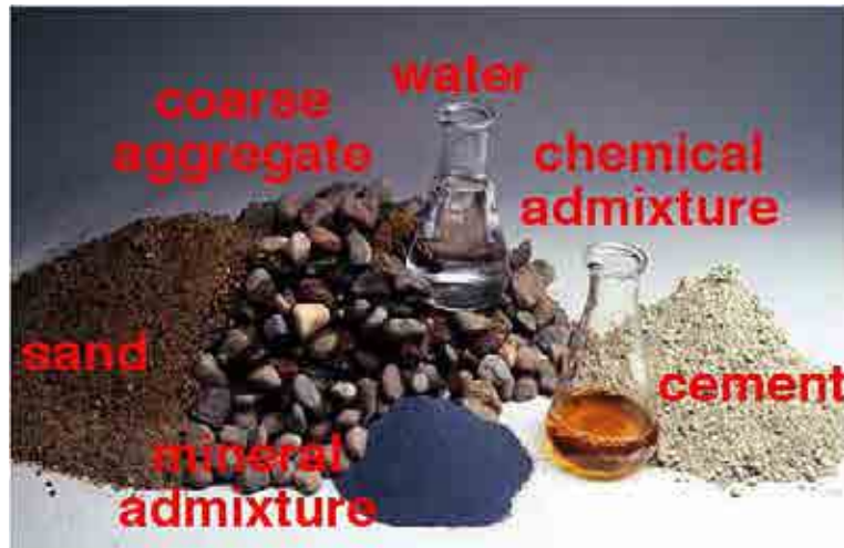
FIG. 17. Concrete constituent components (adapted from Ref. [9]).
