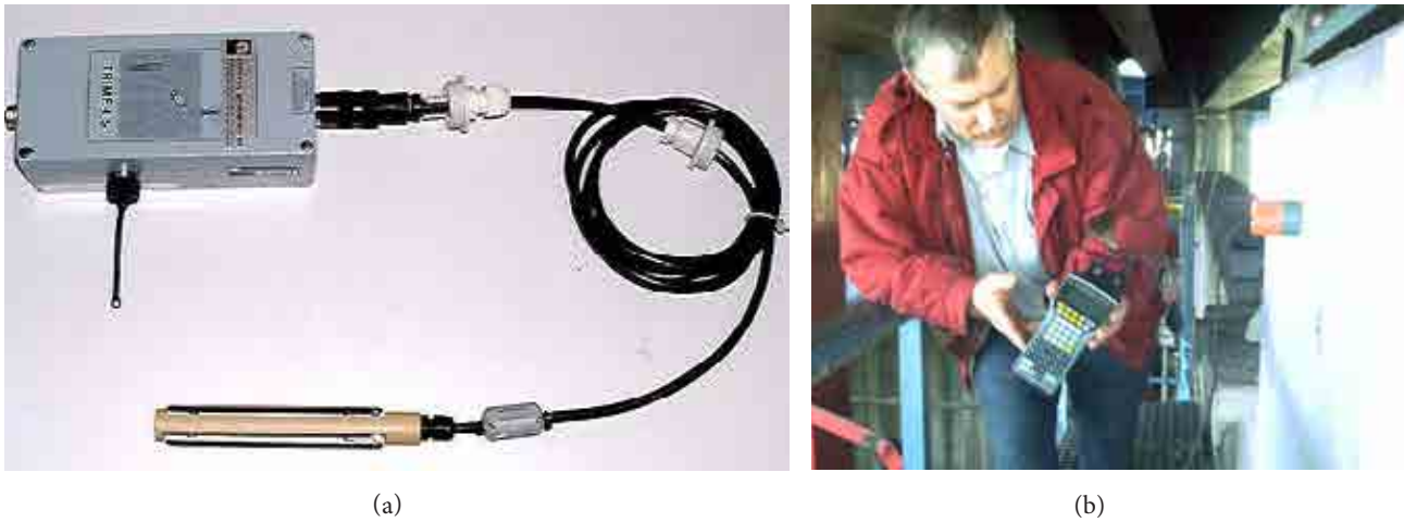
FIG. 134. Application of dielectric measurements to indicate concrete moisture content: (a) TRIME (Time domain Reflectometry with Intelligent MicroElements) sensor for moisture determination (IMKO GmbH); (b) measuring concrete dielectric properties [485].
