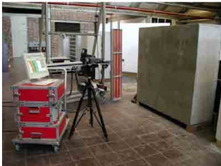
FIG. 75. Impulse thermography test set-up [376].
