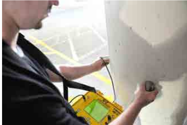
FIG. 61. Example of portable ultrasonic pulse velocity test equipment (courtesy of NDT James Instruments [345]).
