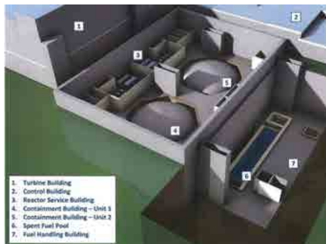
FIG. 187. Reactor service building and fuel handling building for a two unit mPower plant [601].
