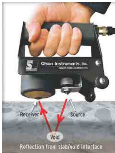
FIG. 65. Impact echo impactor equipment [360].
