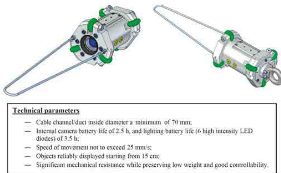
FIG. 112. Prestressing system inspection camera for Temelin NPP; front and rear views (courtesy of Nuclear Research Institute Řež).
