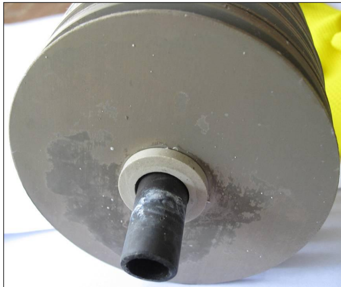
Fig. 2. White debris on the surface of horizontally coupon.
