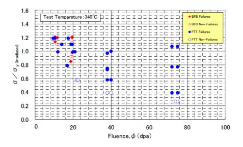
FIG. 2.16. SCC test results as stress/ $\sigma_v$  vs. fluence in dpa (at 340°C) [2.8].
