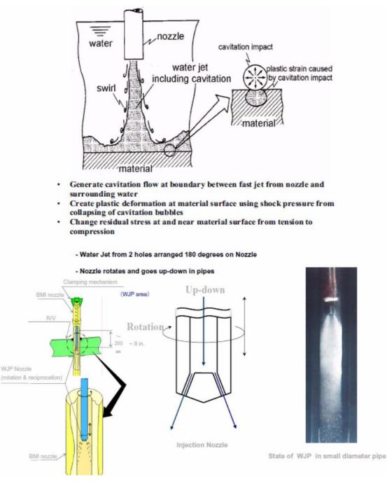
FIG. 6.19. Water jet peening process at the inner surface of a BMI nozzle.
