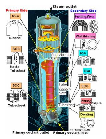
FIG. 3.11. Degradation mechanisms of various steam generator components.
