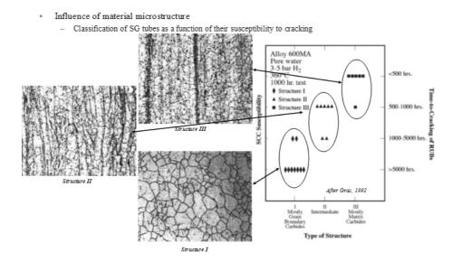
FIG. 2.6. Carbide classification system due to Vaillant.
