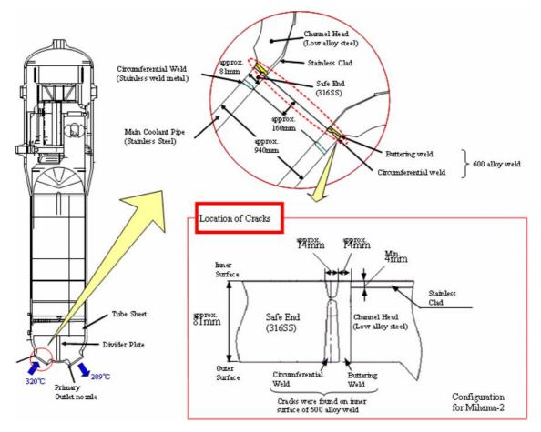
FIG. 3.12. Location of the primary inlet nozzles with indication.
