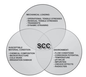
FIG. 2.1. Critical factors for stress corrosion cracking.
