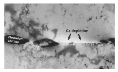
FIG. 2.3. Transmission electron microscope (TEM) image showing chromium carbide precipitates along a grain boundary and the zone of Cr-depletion [2.1].
