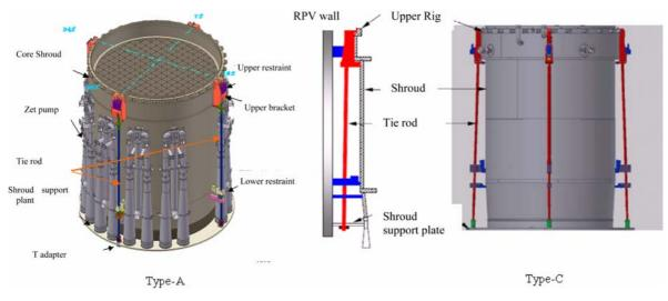
FIG. 6.10. Core shroud tie rods.
