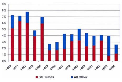
FIG. 3.5. Corrosion related capacity factor losses due to corrosion in PWRs [3.1].
