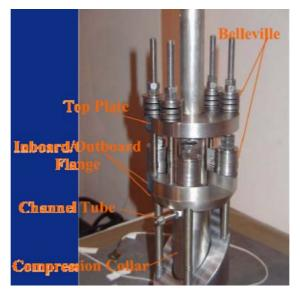
FIG. 6.24. MNSA device on a test location.
