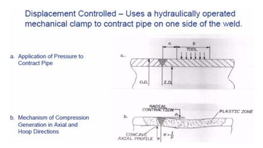
FIG. 6.17. Basic concept of MSIP: a clamp is applied on one side of a pipe weld to plastically deform the weld and in the process generates compressive stresses in both the axial and hoop directions.
