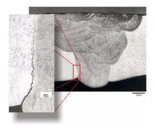
FIG. 3.2. IGSCC initiated at a notch root as a result of moderate cold work and a crevice condition.
