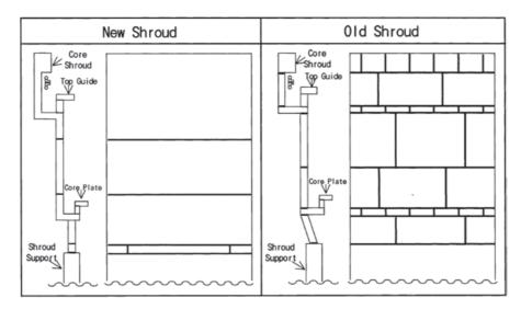
FIG. 6.2. Comparison between the old and new core shroud structures.
