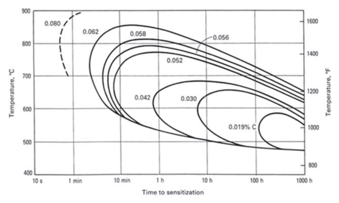
FIG. 2.2. Time-temperature-transformation (TTT) diagram for austenitic stainless steel showing the combinations of time, temperature and carbon content that lead to sensitization.
