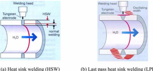
(b) Last pass heat sink welding (LPHSW)
