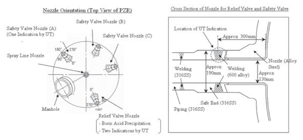
FIG. 3.10. Location of the nozzle with indication at Tsuruga Unit 2 [3.25].
