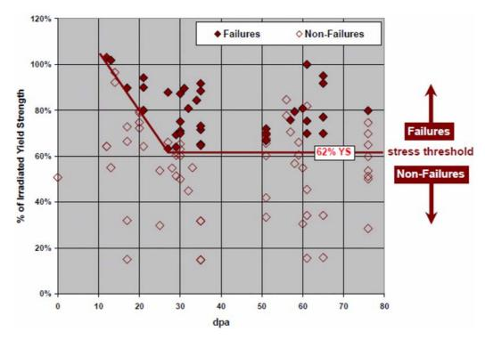
FIG. 2.17. SCC test results as stress/ $\sigma_v$  vs.fluence in dpa (at 340°C) [2.15].
