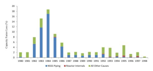
FIG. 3.1. Corrosion related capacity factor losses due to corrosion in BWRs [3.1].
