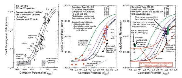
FIG. 6.6. Relationship between crack propagation rate and corrosion potential for sensitized Type 304 stainless steel in 288°C water under constant load and conductivity between 0.1 to 0.3  $\mu$ S/cm. The curves are the predicted relationships based on the slip-oxidation mechanism of crack propagation [6.14].
