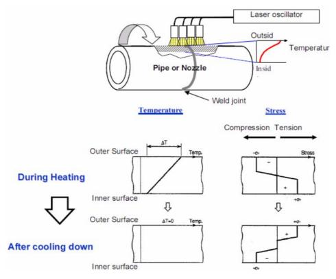
FIG. 6.20. Principle of L-SIP.
