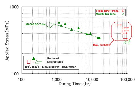
FIG. 2.14. Results of PWSCC tests on alloy 690 base metal and Alloy 600 base metal showing no cracking detected in alloy 690 after test times up to ~75 000 hours.
