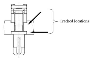
FIG. 3.13. Typical cracked location.
