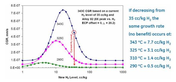
FIG. 6.23. Modelled crack growth rates for Inconel 82 showing the effect of hydrogen at different temperatures.
