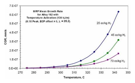
FIG. 2.9. Effect of temperature on PWSCC crack growth rate for alloy 182 [2.11].
