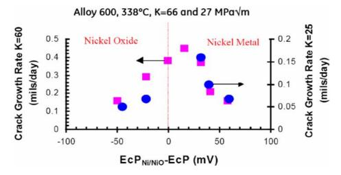
FIG. 2.8. Crack growth rate for alloy 600 in simulated PWR environment at 338°C [2.11].
