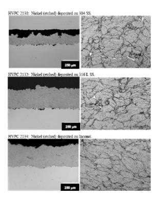
FIG. 6.13. Typical appearance of cold spray coatings in cross-section and on the surface. Both nickel and stainless steels coatings have been applied to type 304 SS, type 316 SS and alloy 600 substrates.
