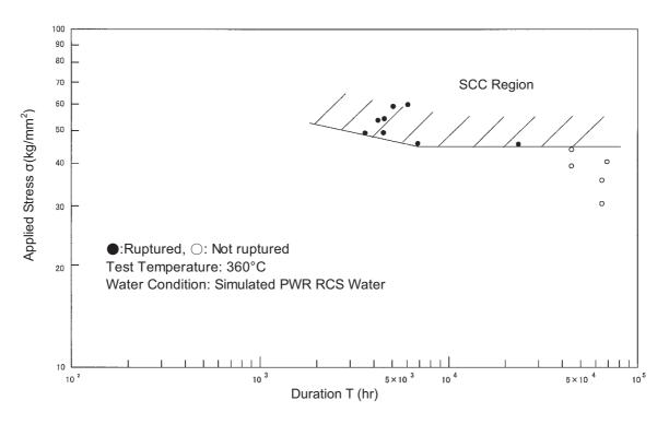
FIG. 2.12. Results of constant load PWSCC tests for alloy 600 base metal.
