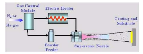
FIG. 6.12. Sketch of the cold spray corrosion resistant coating process.
