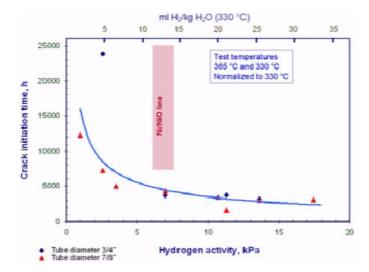
FIG. 2.10. The effect of hydrogen on initiation time. The data includes measurements at different temperatures normalized to the hydrogen partial pressure at  $330^{\circ}C$  [2.12].
