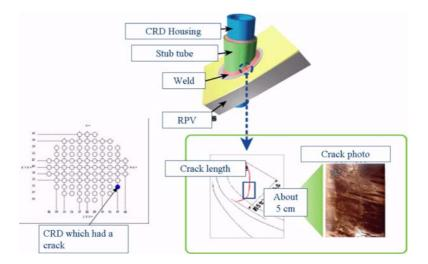
FIG. 3.3. CRD stub tube leak at Hamaoka NPP.
