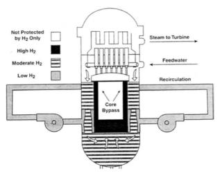
FIG. 6.7. Hydrogen water chemistry in reactor internals [6.15].
