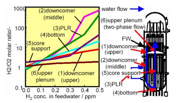
FIG. 6.8. ECP distribution for BWR internals.
