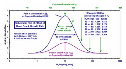
FIG. 6.22. Modelled crack growth rate for alloy 600 and alloy 182 for different hydrogen concentrations at 325°C.
