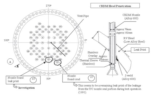
FIG. 3.8. Location of CRDM head penetrations with leakage [3.24].
