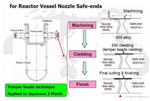
FIG. 6.14. 3-layer temper bead weld cladding technology.
