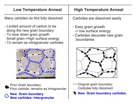
FIG. 2.5. Schematic of the carbide precipitation process.
