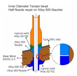
FIG. 6.25. Schematic of a crevice formed by the half nozzle repair.
