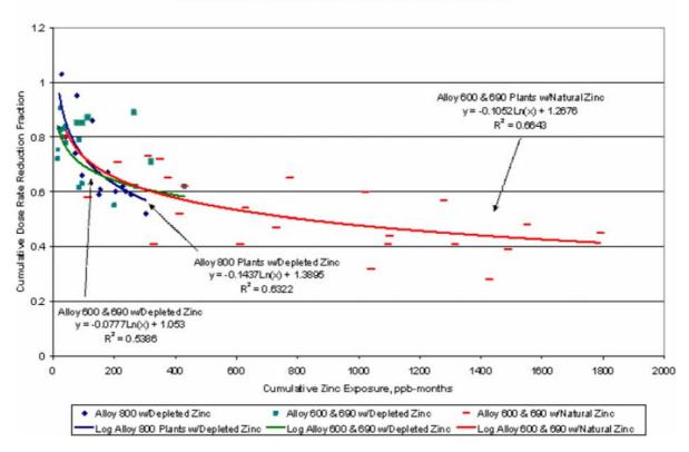
FIG. 6.21. Trends observed at US PWRs adding zinc, dose rate reduction vs. cumulative zinc exposure (ppb-mo). A significant fraction of the decrease in dose due to less corrosion product release is observed after ~300 ppb-mo of zinc exposure. Similar effects are anticipated for reduction in PWSCC [6.39].
