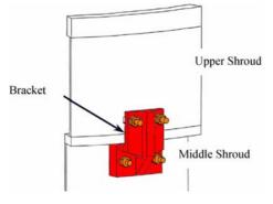
FIG. 6.11. Brackets repair technology.
