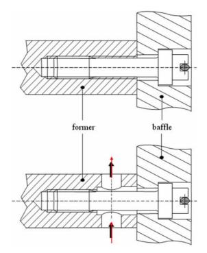
FIG. 6.15. Holes for water flow through formers to cool baffle bolts.
