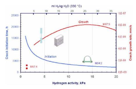
FIG. 2.11. Comparison of the effect of hydrogen on initiation and propagation of PWSCC in alloy 600 MA [2.12].
