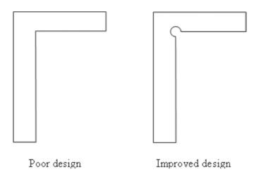
FIG. 6.3. Sketch of the tie rod upper support designs.
