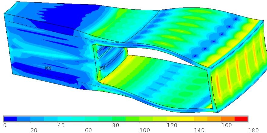
FIG.5. Von Mises stress contour plot for 316L shroud with flat beam profile and 60rpm rotation rate.
