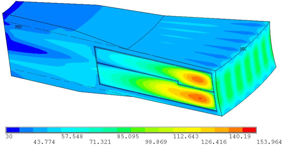
FIG. 3. Temperature profile plot just after the pulse at 16 s for a flat beam profile and 60 rpm.
