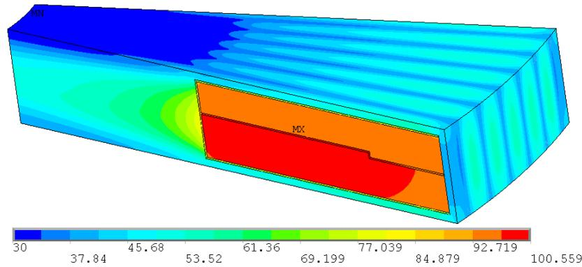
FIG. 6. Temperature profile plot for decay heat removal with 1mm tantalum cladding.
