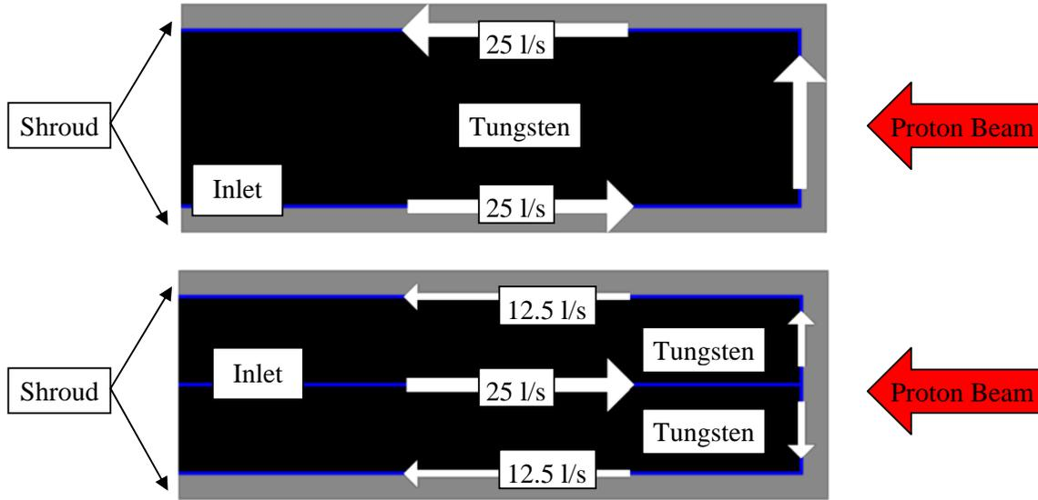
FIG. 1. Cross-section views for coolant flow designs for top, bottom, and outer face only scheme (top) and with additional central cooling channel (bottom).
