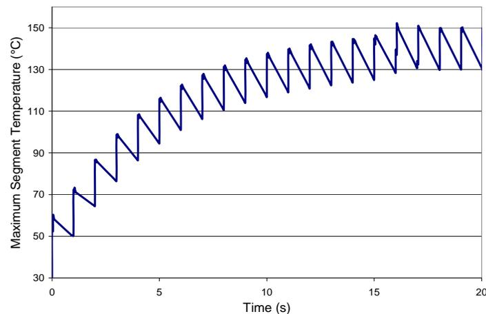
*FIG. 2. Maximum segment temperature vs. time for a flat beam profile and 60 rpm.*
