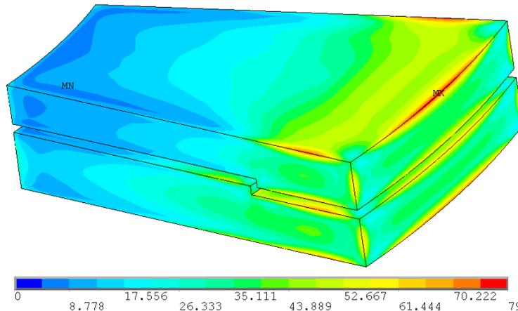
FIG. 4. 1<sup>st</sup> principle stress contour plot for tungsten with a flat beam profile rotated at 60rpm.
