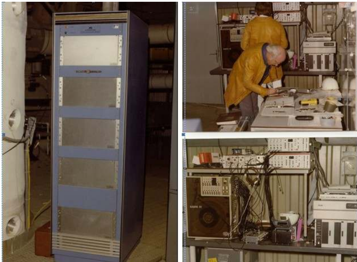
FIG. 2 256 Channel BatScan System installed at SCTI (USA); 8 Channel BatScan at Hengelo (NL)
