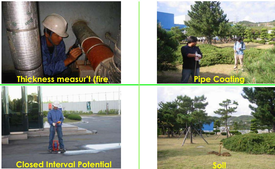
FIG. 4. Buried commodity inspection in the field
