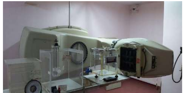
Figure 21. Cobalt-60 machine and different phantoms used in the calibration of radiotherapy dosimeters
