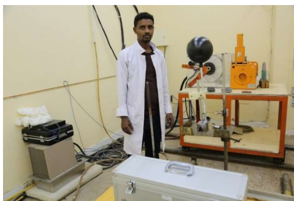
Figure 15. Set up preparation for ionization chamber X-ray and Gamma irradiator
