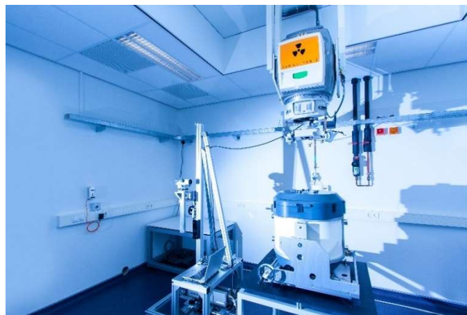
Figure 11. VSL water calorimeter in the ^{60}\text{Co} facility
