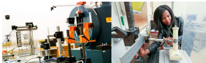
Figure 23. From left to right: The Co-60 irradiator with a water phantom and some setup equipment for air kerma measurements, A Scientist setting up for a calibration of a contamination monitor.
