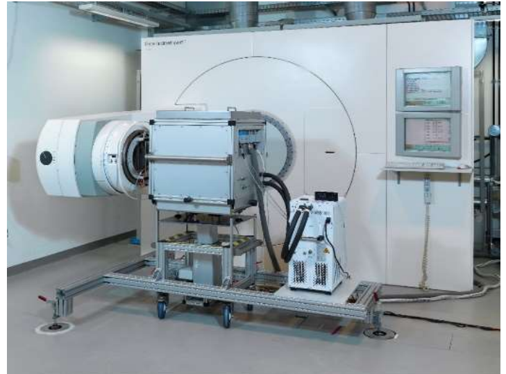
Figure 9. PTB's water calorimeter (with the cooling system) in front of the clinical linac
