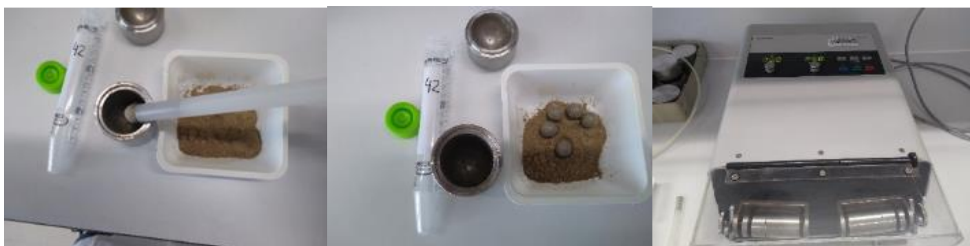
Figure 1. Ball-milling soil samples for MIRS analysis.
