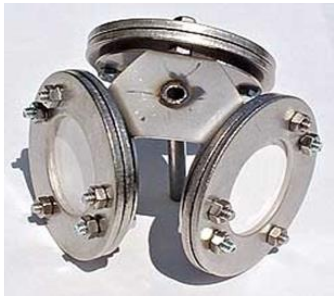
Passive samplers for evaluating pesticide isotope signatures (Photo Credit: G. Imfeld, France)
