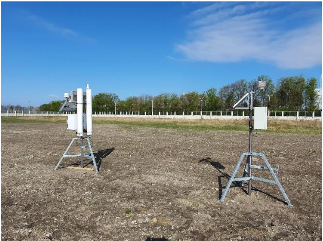
Figure 1. Traditional (left) and novel (right) Cosmic Ray Neutron Sensors at the SWMCN Laboratory research site in Seibersdorf, Austria.
