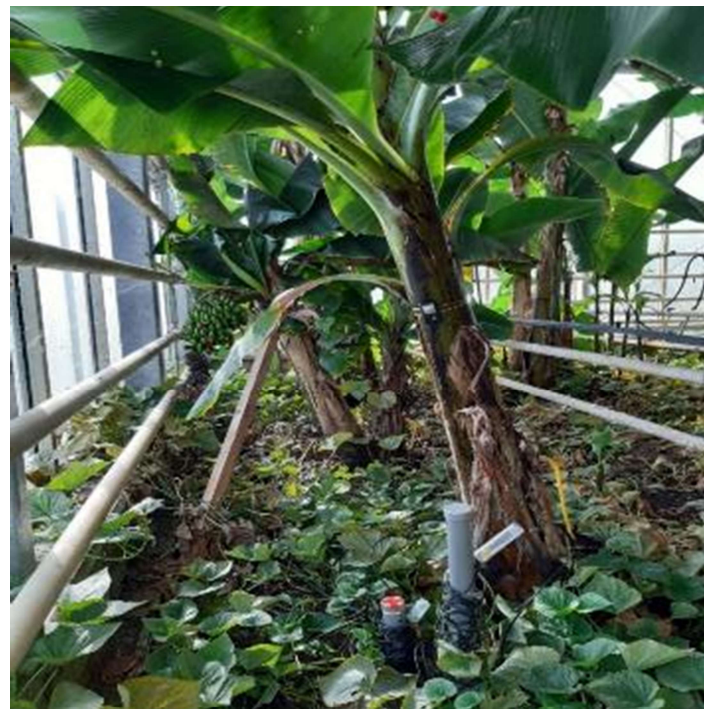
Figure 1. Experimental set-up with TDR sensors inserted in the soil at different depths and RH and air temperature sensor attached to the plant.
