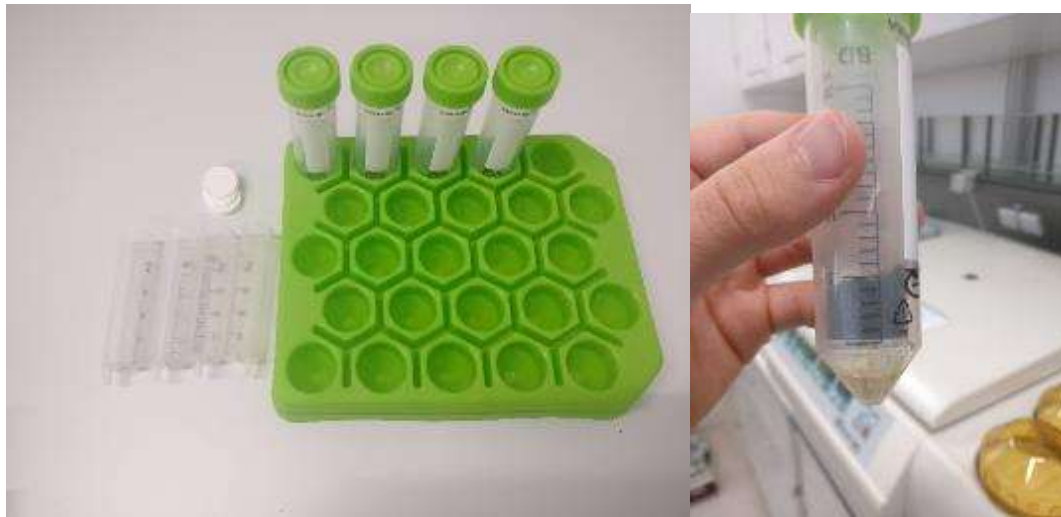
Figure 2. Soil water extraction tubes for centrifugation. The only materials needed are 50 mL centrifugation tubes, 20 or 30 mL syringes and a filter. The extracted water is collected in the space under the syringe and can be used for isotopic analysis of water.
