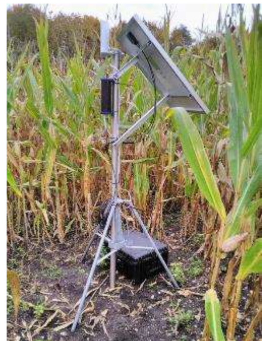
Figure 1. Gamma Soil Moisture Sensors (GSMS), model GSMS100 in Seibersdorf, Austria
