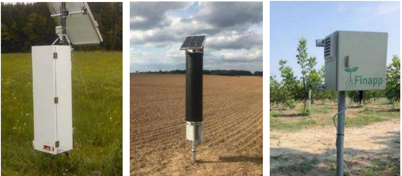
Figure 2. Alternative to proportional gas tube CRNS probes from Lab-C (left), Stix-neutronica (centre), Finapp (right)
