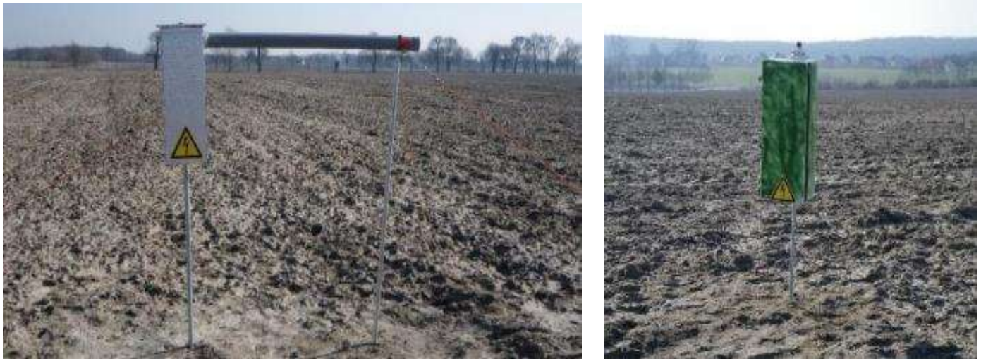
Figure 1. CRNS detectors (left) a commercial CRS1000 from Hydroinnva LCC; (right) a home-made assembly based on Canberra proportional gas tube.
