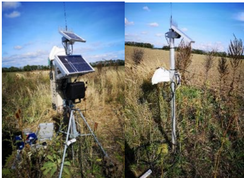
Figure 1. Cosmic Ray Neutron Sensor (left); Drill & Drop capacitance probe (right) installed in Rutzendorf Austria
