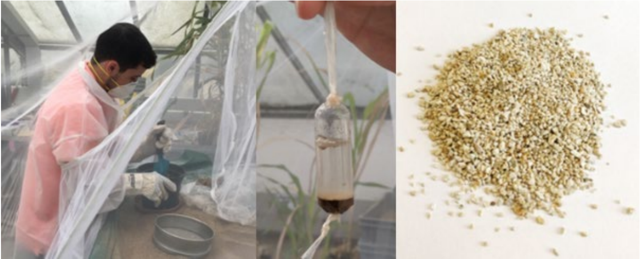
From left to right: (1) Preparation of soils; (2) Dialysis bags with soil samples for RIP analysis; (3) Zeolite minerals
