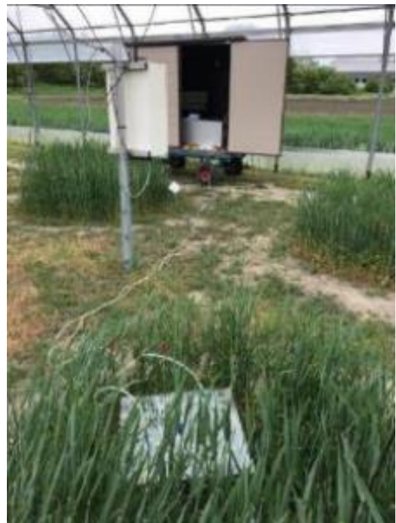
\text{N}_2\text{O} measurement on a lysimeter, using off-axis Integrated Cavity Output Spectroscopy (OA-ICOS).
