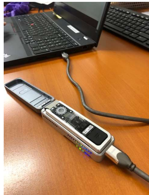
FIG. 2. The Oxford Nanopore plc MinION DNA Sequencer connected to a laptop through USB and loaded with a Flongle, the sequencing consumable containing the membrane with pores. Flongle costs around 100 Dollars and provides sequencing capacity up to 1.8 Gb.
