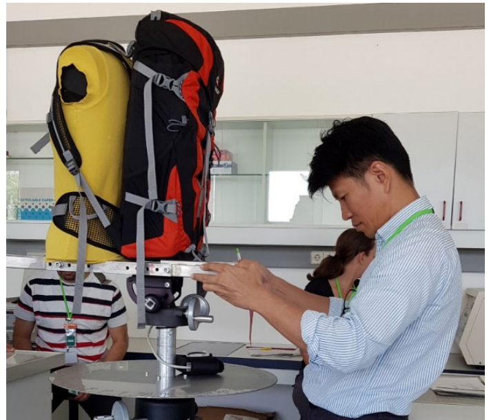
Figure 8: Testing of backpack spectrometer within the training
